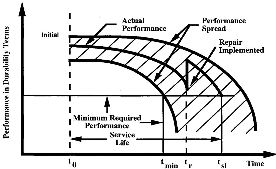
Fig. 2.24 Relationship between concrete performance and service life.
