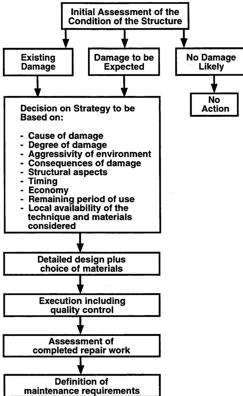
Fig. 3.4 Steps to be taken in a repair process. Source: Technical Committee 124- SRC, "Draft Recommendation for Repair Strategies for Concrete Structures Damaged by Reinforcement Corrosion," pp. 415-436 in *Materials and Structures* 27(171), International Union of Testing and Research Laboratories for Materials and Structures (RILEM), Cachan, France; adapted with permission from RILEM.
