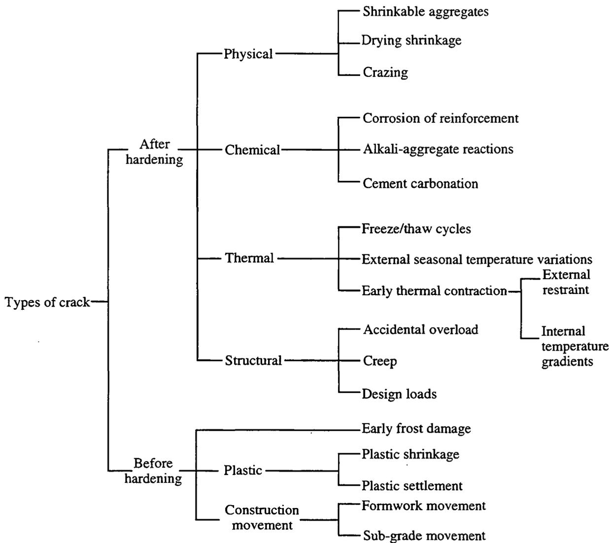
Fig. 2.9 Relationship between primary causes and types of cracks that can occur in concrete. Source: Comité Euro-International du Béton (CEB), *Durable Concrete Structures—Design Guide*, published by Thomas Telford Services Ltd., London, England, 1989; reprinted with permission from CEB and Thomas Telford Services Ltd.
