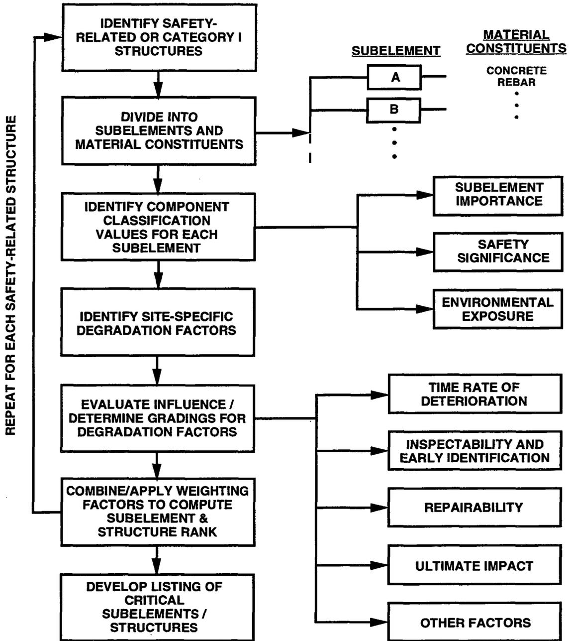
Fig. 4.1. Structural aging assessment methodology flow diagram.
