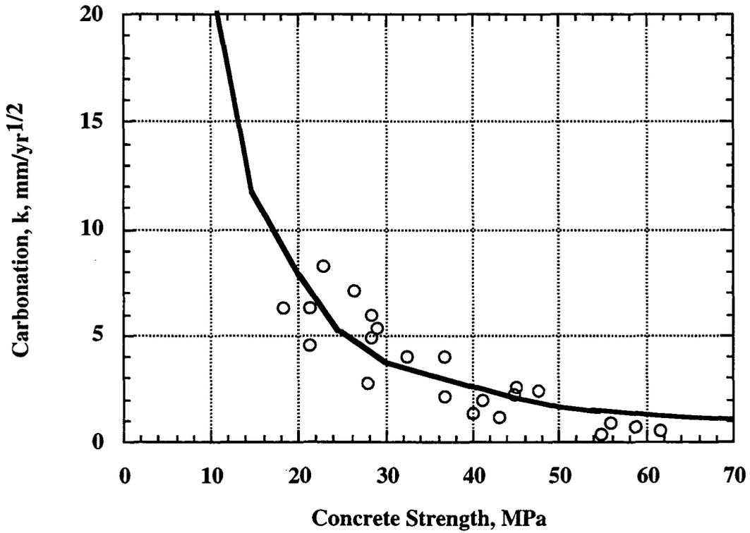
Fig. 2.14 Carbonation data for exterior sheltered concrete.<sup>123</sup>
