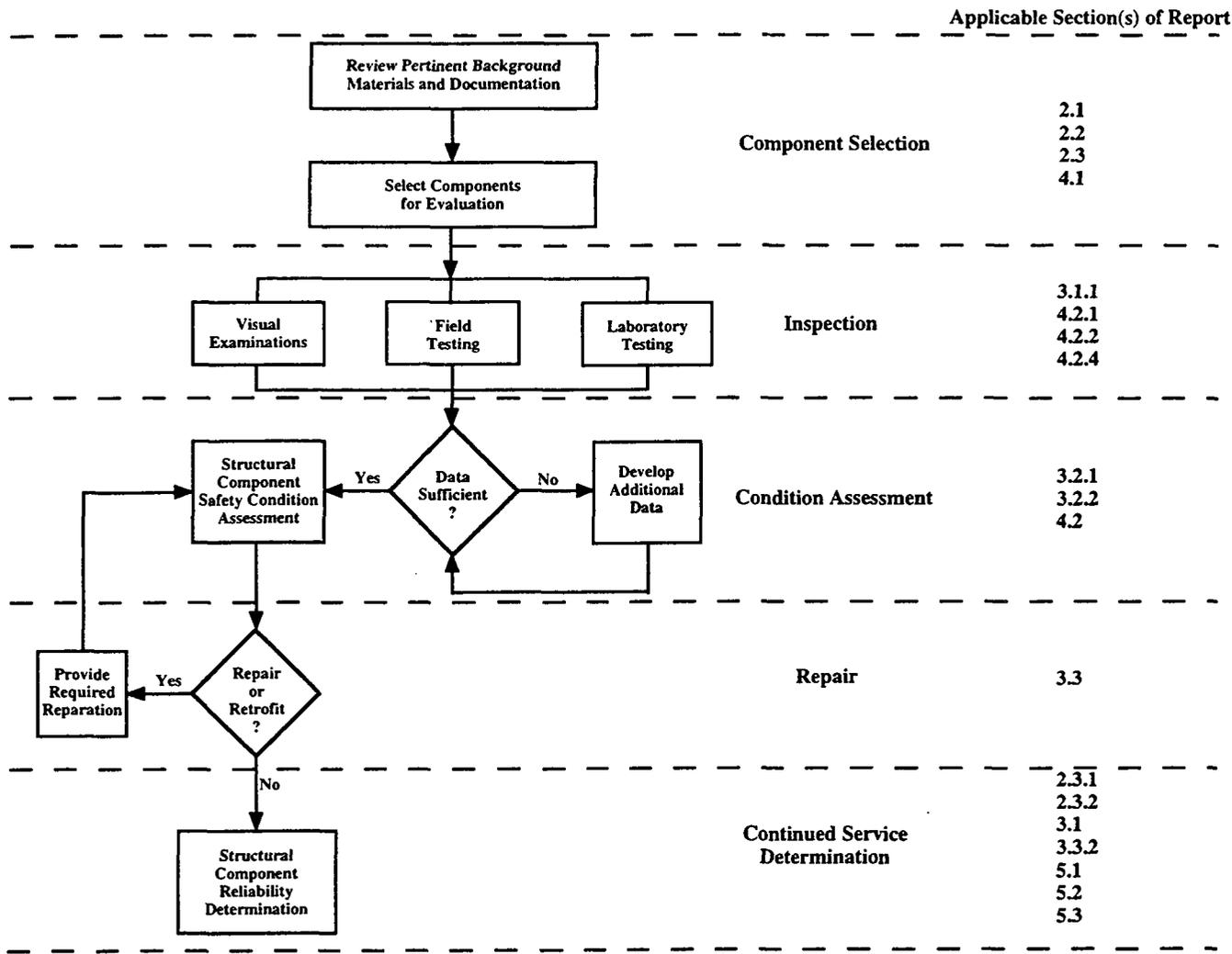
Fig. 1.6 Evaluation methodology for NPP reinforced concrete structures.
