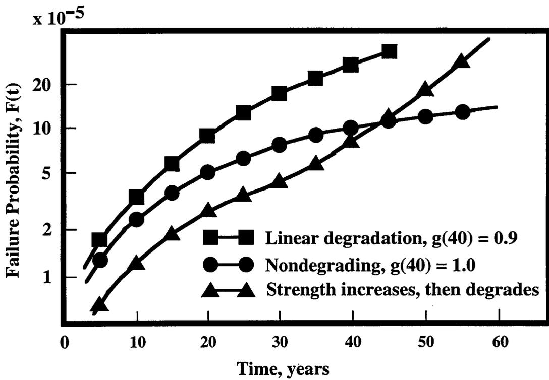
Fig. 5.3 Failure probability of a one-way slab.
