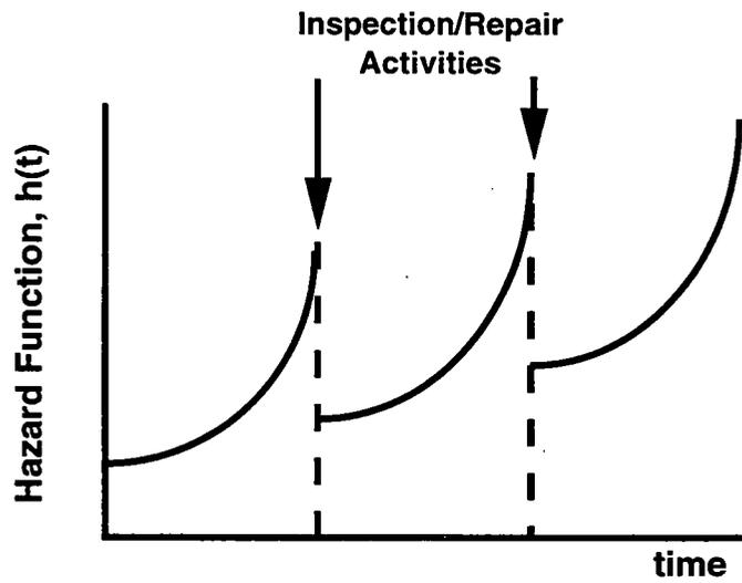
Fig. 5.9 Role of inspection/repair in controlling failure rate.
