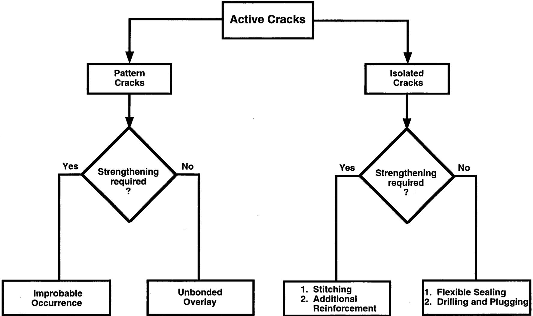
Fig. 3.6 Selection of repair technique for active cracks. Source: *Evaluation and Repair of Concrete Structures*, EM 1110-2-2003, U.S. Army Corps of Engineers, Washington, D.C., 1986.
