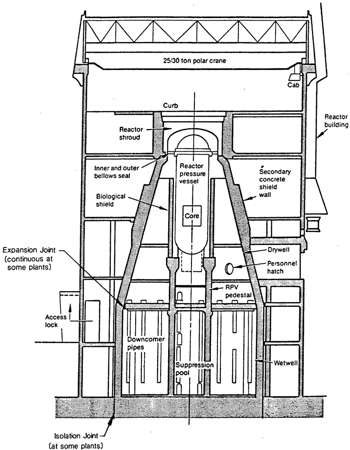
Fig. 2.2 BWR Mark II type reinforced concrete containment. Source: Copyright © 1994. Electric Power Research Institute. EPRI TR-103840-R1. *BWR Containments License Renewal Industry Report: Revision 1*. Reprinted with Permission.
