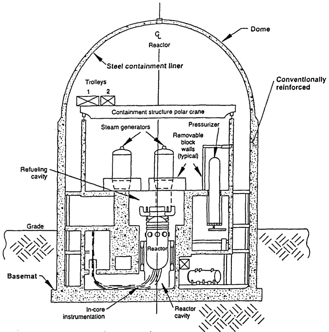
Fig. 2.4 PWR subatmospheric type reinforced concrete containment.
