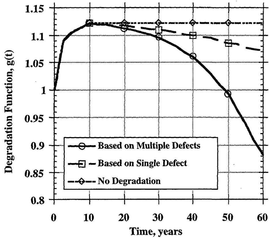
Fig. 5.5 Mean degradation function of wall in shear without repair.
