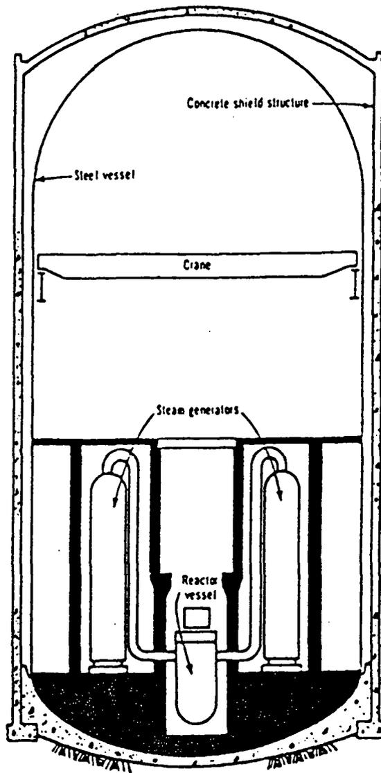
Fig. 2.7 PWR free-standing steel containment with elliptical bottom. Source: Copyright © 1994. Electric Power Research Institute. EPRI TR-103835. *PWR Containment Structures License Renewal Industry Report: Revision 1*. Reprinted with Permission.
