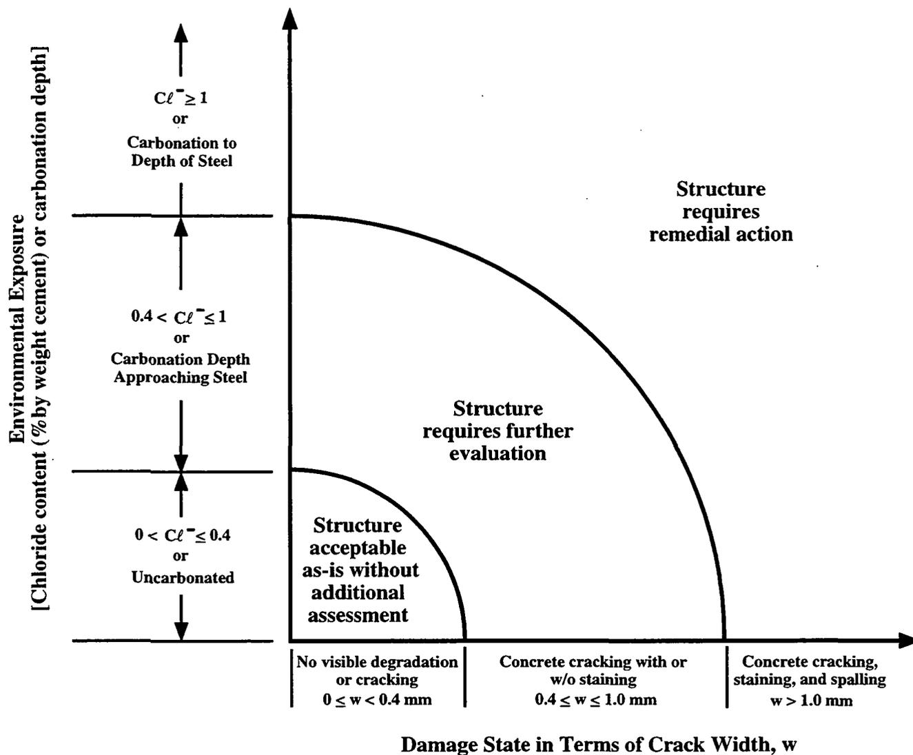
Fig. 4.2 Damage state chart relating environmental exposure, crack width, and necessity for additional evaluation or repair.
