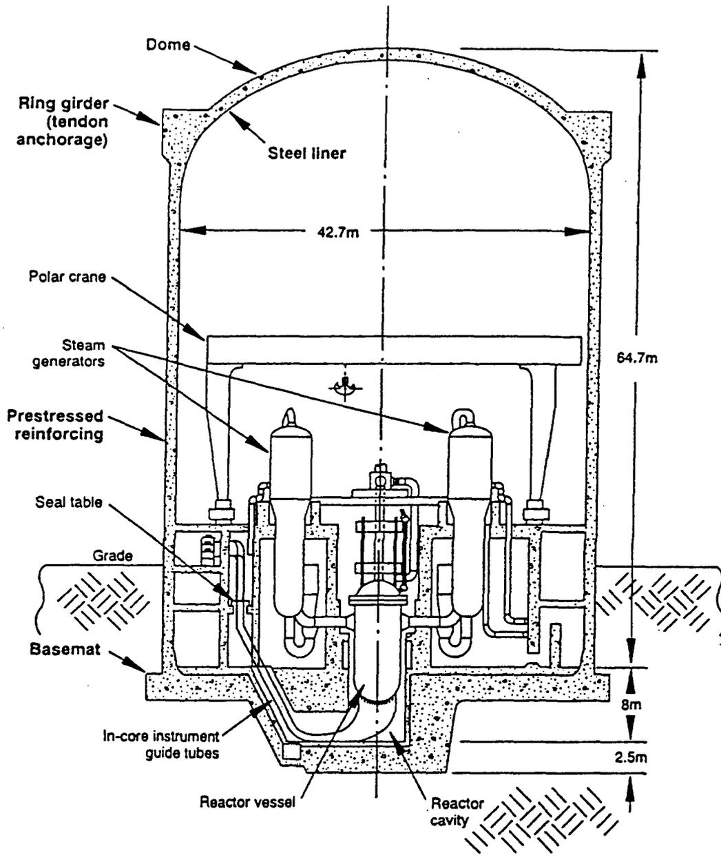
Fig. 2.6 PWR large dry prestressed concrete containment.
