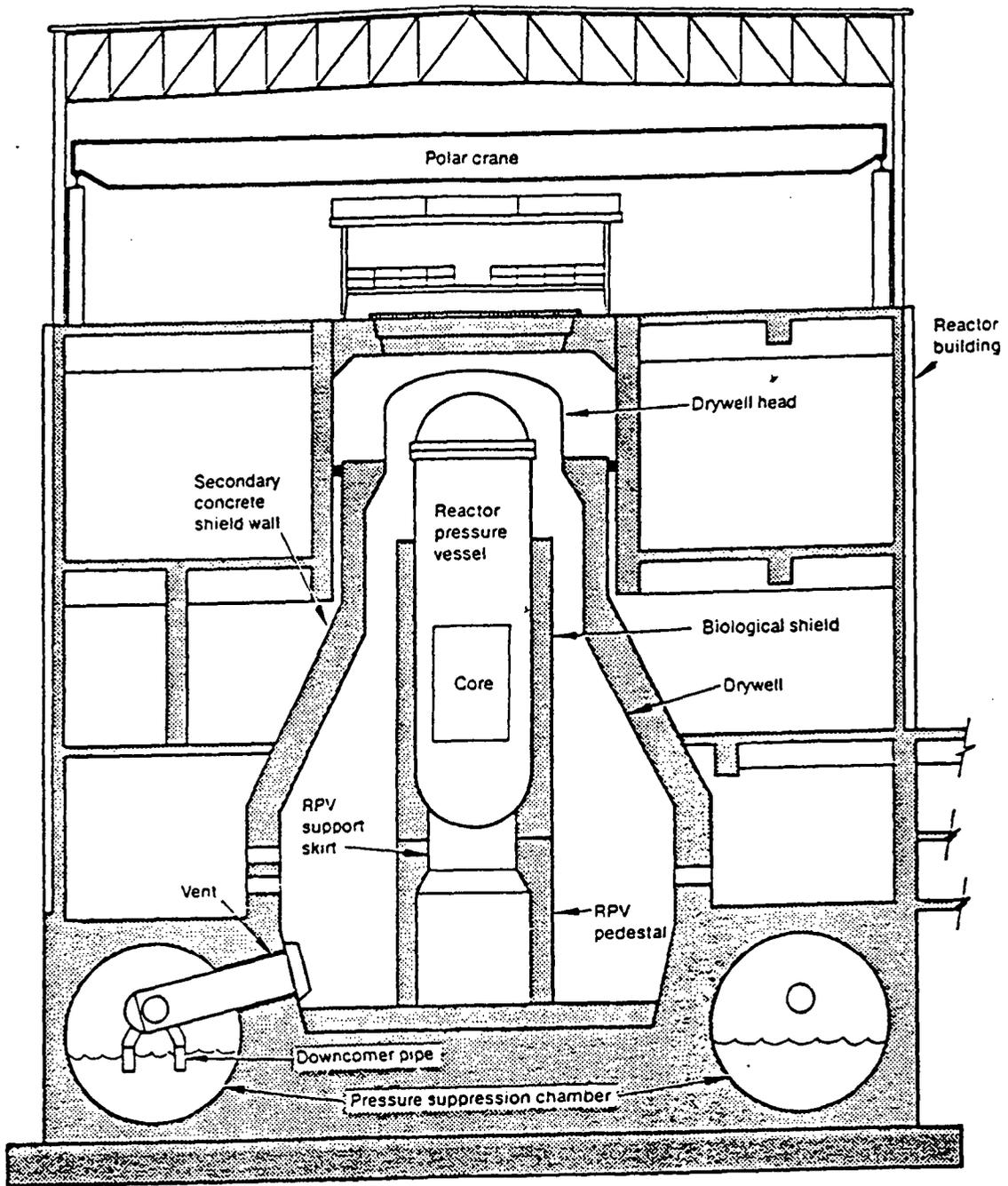
Fig. 2.1 BWR Mark I type reinforced concrete containment. Source: Copyright © 1994. Electric Power Research Institute. EPRI TR-103840-R1. *BWR Containments License Renewal Industry Report; Revision 1*. Reprinted with Permission.
