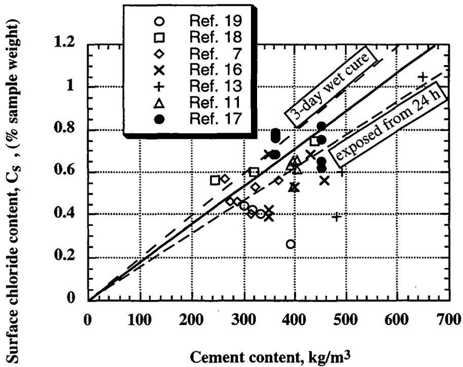
Fig. 2.15 Proposed curves for surface chloride content versus cement content for different curing conditions (Refs. refer to Ref. 123).
