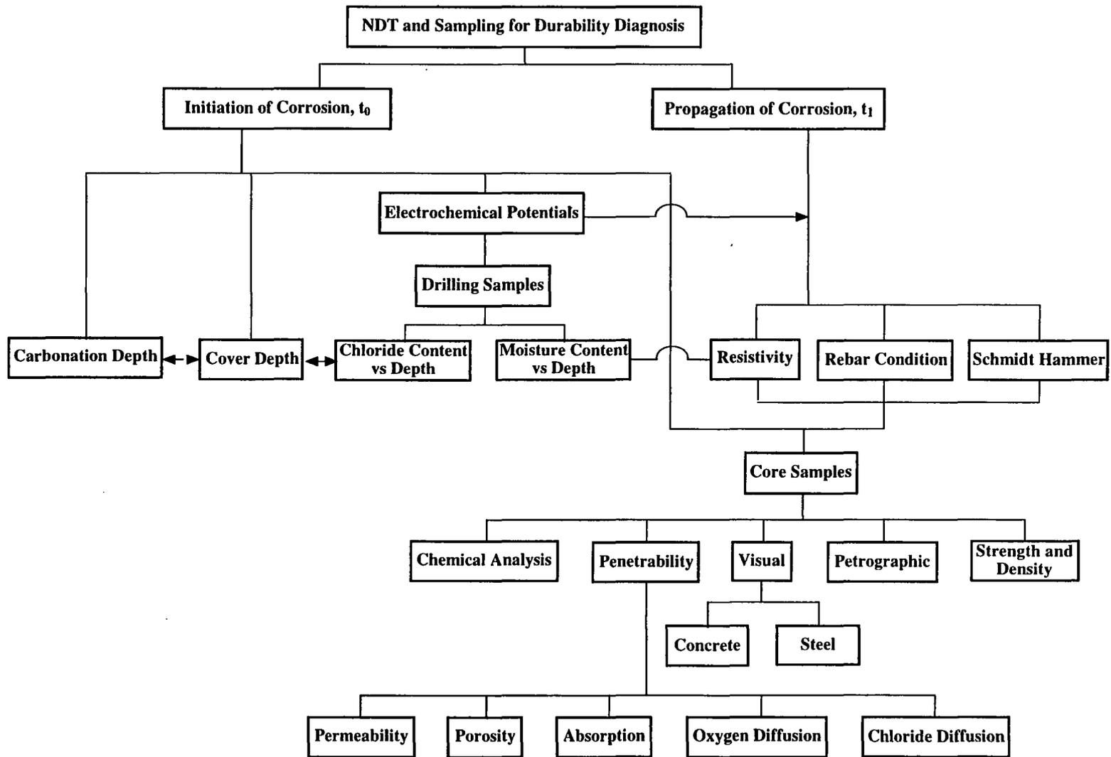
Fig. 3.1 Techniques for assessing deterioration. Source: R. D. Browne, "Durability of Reinforced Concrete Structures," *Pacific Concrete Conference*, Proceedings Vol. 3, Auckland, New Zealand, New Zealand Concrete Society, November 1988; reprinted with permission from author.
