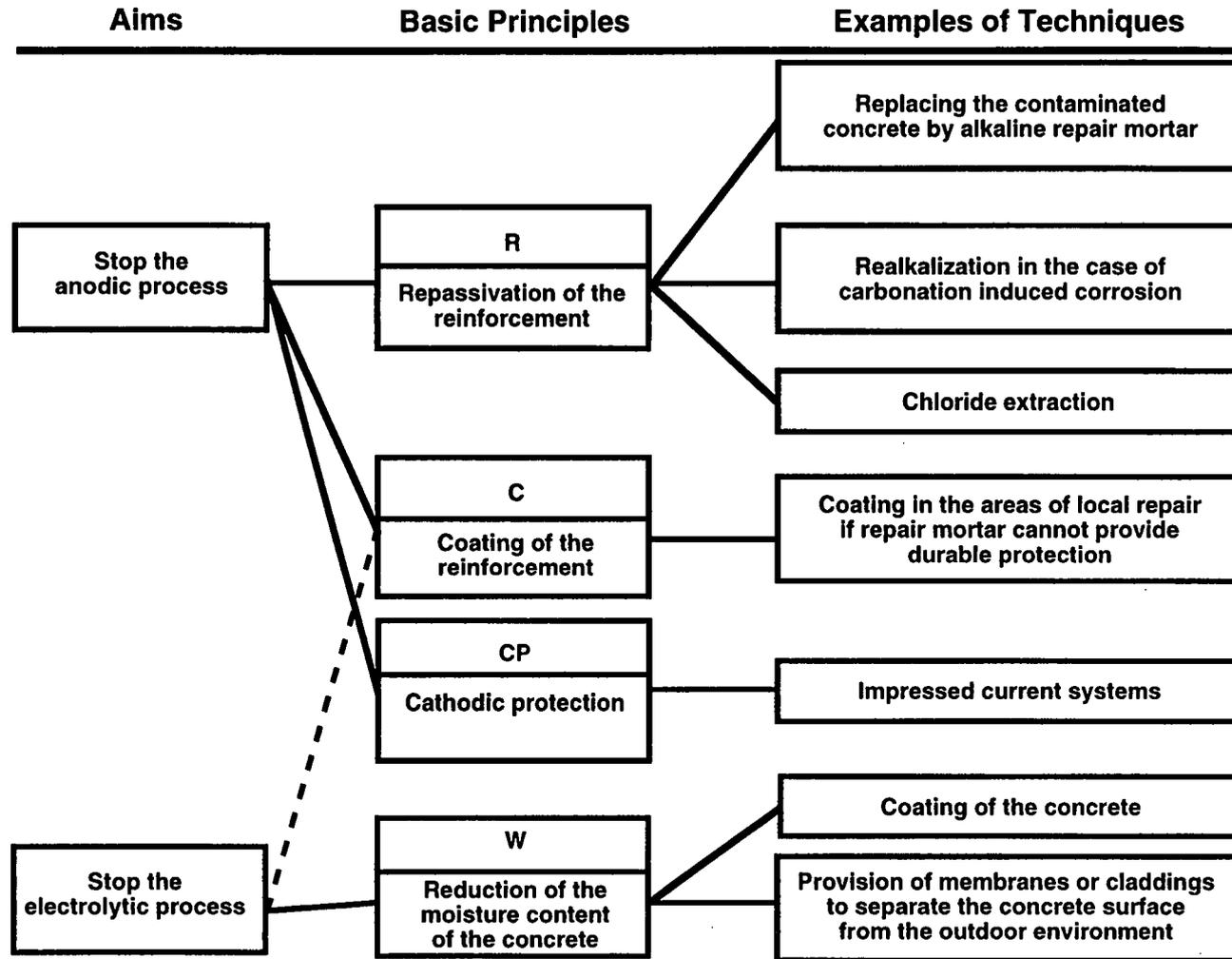
Fig. 3.7 Principles of repair to stop corrosion.
