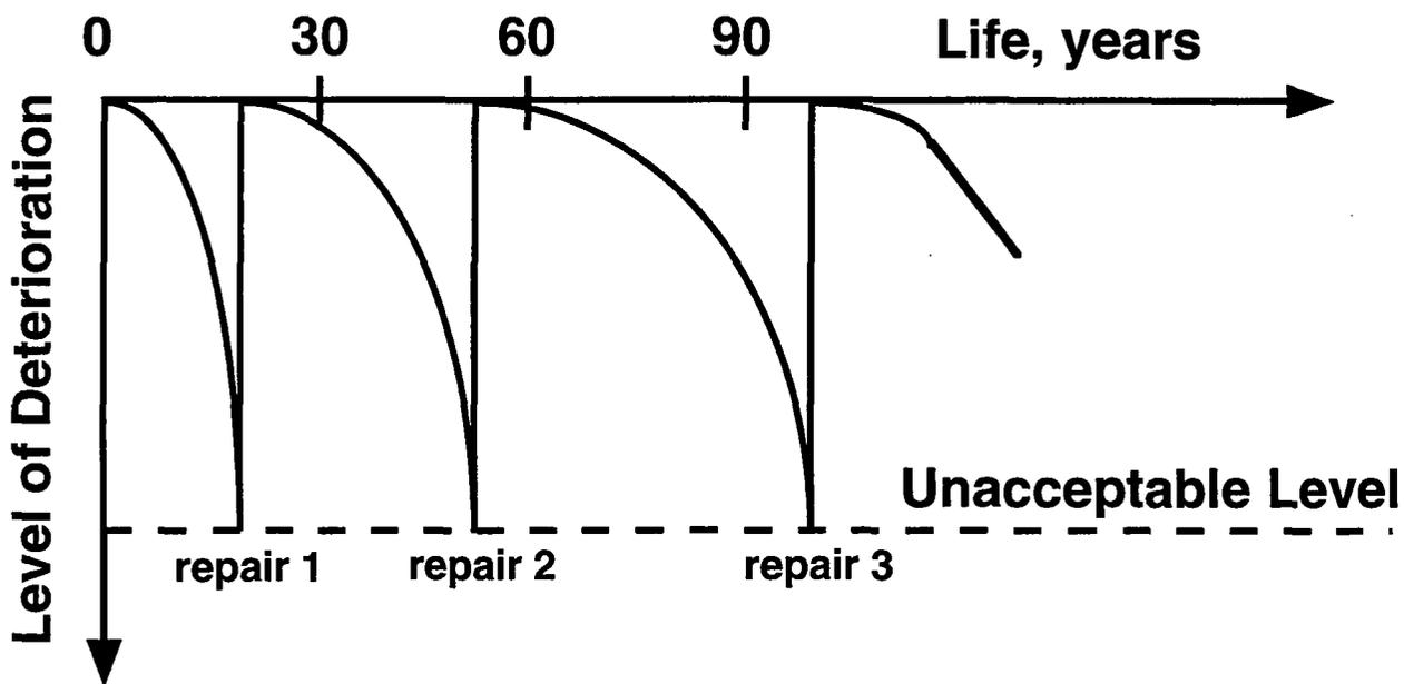
Fig. 3.3 Effect of multiple repairs over the life of a structure.
