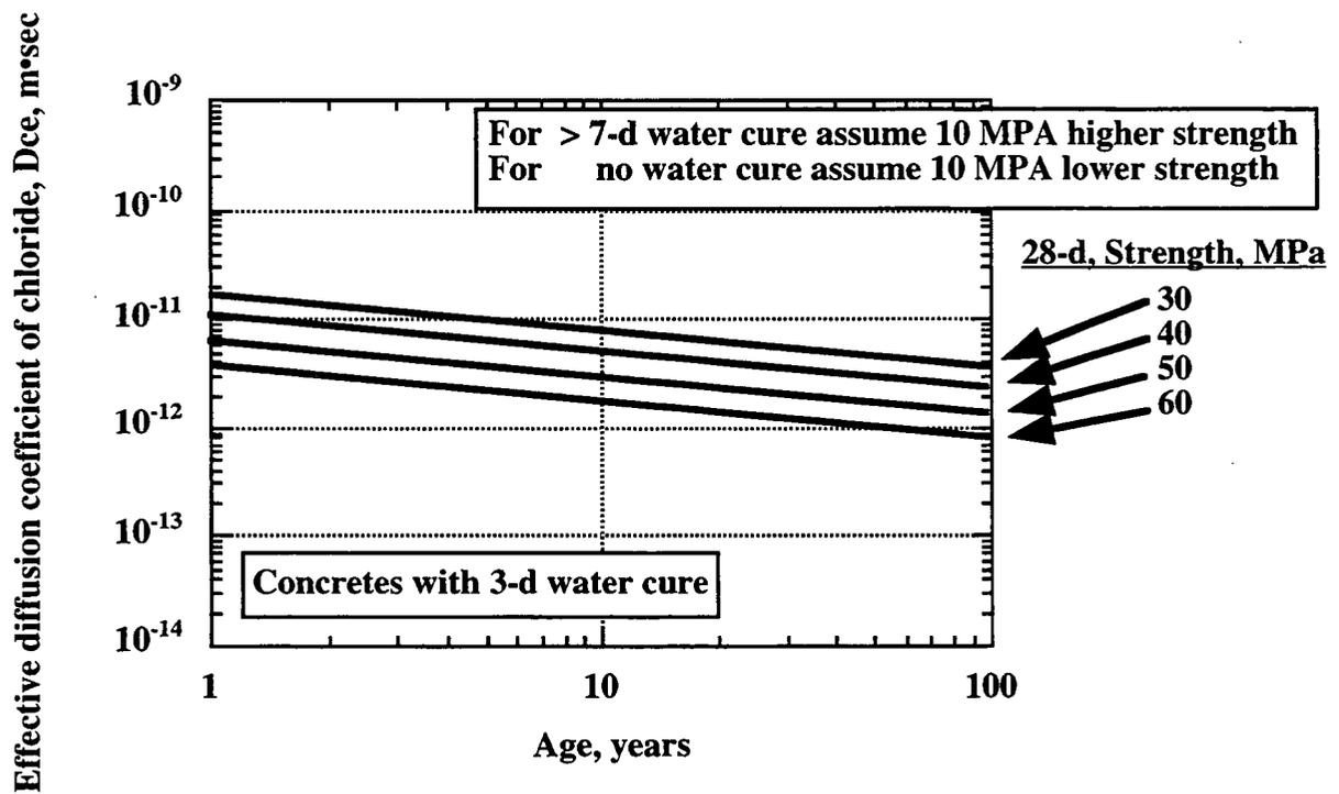
Fig. 2.16 Effective diffusion coefficient of chloride versus time for ordinary portland cement concretes.<sup>123</sup>
