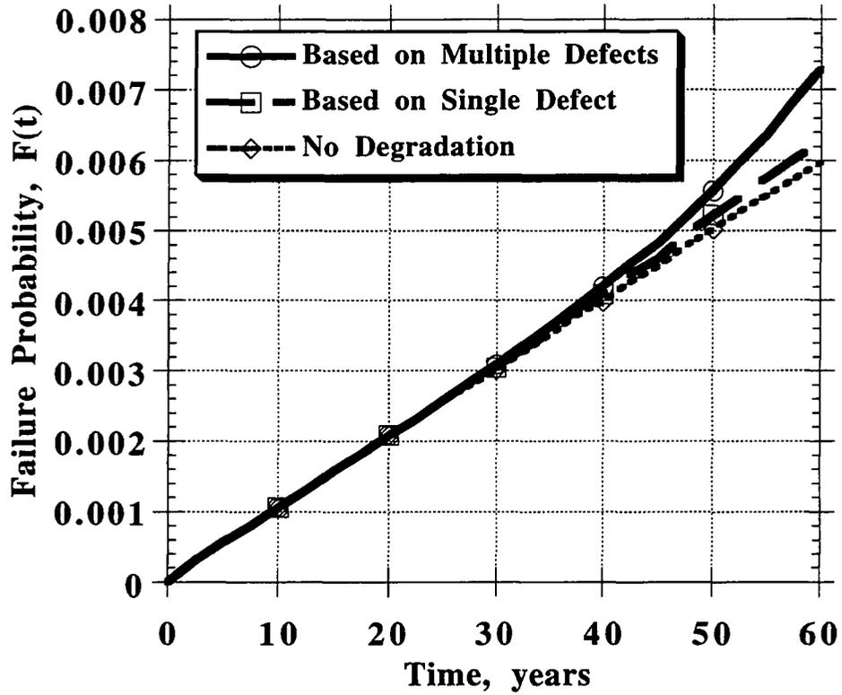
Fig. 5.6 Failure probability of wall in shear without repair.
