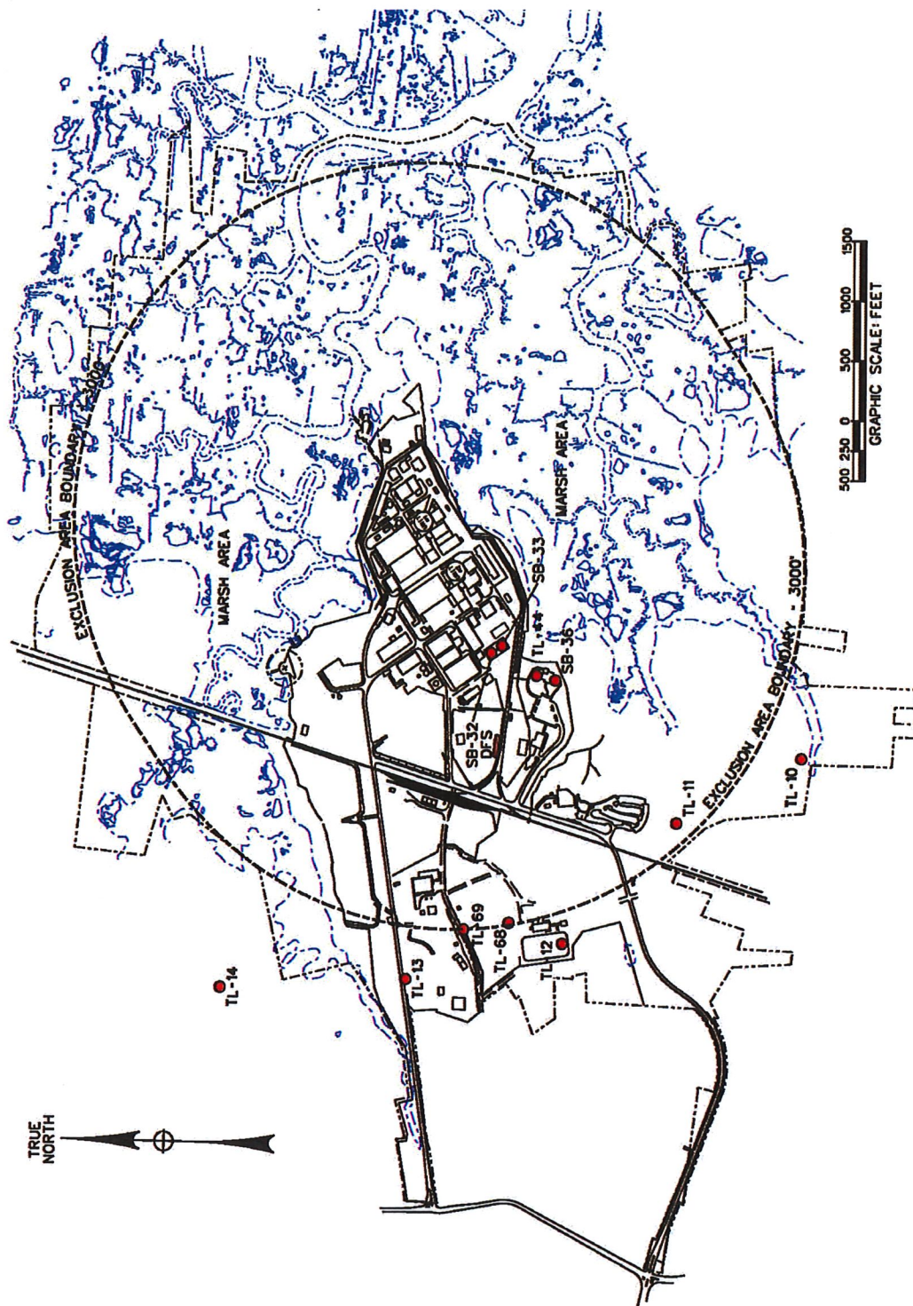
Figure 4.0.1 Dry Fuel Storage TLD Environmental Monitoring Locations
