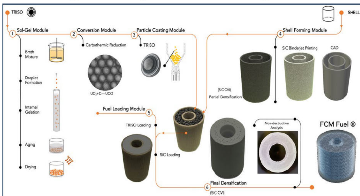
Figure 3.1. Flow Diagram of FCM Fuel Manufacturing Process
