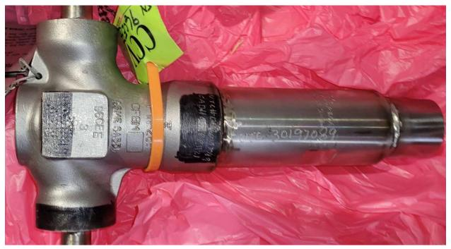
There was evidence that a lock weld had been placed on the adjustment screw that was removed and replaced.
