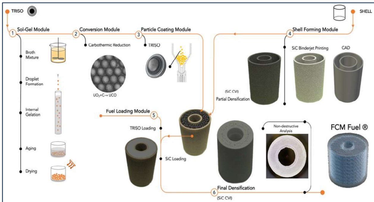
Figure 3.1. Process Flow Diagram of FCM Fuel Manufacturing Process
