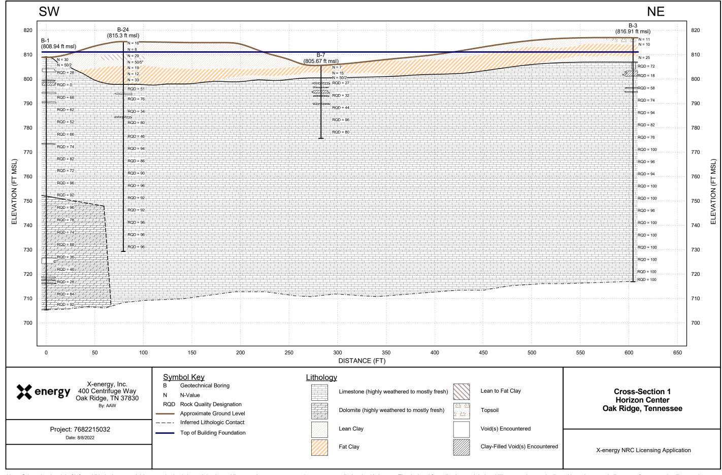
Note: Orientation (angle) of inferred lithologic contact(s) between bedrock (e.g., dolomite and limestone) represents approximate apparent dip (angle, 19 degrees E) calculated from dip observed during drilling operations and adjusted based on actual alignment of cross-section illustrated on the 20:50 vertical-to-horizontal exaggerated-profile scale. N-value and rock quality designation displayed approximately at the mid-point of the run.
