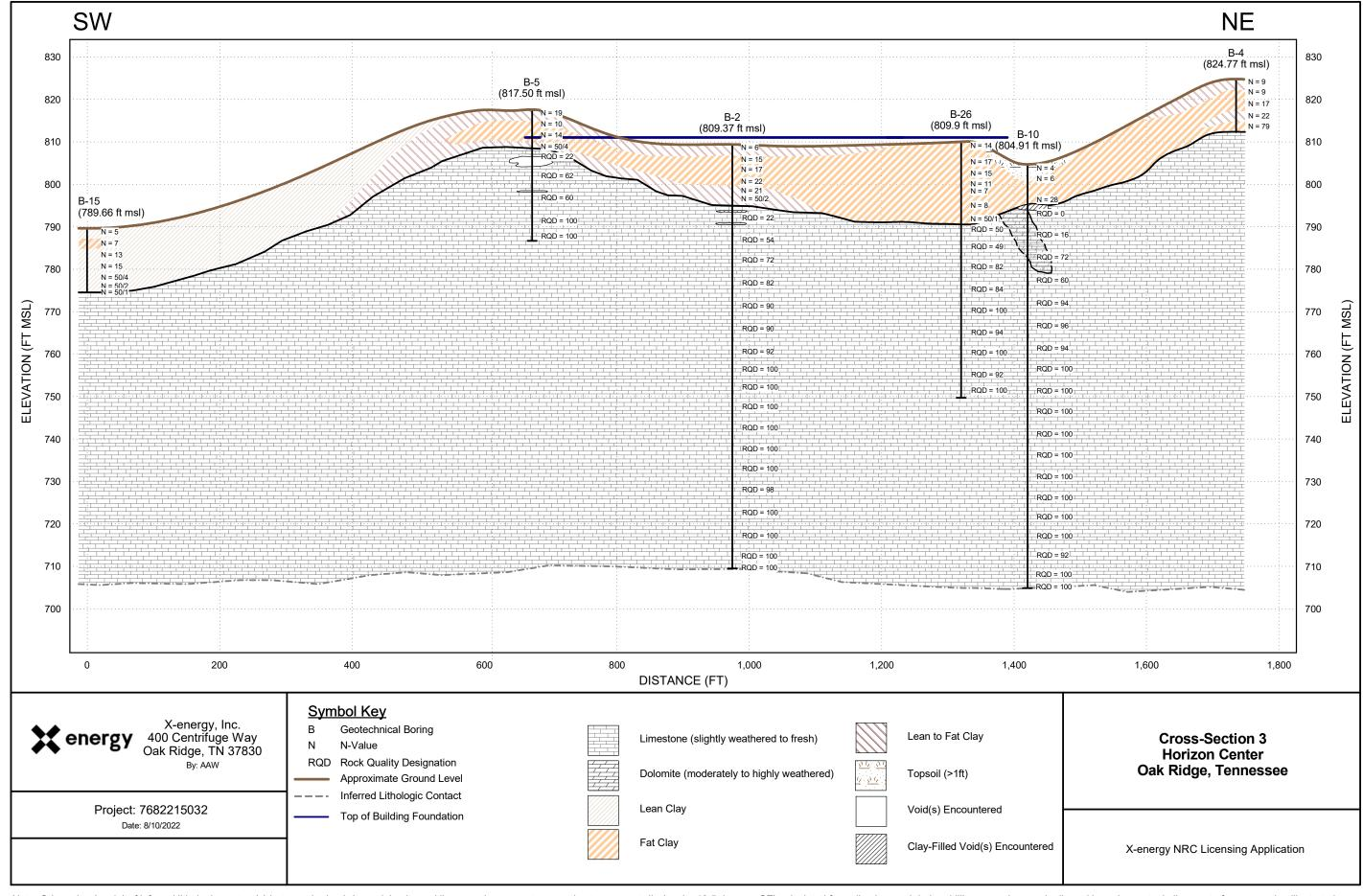
Note: Orientation (angle) of inferred lithologic contact(s) between bedrock (e.g., dolomite and limestone) represents approximate apparent dip (angle, 13.5 degrees SE) calculated from dip observed during drilling operations and adjusted based on actual alignment of cross-section illustrated on the 30:200 vertical-to-horizontal exaggerated-profile scale. N-value and rock quality designation displayed approximately at the mid-point of the run.
