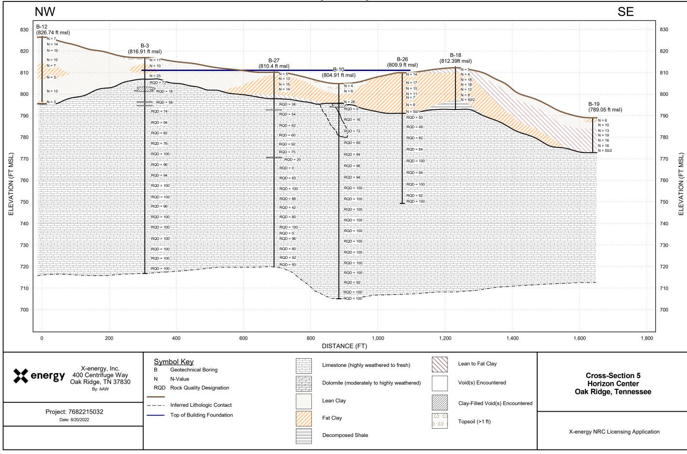
Note: Orientation (angle) of inferred lithologic contact(s) between bedrock (e.g., dolomite and limestone) represents approximate apparent dip (angle, 13.5 degrees SE) calculated from dip observed during drilling operations and adjusted based on actual alignment of cross-section illustrated on the 40:200 vertical-to-horizontal exaggerated-profile scale. N-value and rock quality designation displayed approximately at the mid-point of the run.
