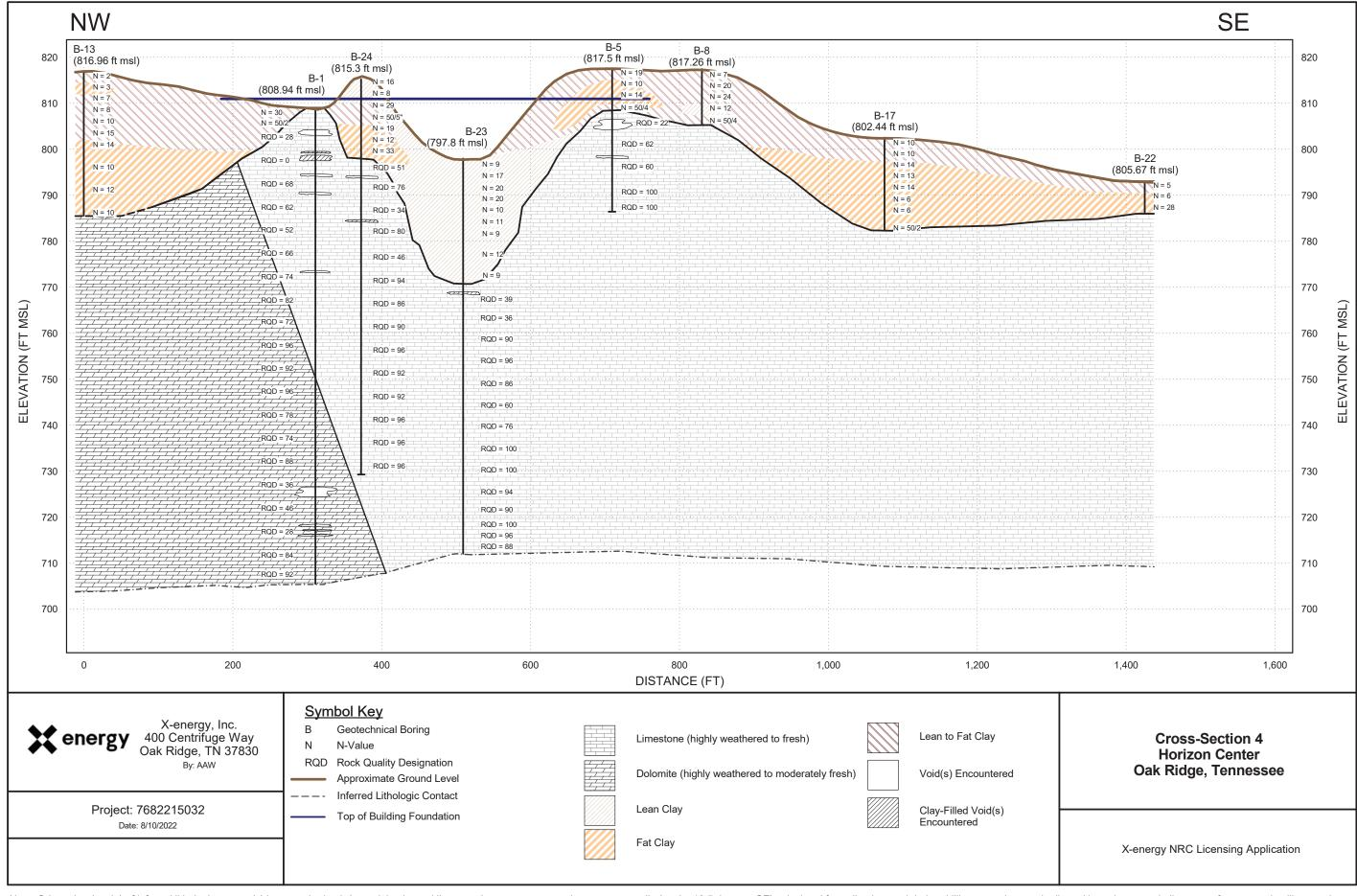
Note: Orientation (angle) of inferred lithologic contact(s) between bedrock (e.g., dolomite and limestone) represents approximate apparent dip (angle, 13.5 degrees SE) calculated from dip observed during drilling operations and adjusted based on actual alignment of cross-section illustrated on the 34:200 vertical-to-horizontal exaggerated-profile scale. N-value and rock quality designation displayed approximately at the mid-point of the run.
