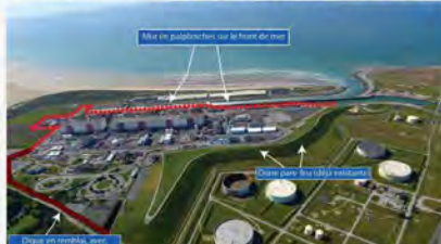
Gravelines (6 reactors of 900 MWe on the sea-side) : recent reinforcement of the dikes
