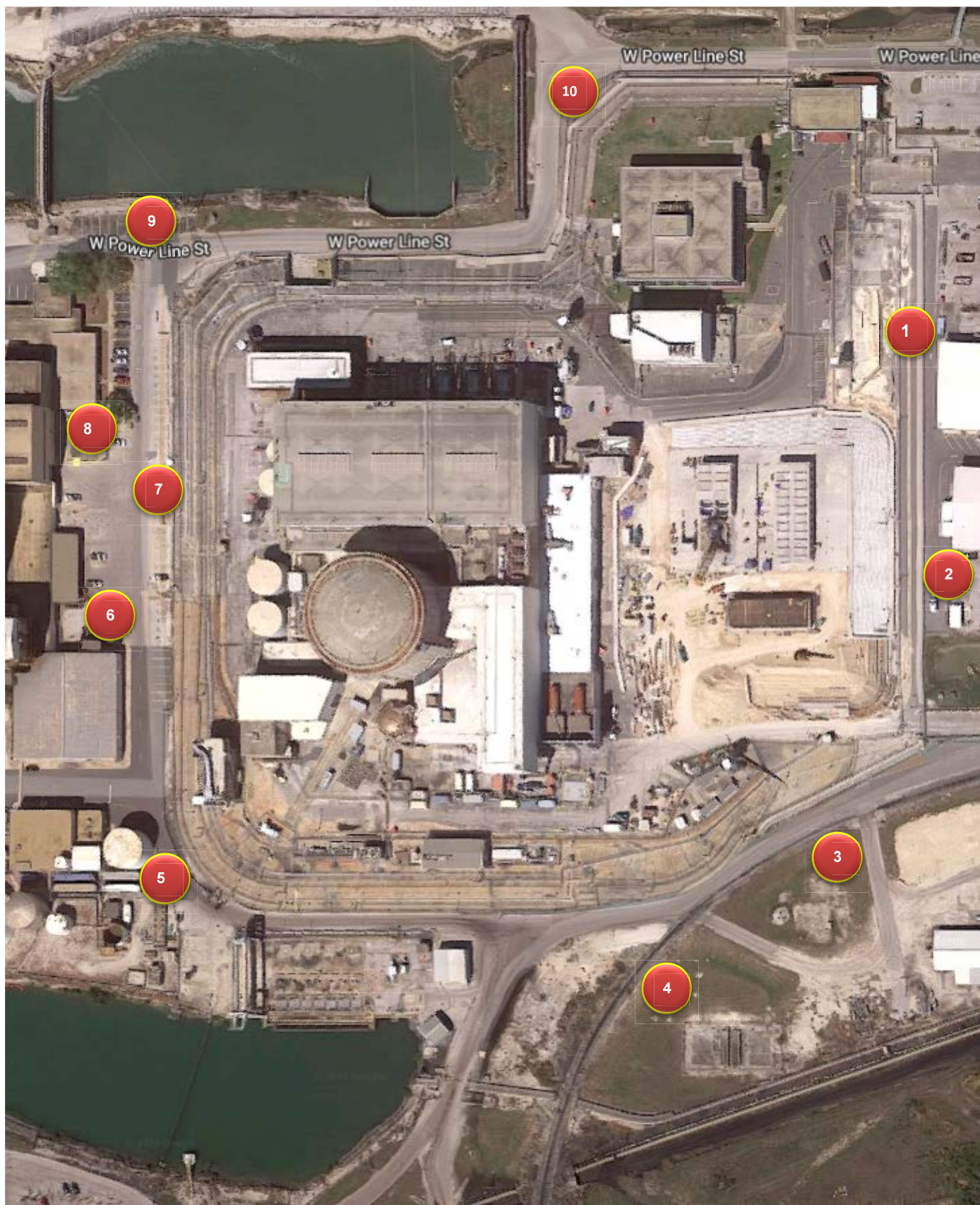
Figure I-4: CR3 Groundwater Monitoring Well Locations Deep Wells Are Also Installed at #'s 1, 3, 6
