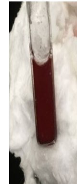
\text{UCl}_3 - \text{RbCl} melt at 850^\circ\text{C}
