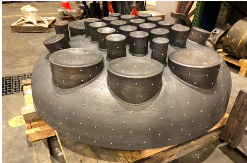
Figure 44. The 44% scale upper vessel head assembly produced by PM-HIP [36].
