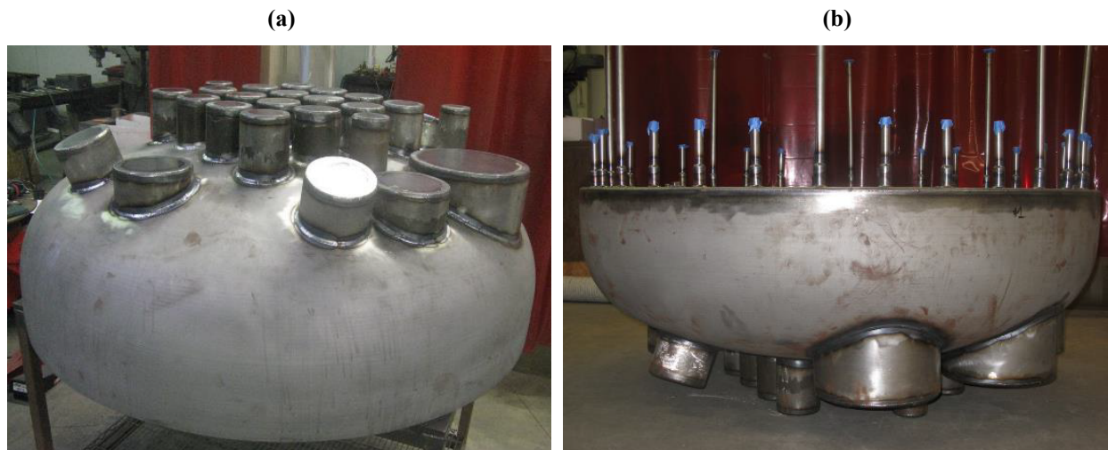
Figure 43. Fabrication can for the 44% scale can of the pressure vessel upper head for the NuScale SMR (a), and completed can with tube stems installed (b) [17].
