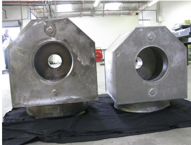
Figure 14. Volumetric shrinkage of large 316L SS valve body powder-filled can before (left) and after HIP (right) [75].
