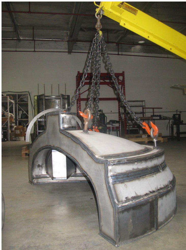
Figure 47. The half-section of the can for the lower vessel head after fabrication and welding [36].
