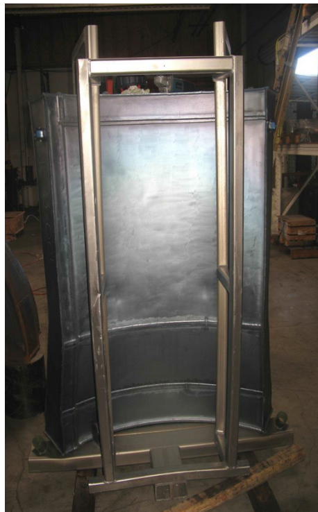
Figure 49. View of the inner surface of the transition shell section after consolidation by HIP [37].
