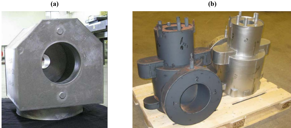
Figure 42. Valve bodies of 316L SS (a) and Grade 91 steel (b) produced by PM-HIP [26].
