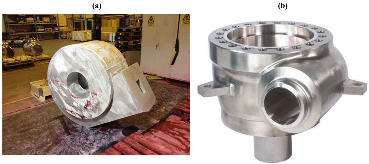
Figure 41. (a) RCP bowl blank produced from 316L SS by PM-HIP after consolidation and can removal (a) and finished machined RCP bowl (b) [31].
