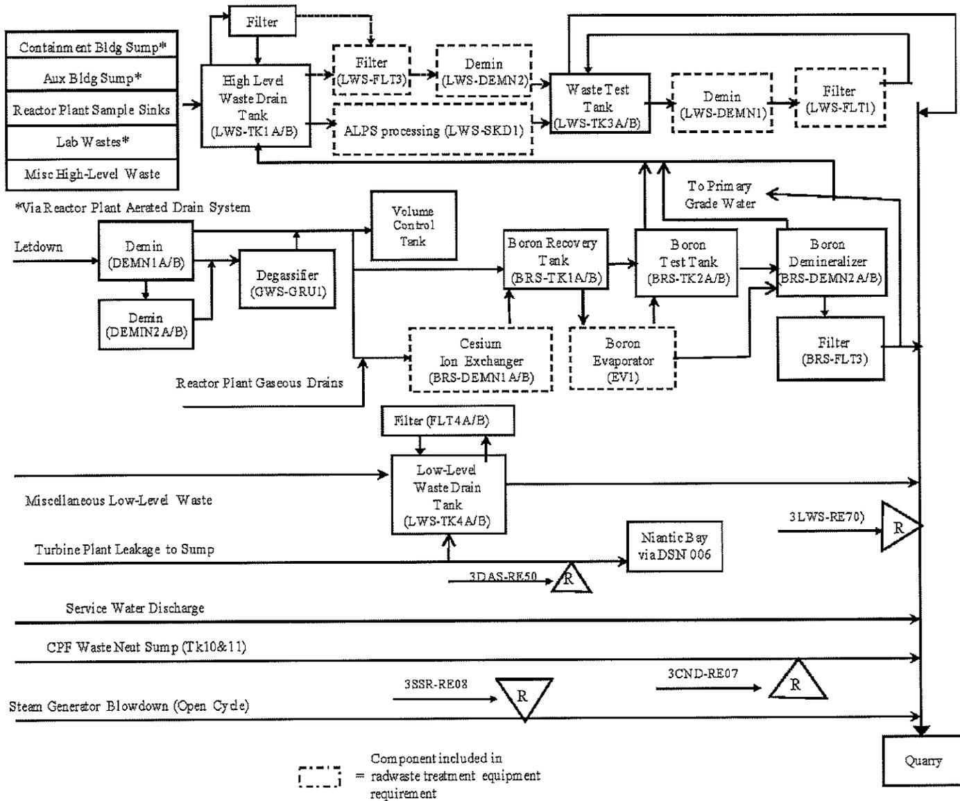
Figure I.C.-3, "Simplified Liquid Effluent Flow Diagram Millstone Unit 3"
