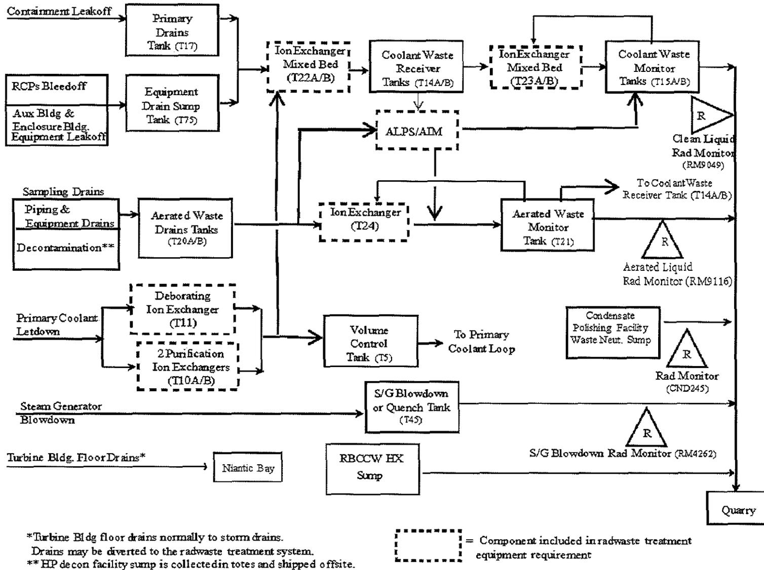
Figure I.C.-2, "Simplified Liquid Effluent Flow Diagram Millstone Unit 2"
