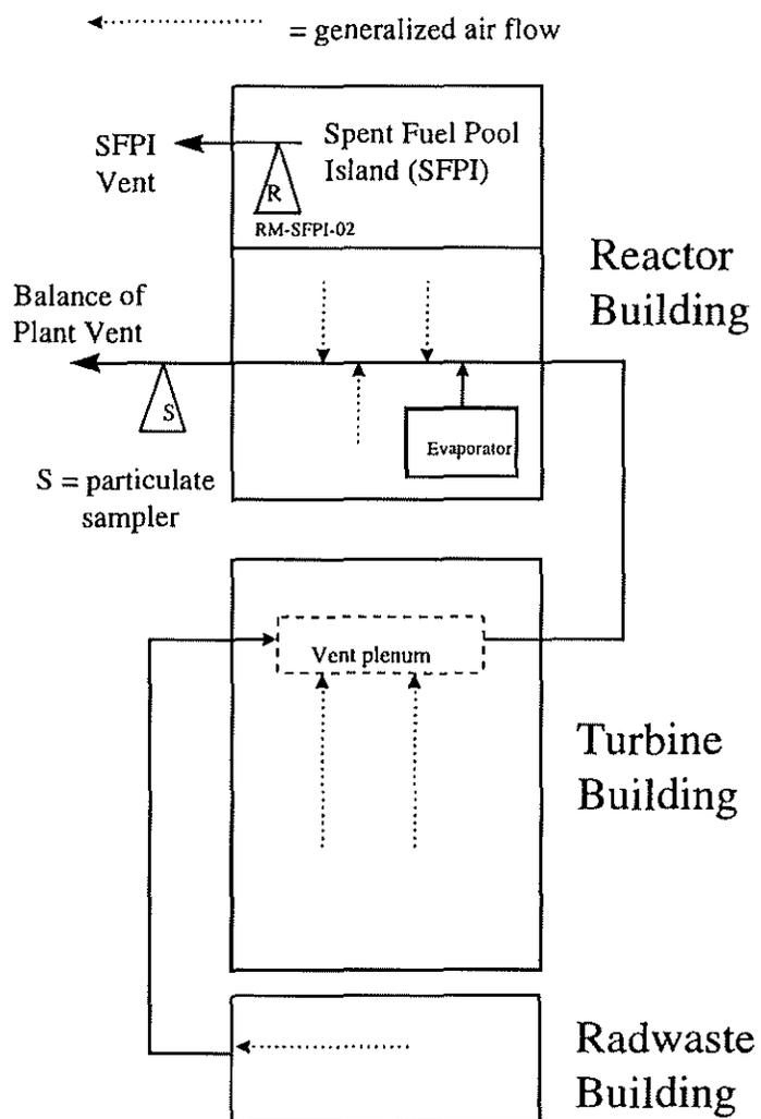
Figure I.D.-2, "Simplified Gaseous Effluent Flow Diagram Millstone Unit Two"
