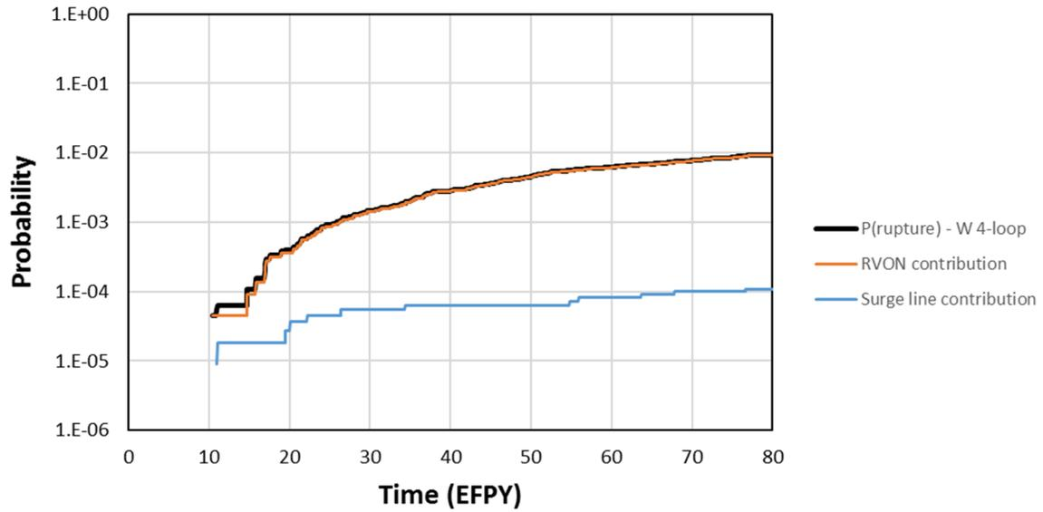
**Figure 4-7 Westinghouse four-loop system probability of rupture and component contributions**
