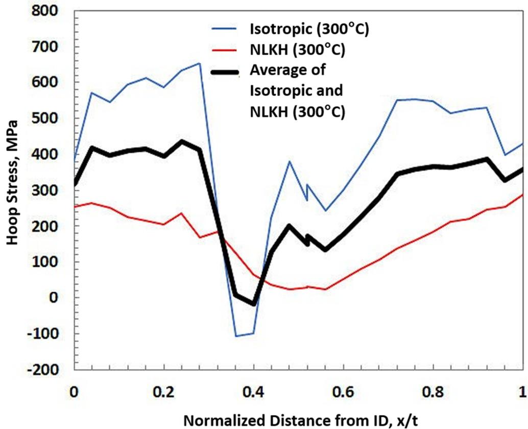
**Figure C-19 Replacement steam generator nozzle hoop WRS profiles**
