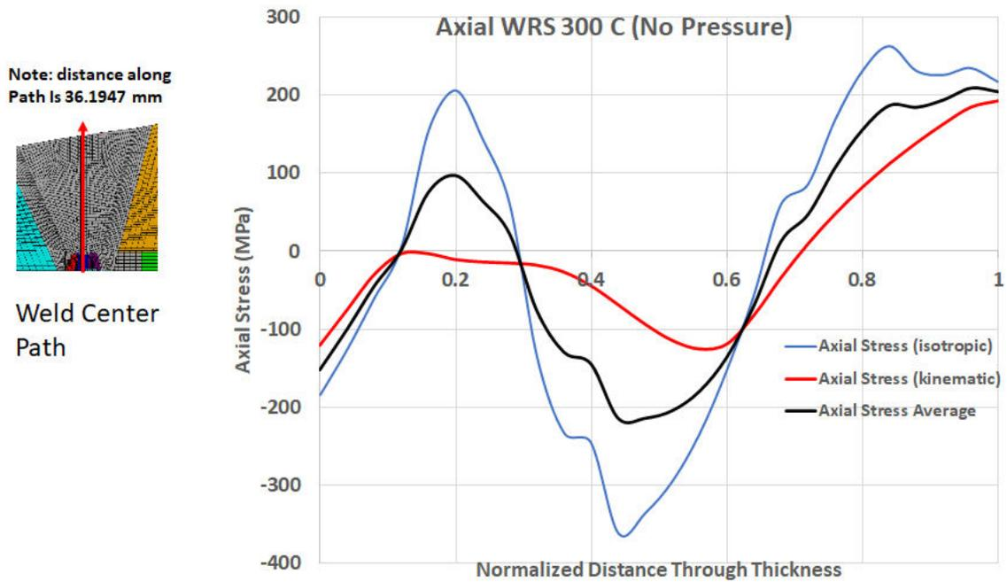
Figure C-29 CE branch line nozzle axial WRS profiles through the weld centerline
