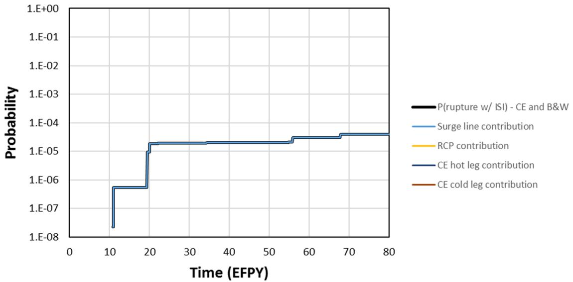
**Figure 4-24 CE and B&W system probability of rupture with a 10-year inspection frequency and component contributions**
