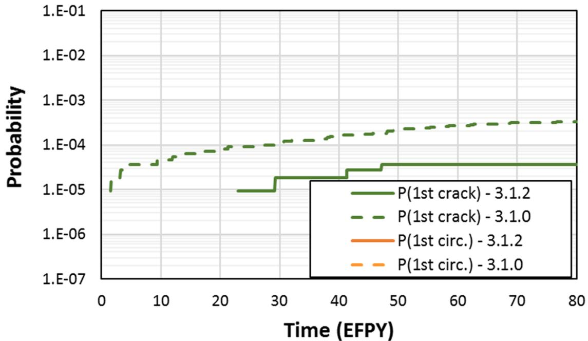
Figure 3-56 Case 3.1.2 time-dependent probabilities of first crack
