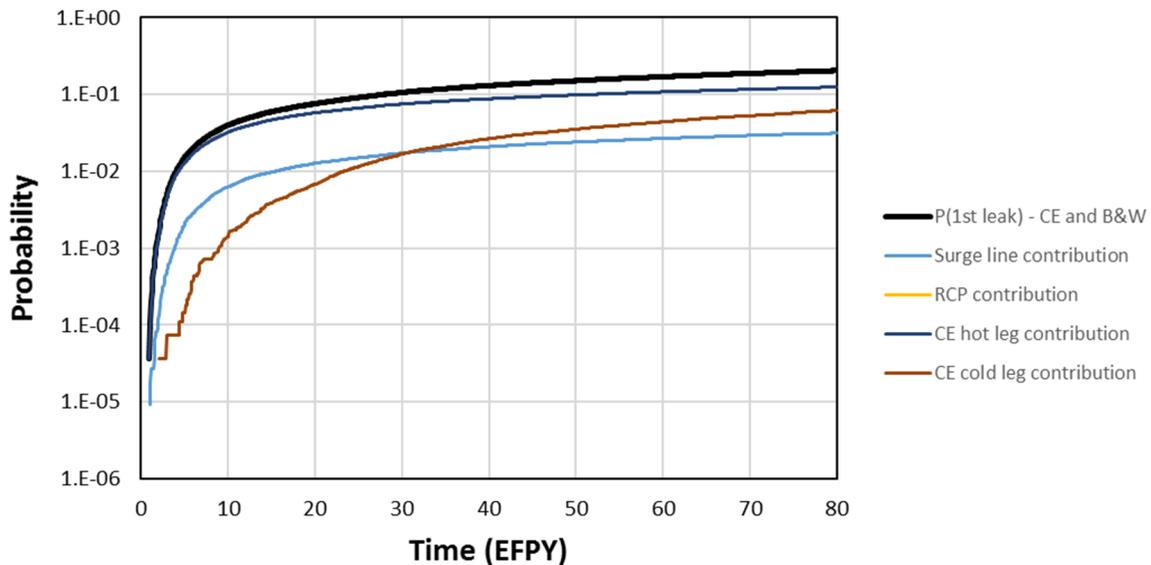
**Figure 4-20 CE and B&W system probability of first leak and component contributions**
