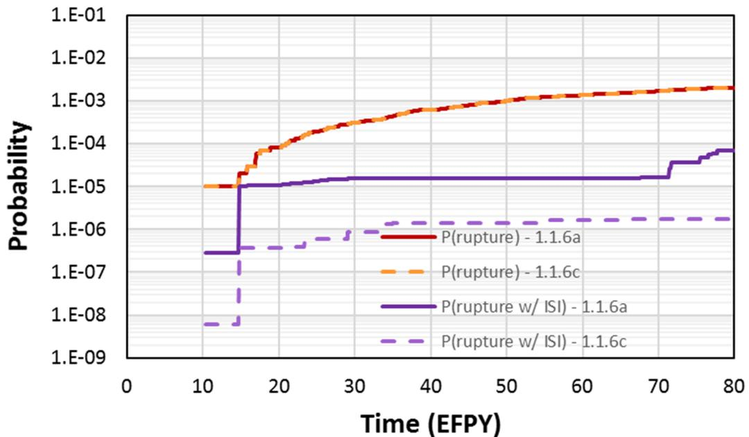
**Figure 3-8 Comparison of Case 1.1.6c time-dependent probabilities of rupture and rupture with ISI with Case 1.1.6a**
