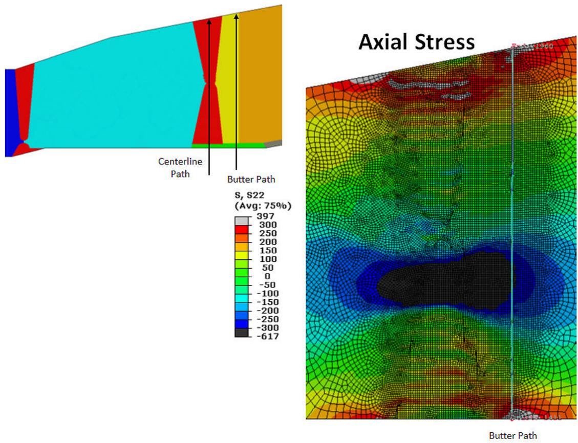
**Figure C-20 Replacement steam generator nozzle baseline axial WRS contour plot generated from FEA**
