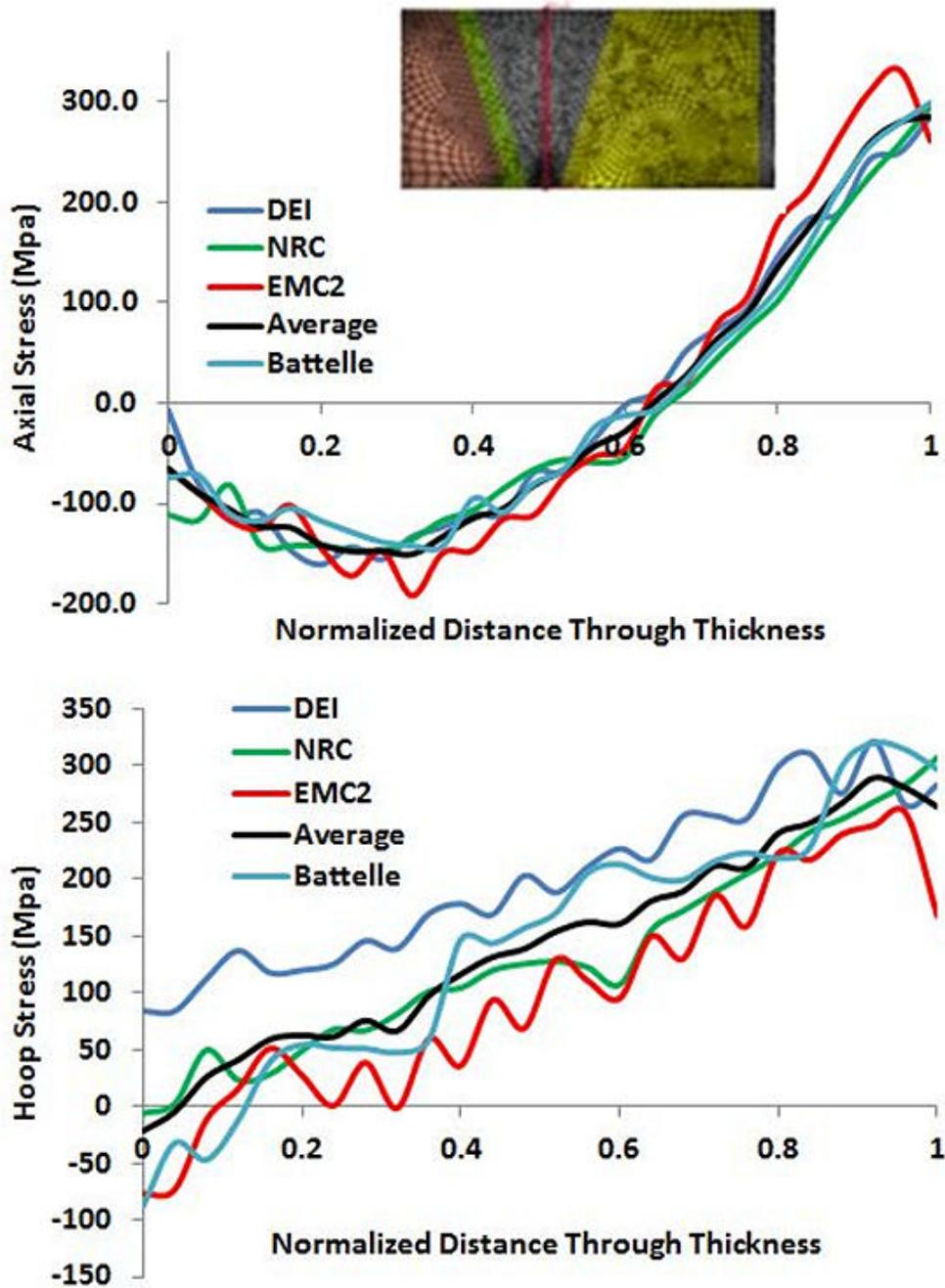
Figure C-39 Axial and hoop WRS profiles for Westinghouse three- and four-loop RVONs
