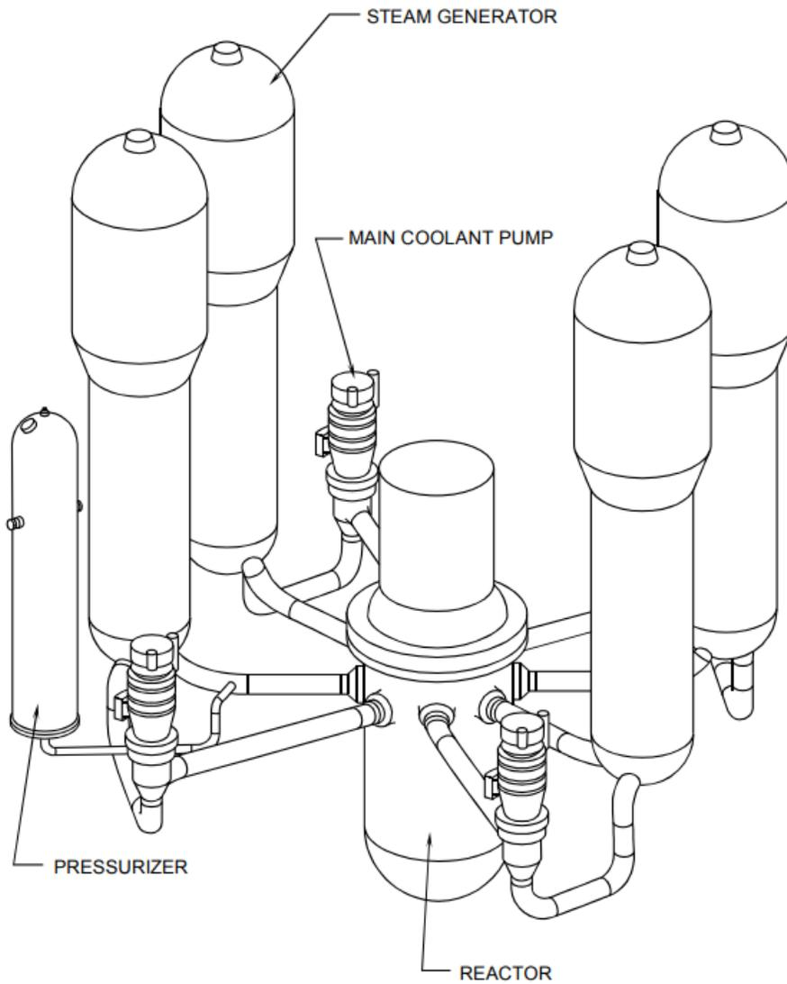
**Figure 2-1** Typical Westinghouse four-loop PWR nuclear steam supply system piping arrangement
