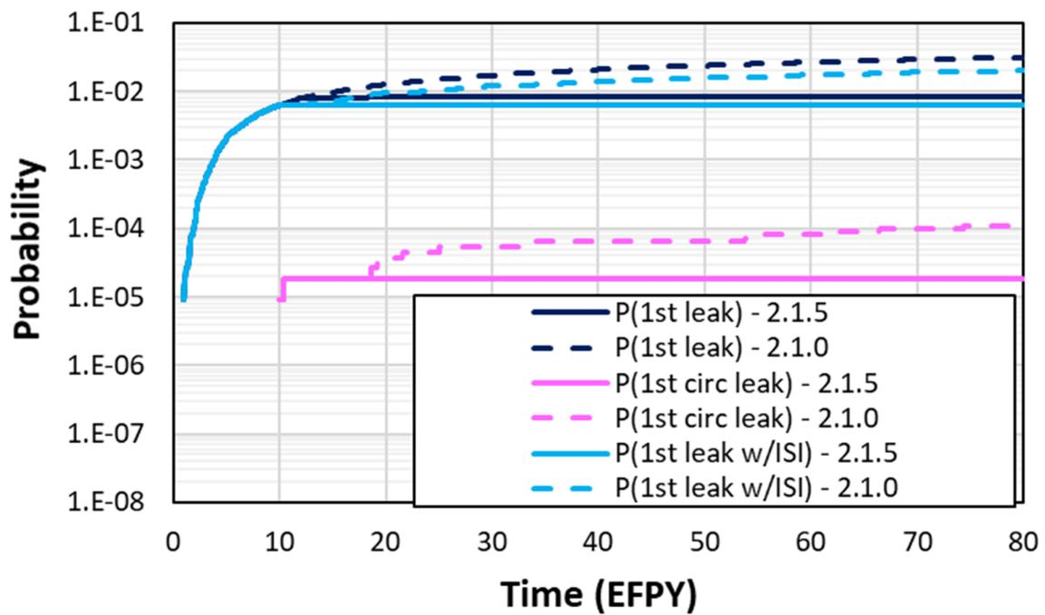
**Figure 3-47 Case 2.1.5 time-dependent probabilities of first leak**
