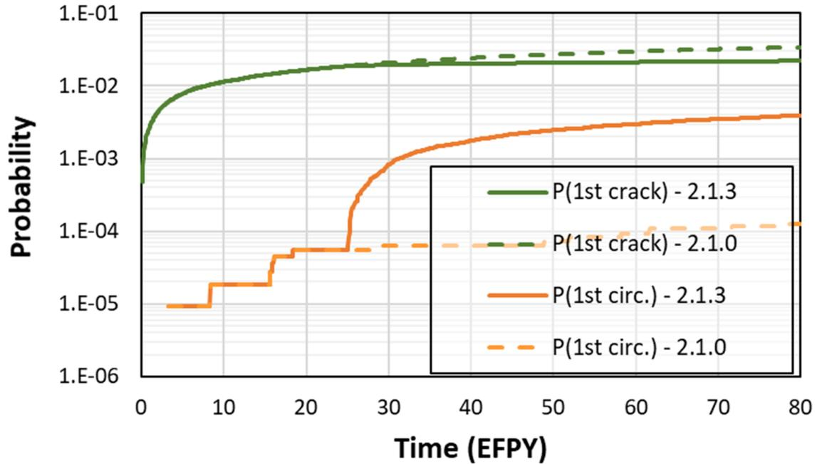
**Figure 3-35 Case 2.1.3 time-dependent probabilities of first crack**
