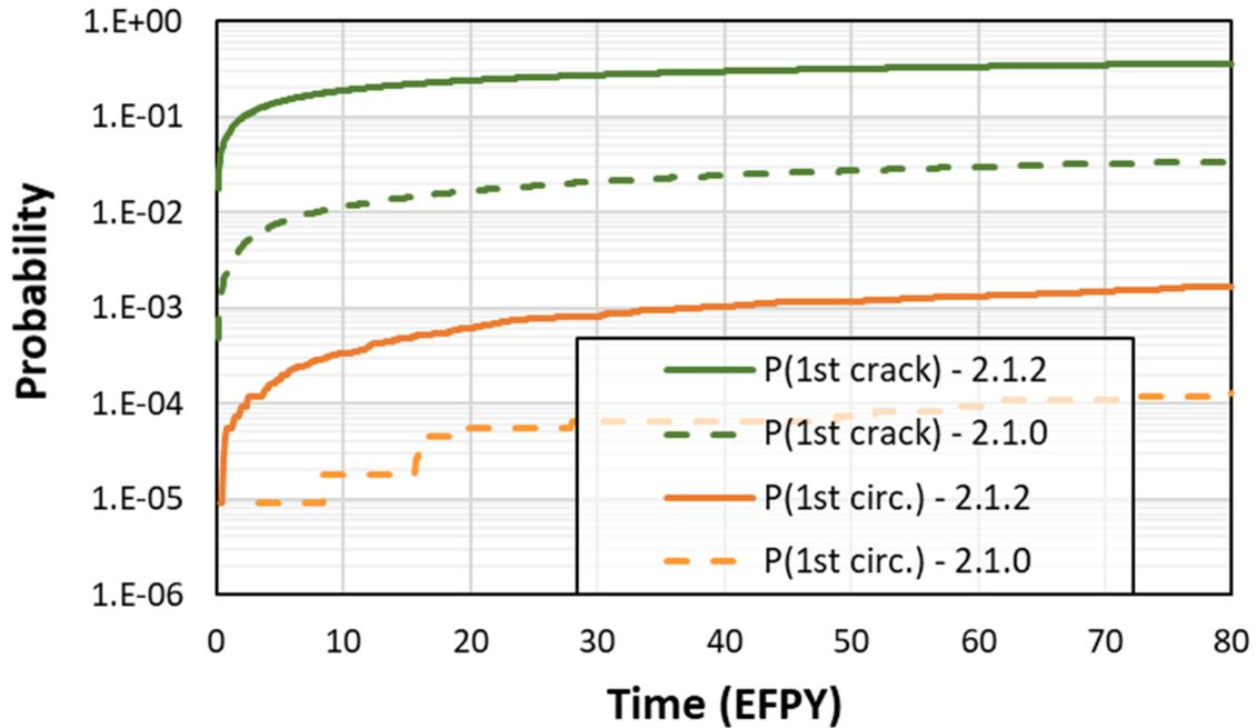
**Figure 3-28 Case 2.1.2 time-dependent probabilities of first crack**
