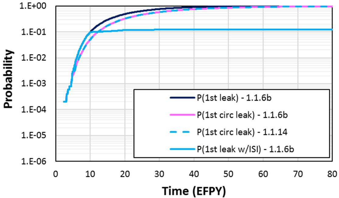
**Figure 3-11 Case 1.1.6b time-dependent probabilities of first leak**
