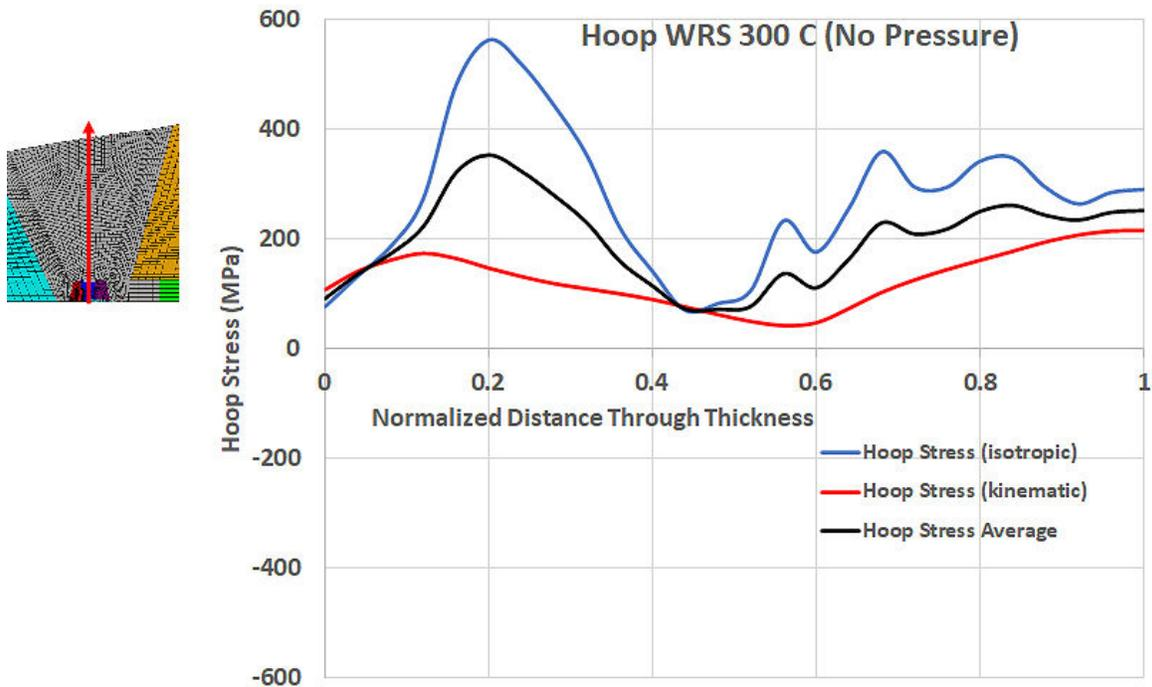
**Figure C-30 CE branch line nozzle hoop WRS profiles through the weld centerline**
