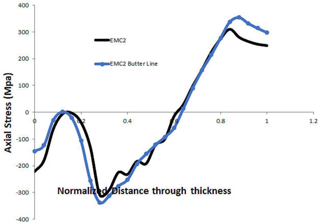
Figure C-14 RCP nozzle axial WRS profiles through the weld centerline and butter from Emc<sup>2</sup>
