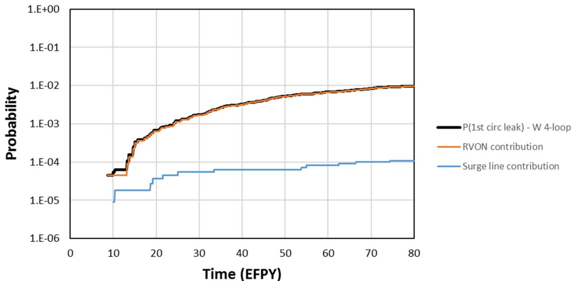
**Figure 4-6 Westinghouse four-loop system probability of first circumferential leak and component contributions**
