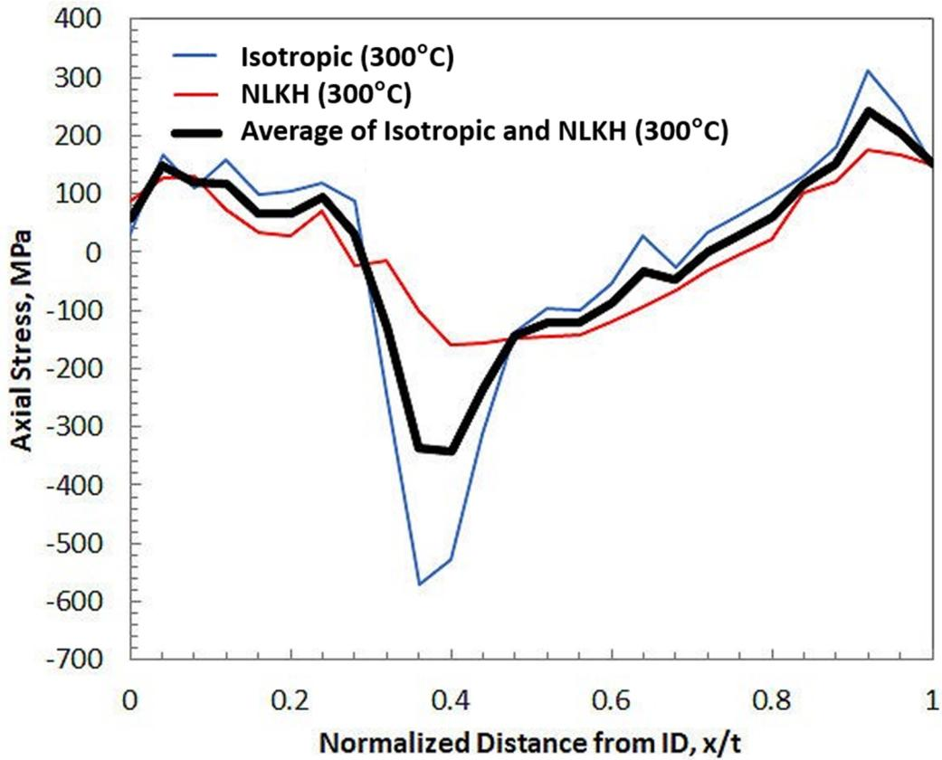
Figure C-18 Replacement steam generator nozzle axial WRS profiles
