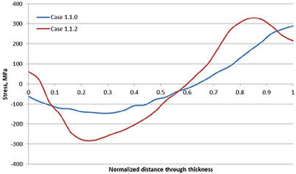
Figure C-43 Comparison of more severe and axial WRS profiles for the RVON weld
