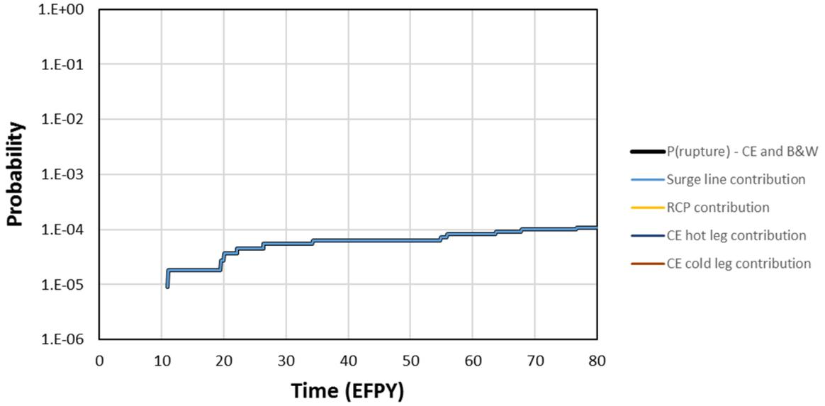
**Figure 4-23 CE and B&W system probability of rupture and component contributions**
