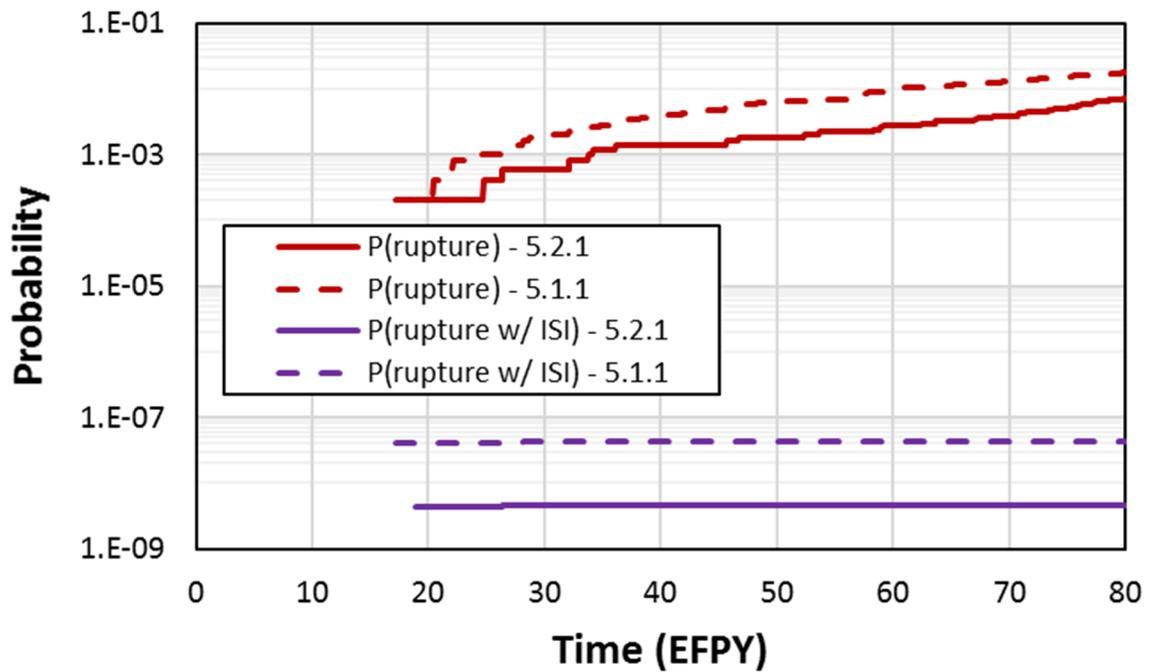
**Figure 3-91 Case 5.2.1 time-dependent probabilities of rupture**
