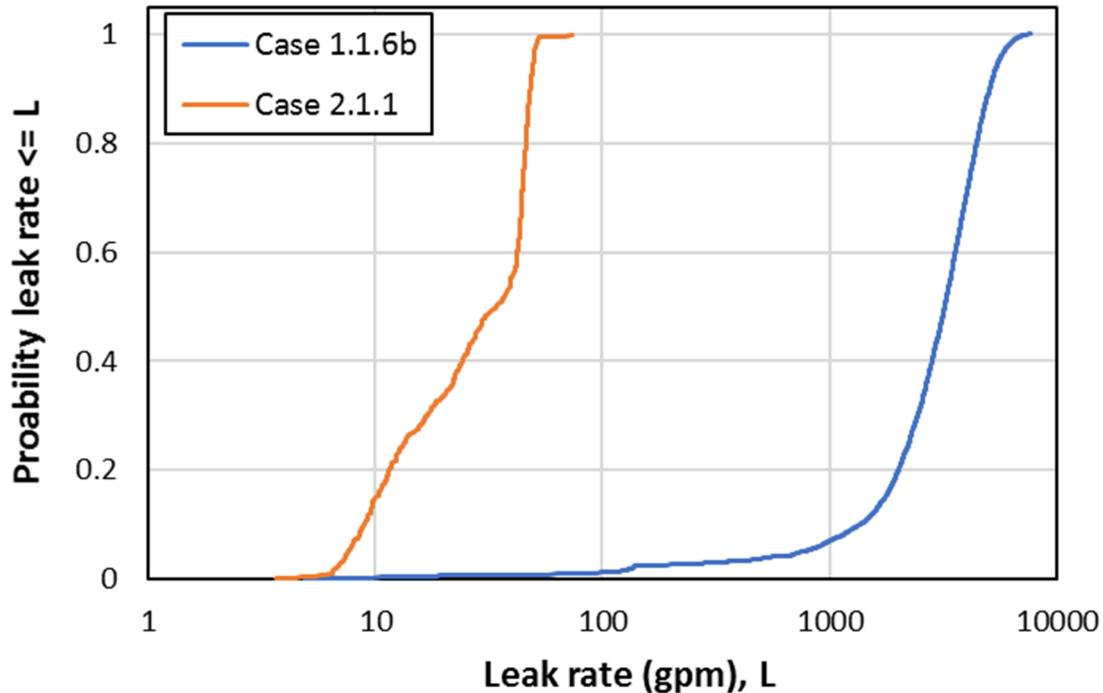
**Figure 3-24 Comparison of Cases 2.1.1 and 1.1.6b leak rates one month before rupture**
