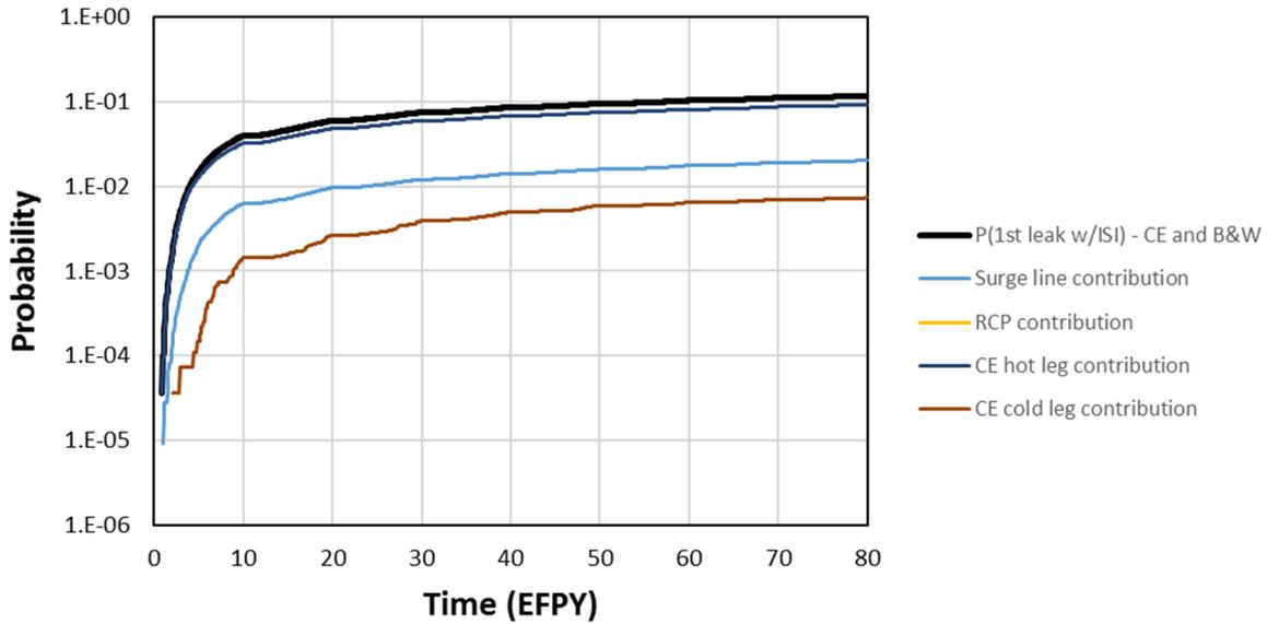
**Figure 4-21 CE and B&W system probability of first leak with a 10-year inspection frequency and component contributions**
