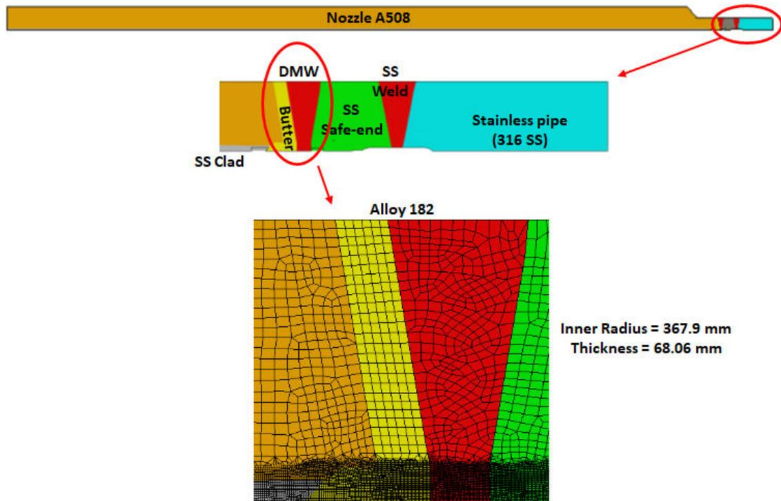
**Figure C-40 RVON nozzle model for more severe WRS profile**
