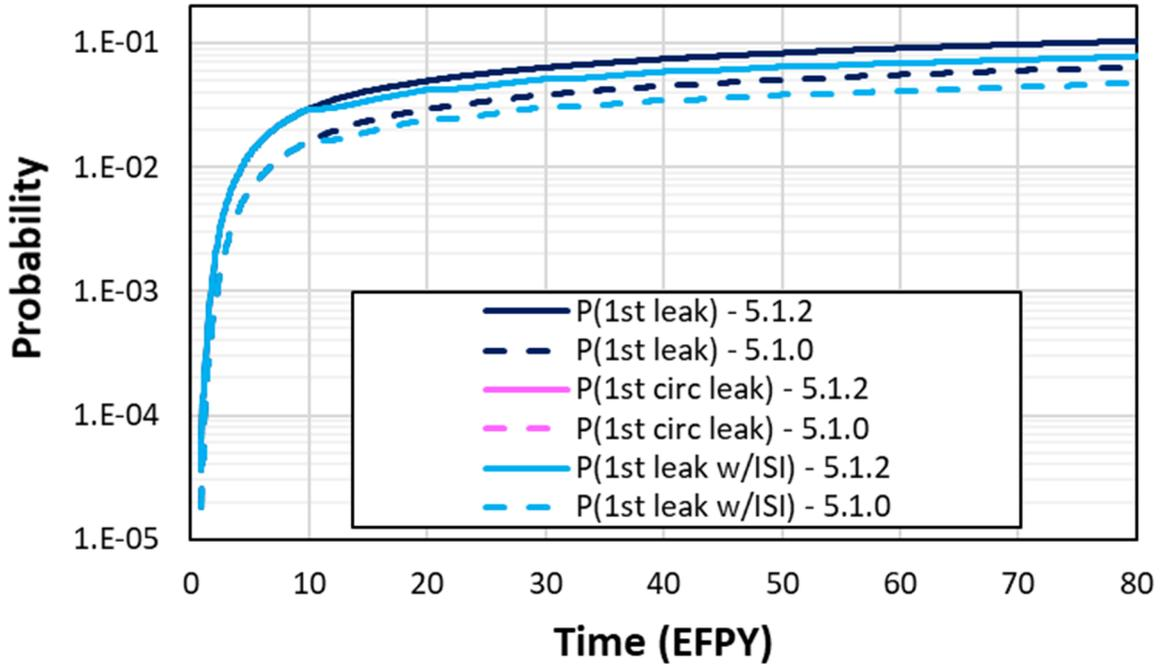
**Figure 3-84 Case 5.1.2 time-dependent probabilities of first leak**
