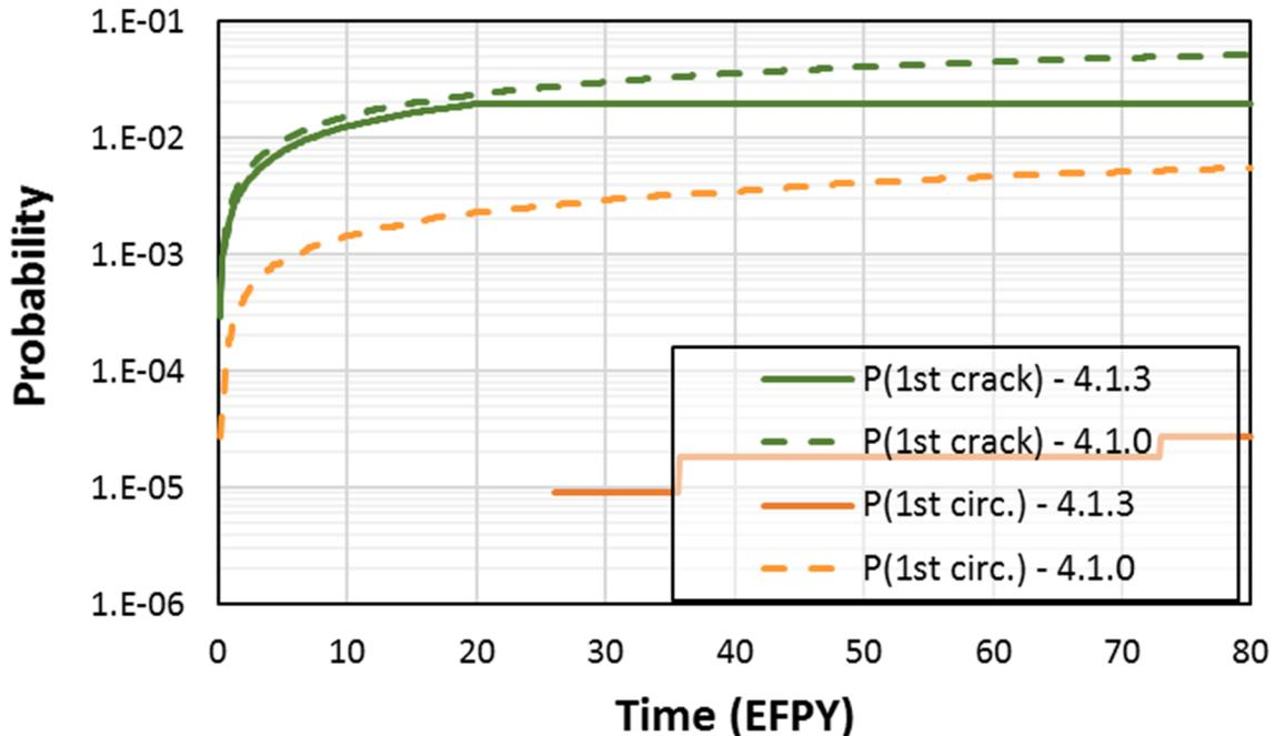
**Figure 3-71 Case 4.1.3 time-dependent probabilities of first crack**
