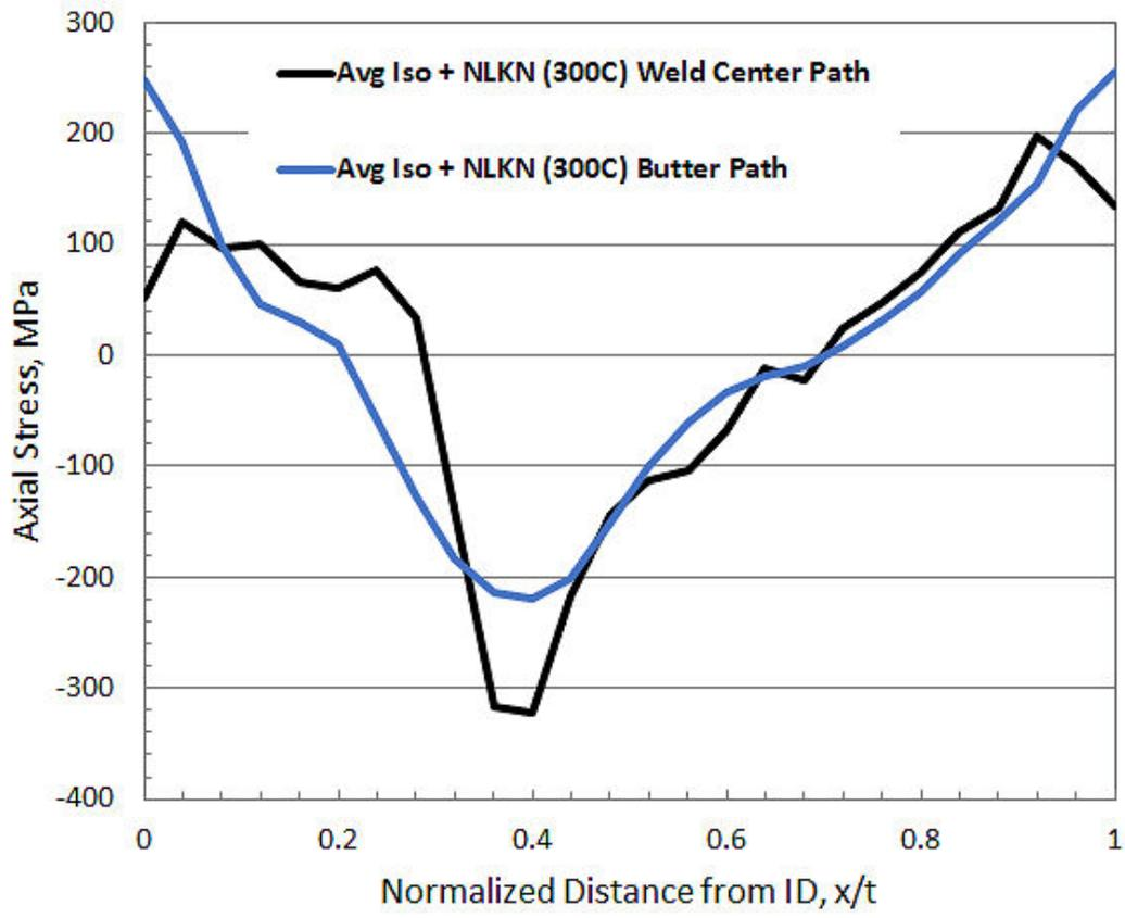
**Figure C-22 Comparison of replacement steam generator nozzle baseline and more severe axial WRS profiles**
