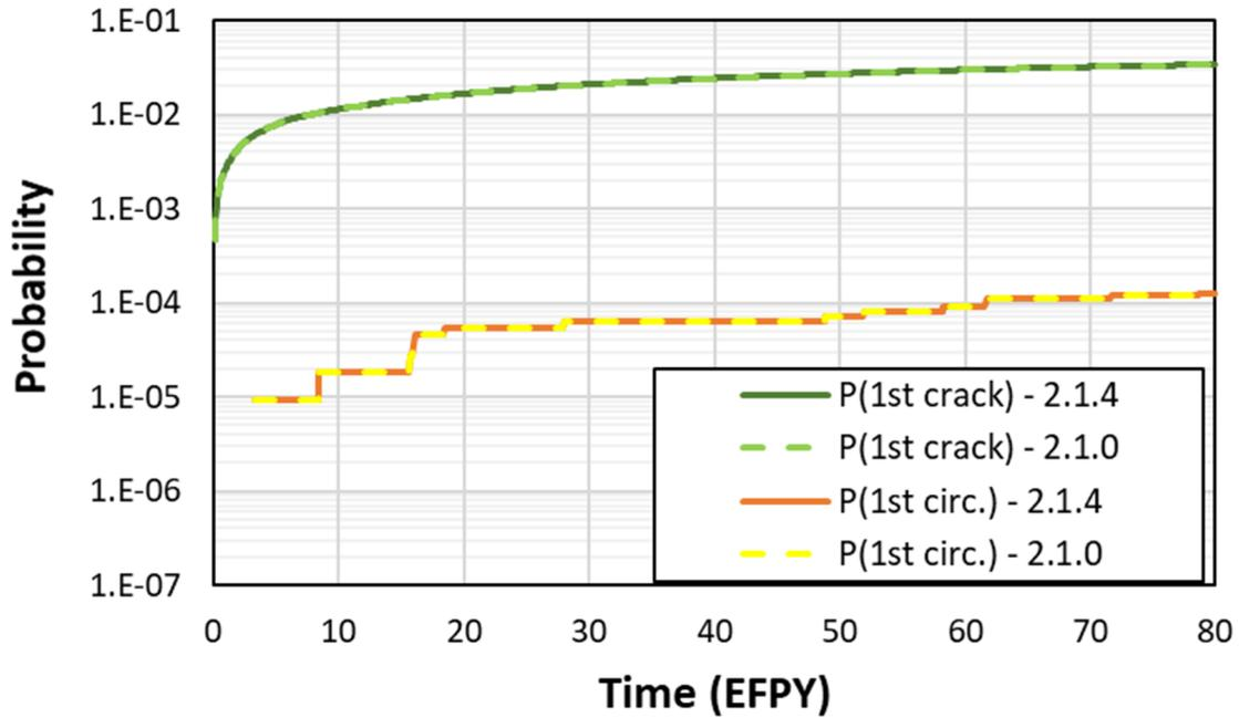
**Figure 3-40 Case 2.1.4 time-dependent probabilities of first crack**
