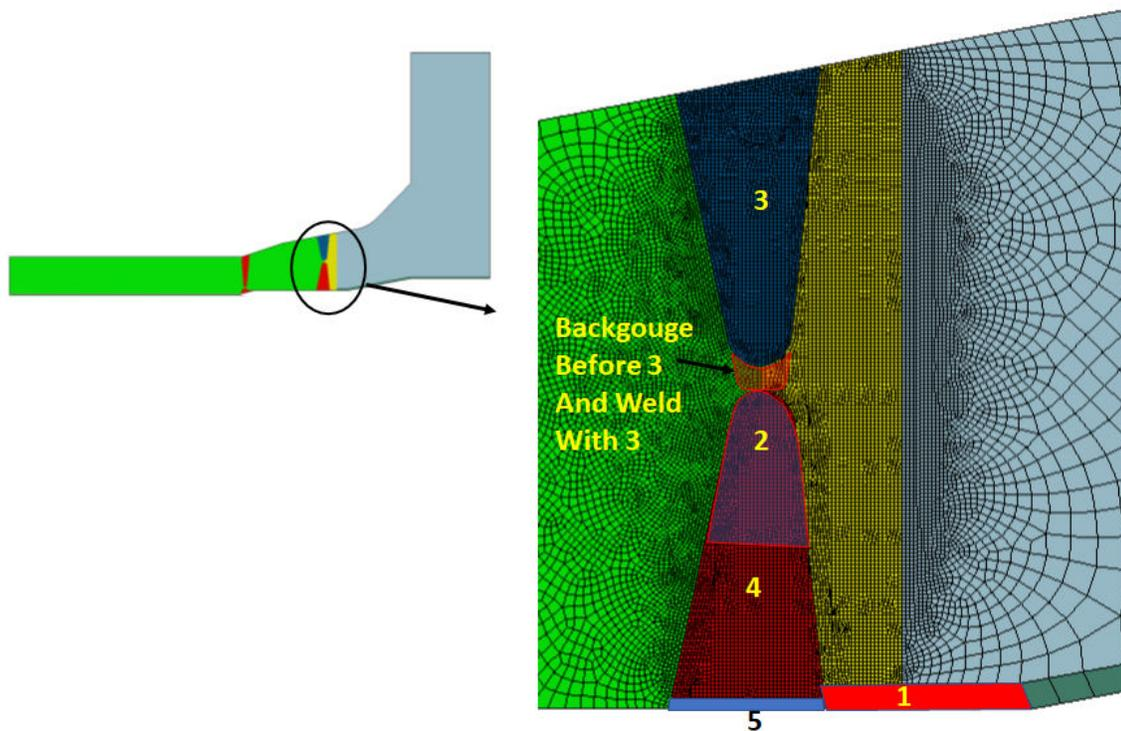
**Figure C-17 FEA model used for replacement steam generator nozzle WRS profile development**
