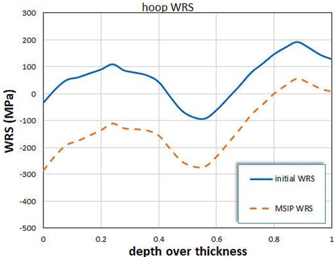
**Figure C-5 Pressurizer surge line nozzle average hoop WRS profiles through the weld centerline**
