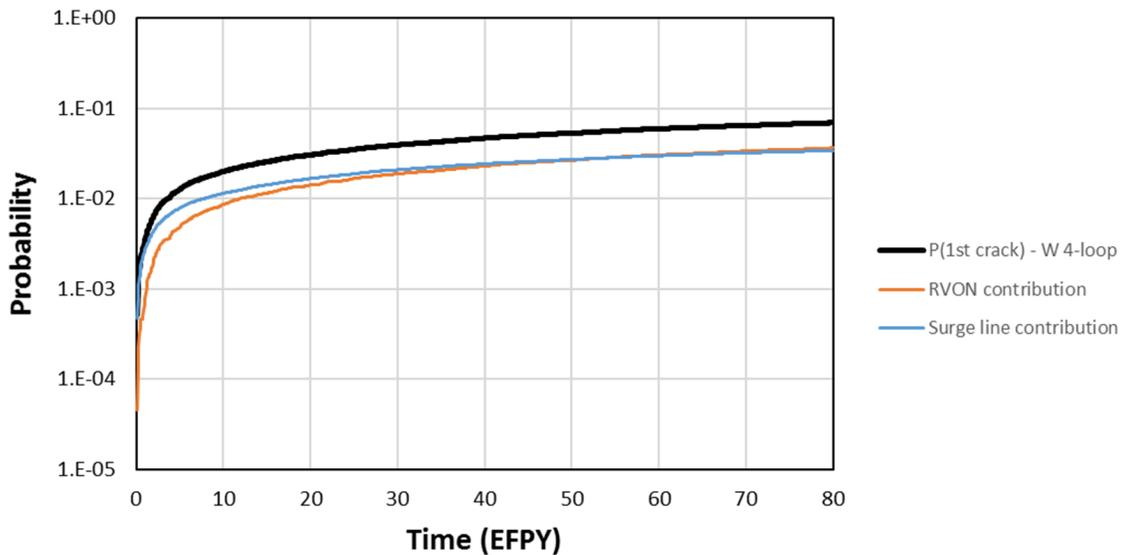
**Figure 4-2 Westinghouse four-loop system probability of first crack and component contributions**
