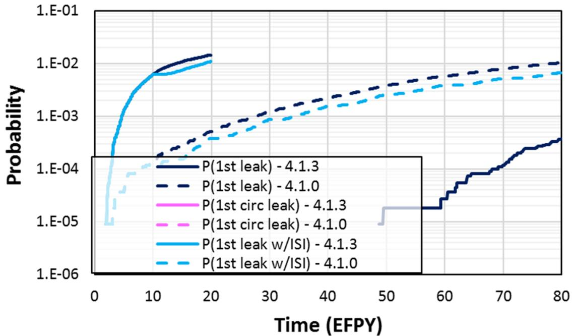
**Figure 3-72 Case 4.1.3 time-dependent probabilities of first leak**
