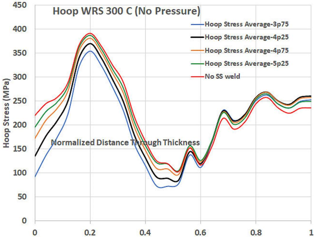
**Figure C-38** Hoop WRS profiles for CE branch line considering different DMW to SS closure weld distances
