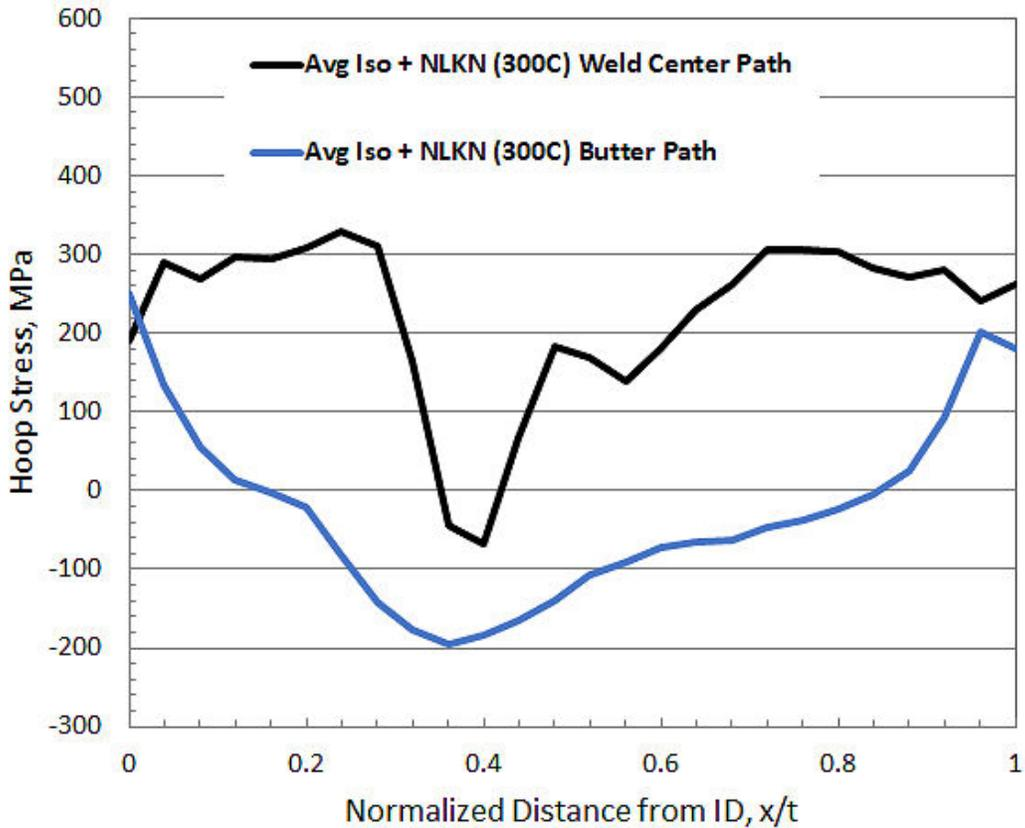
**Figure C-23 Comparison of replacement steam generator nozzle and more severe hoop WRS profiles**
