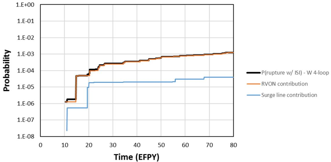
**Figure 4-8 Westinghouse four-loop system probability of rupture with 10-year inspection frequency and component contributions**
