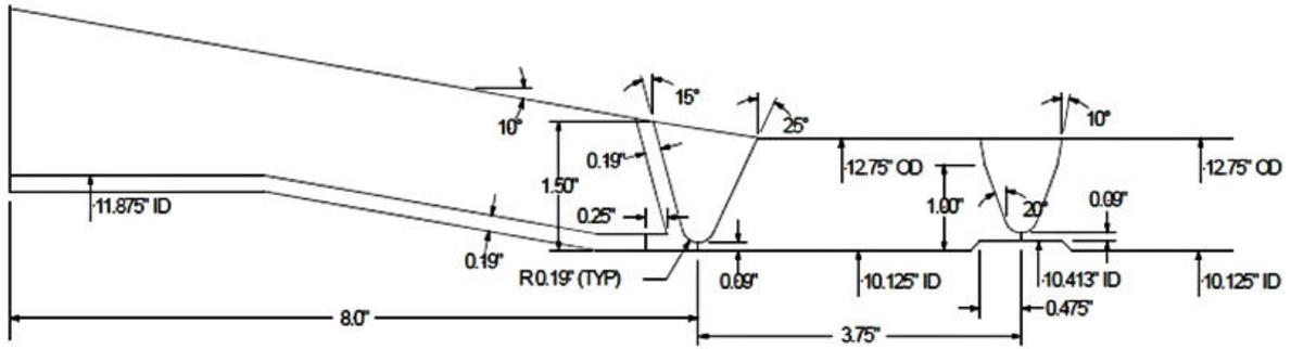
**Figure C-24 Representative CE branch line nozzle geometry and dimensions**
