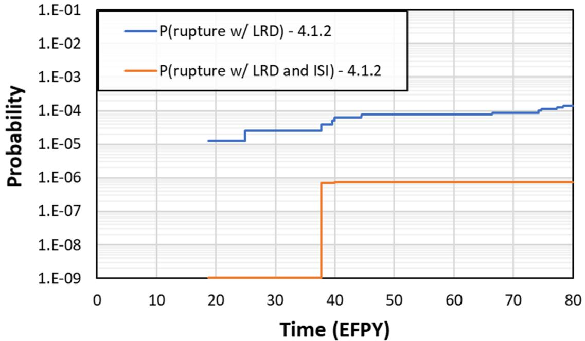
**Figure 3-65 Case 4.1.2 time-dependent probabilities of rupture with leak rate detection**
