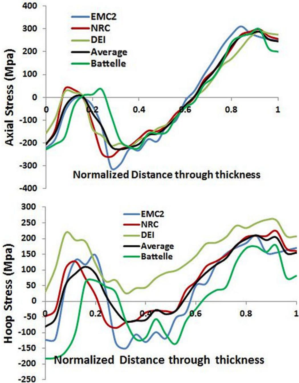
Figure C-11 RCP nozzle axial and hoop WRS profiles through the weld centerline
