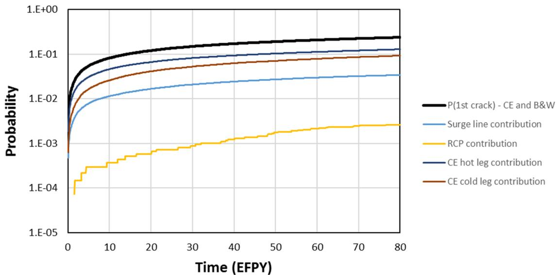
**Figure 4-18 CE and B&W system probability of first crack and component contributions**
