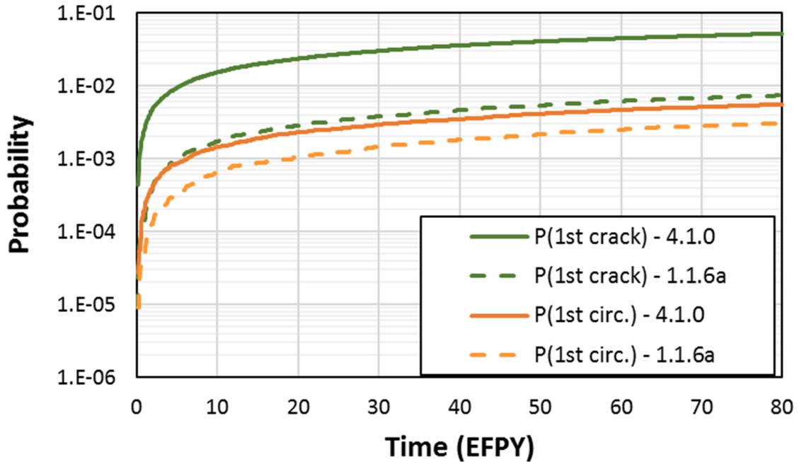
**Figure 3-58 Case 4.1.0 time-dependent probabilities of first crack**
