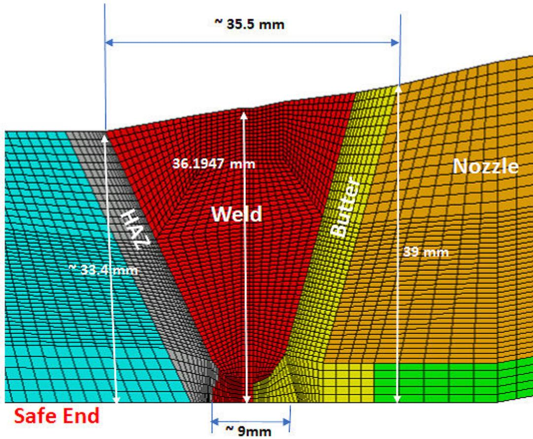
Figure C-26 Details of FEA model used for CE branch line nozzle WRS profile development
