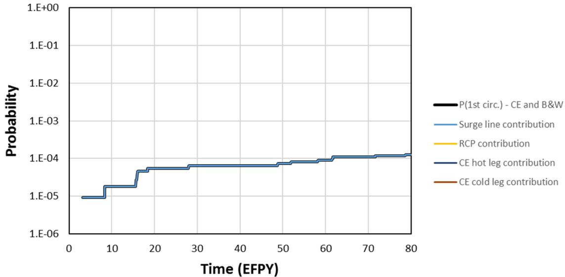
**Figure 4-19 CE and B&W system probability of first circumferential crack and component contributions**
