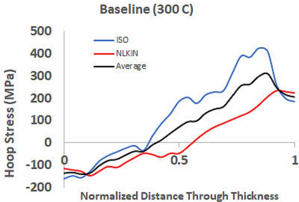
Figure C-42 More severe axial and hoop WRS profiles for the RVON weld
