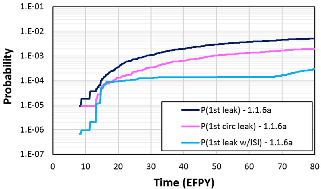
**Figure 3-5 Case 1.1.6a time-dependent probabilities of first leak with a 10-year inspection frequency**
