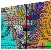
**Step 1 - Apply 36 DM Alloy 182 weld passes. Neglect modeling butter Passes and PWHT since this has small effect on DMW WRS**
