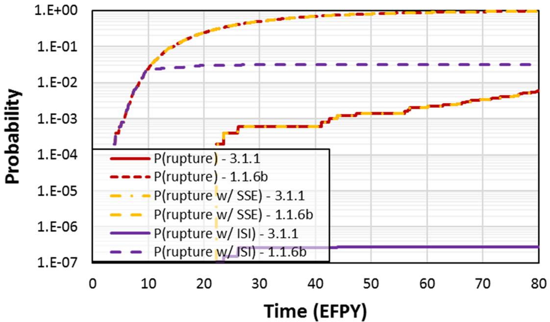
**Figure 3-54 Case 3.1.1 time-dependent probabilities of rupture**
