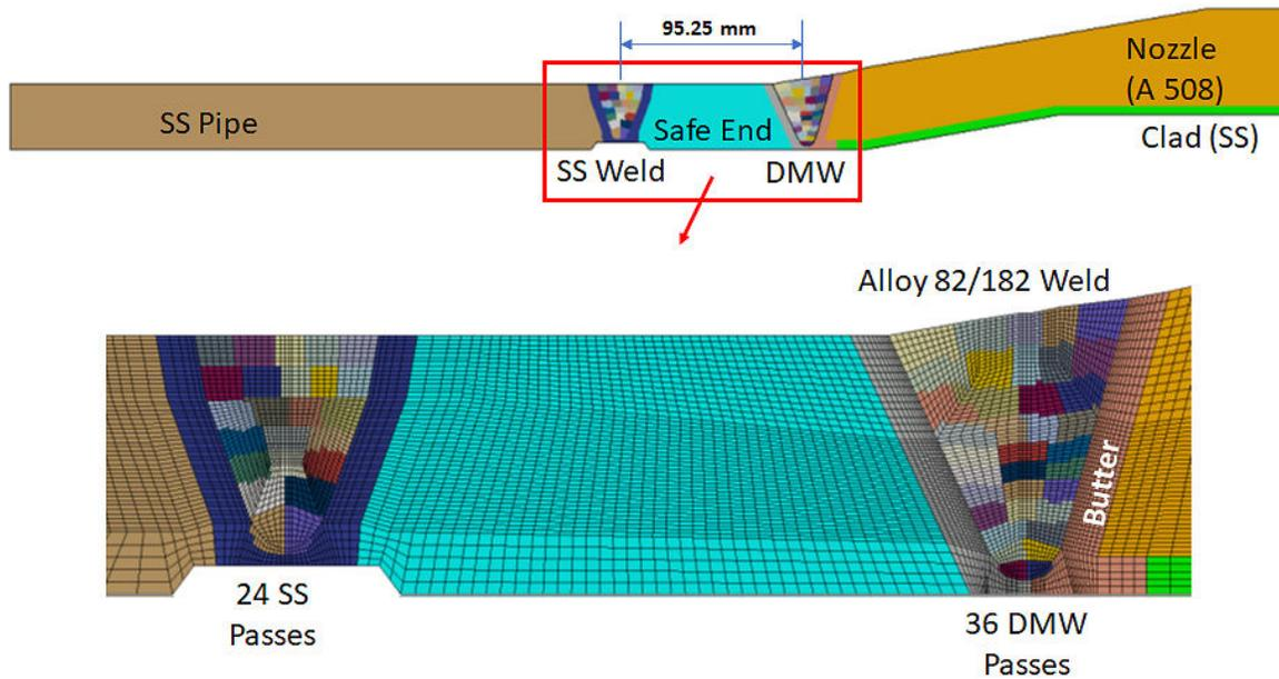
**Figure C-25 FEA model used for CE branch line nozzle WRS profile development**
