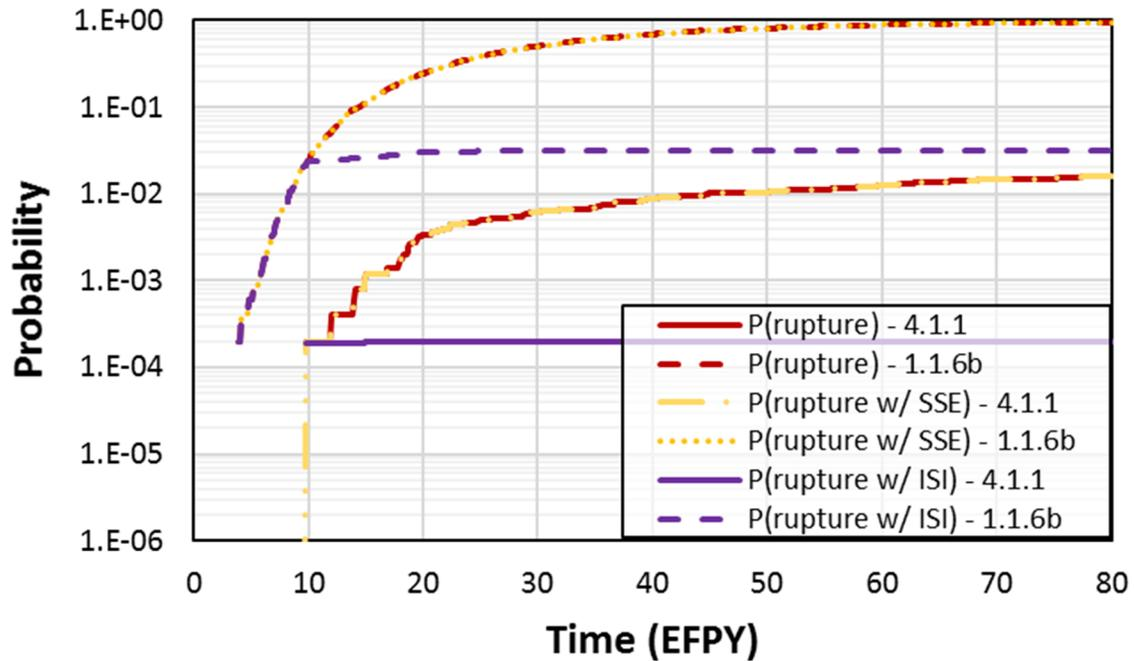
**Figure 3-62 Case 4.1.1 time-dependent probabilities of rupture**
