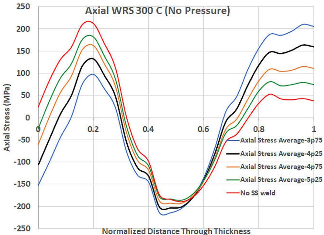
**Figure C-37** Axial WRS profiles for CE branch line considering different DMW to SS closure weld distances
