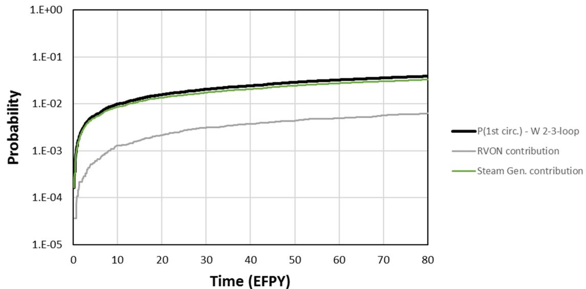
**Figure 4-11 Westinghouse two- and three-loop system probability of first circumferential crack and component contributions**
