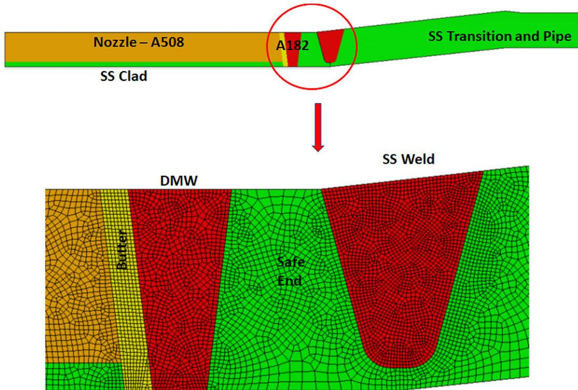
Figure C-10 FEA model used for RCP nozzle WRS profile development
