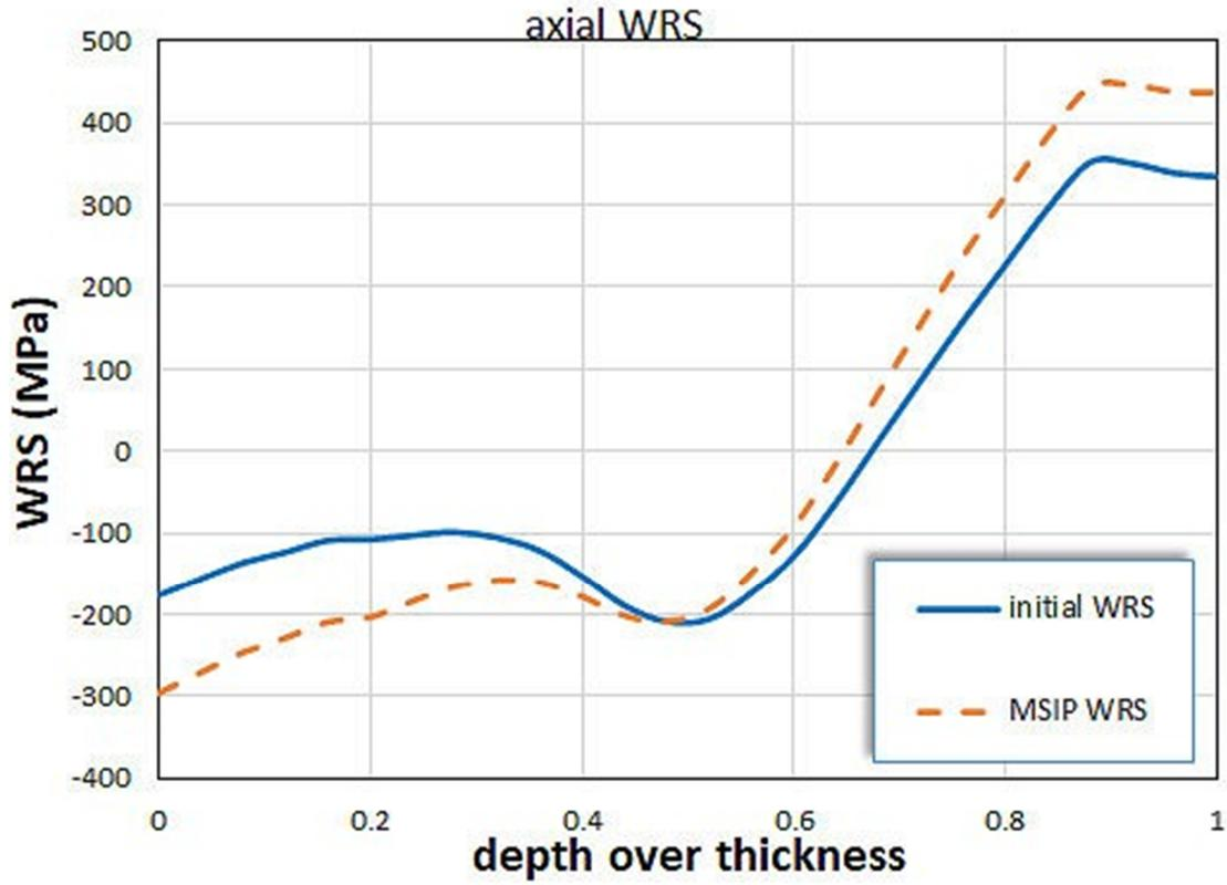
Figure C-4 Pressurizer surge line nozzle average axial WRS profiles through the weld centerline
