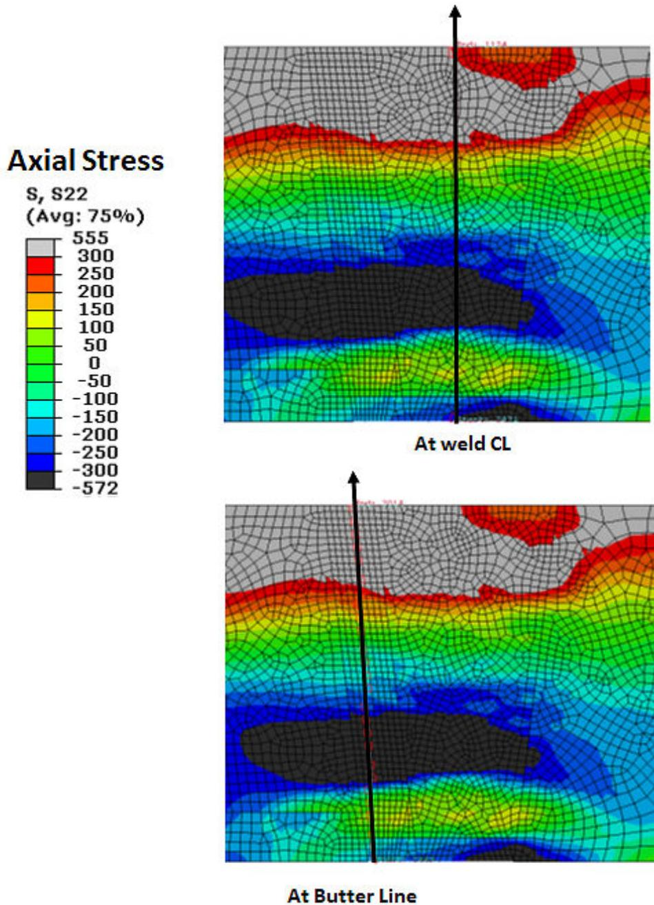
**Figure C- 12 RCP nozzle axial WRS contour plots generated from FEA with isotropic hardening law**
