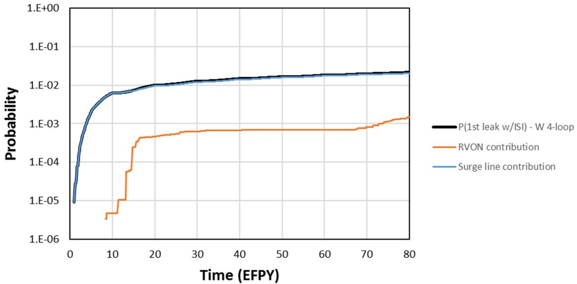
**Figure 4-5 Westinghouse four-loop system probability of first leak with a 10-year inspection frequency and component contributions**
