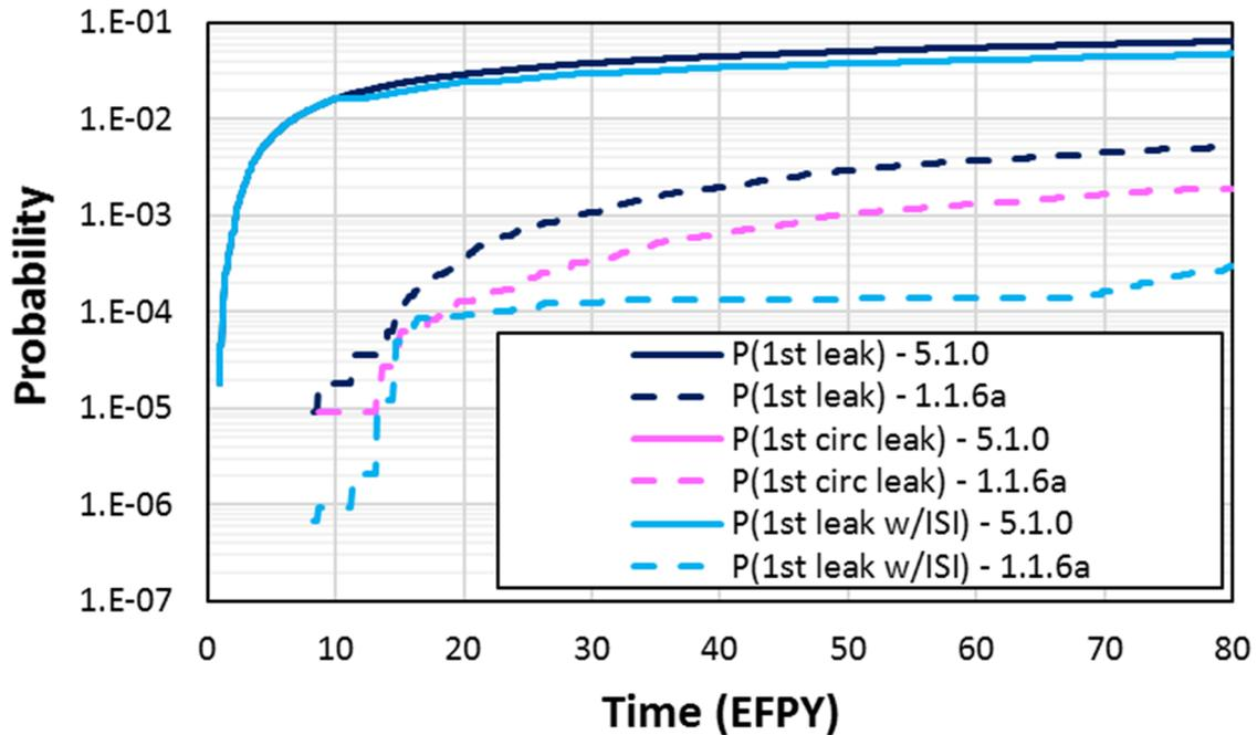
Figure 3-77 Case 5.1.0 time-dependent probabilities of first leak
