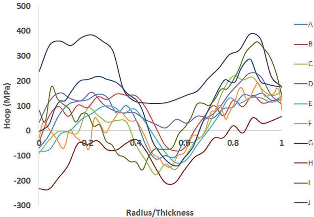
**Figure C-3 Pressurizer surge line nozzle hoop WRS profiles through the weld centerline from 10 modelers**
