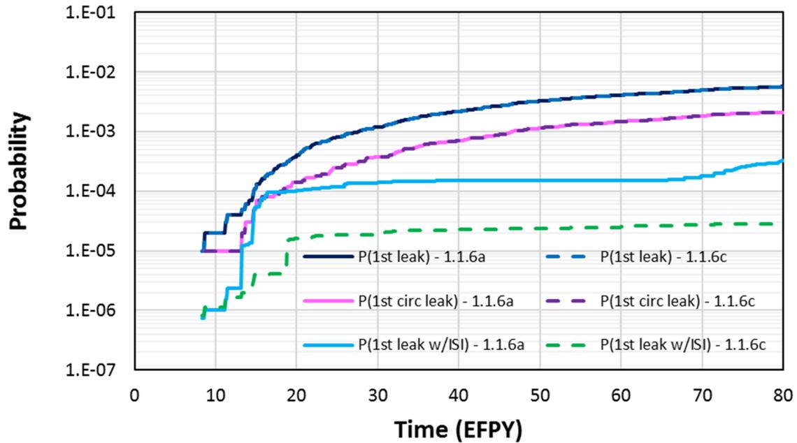
**Figure 3-6 Comparison of Case 1.1.6c time-dependent probabilities of first leak, first circumferential leak, and first leak with ISI with Case 1.1.6a**
