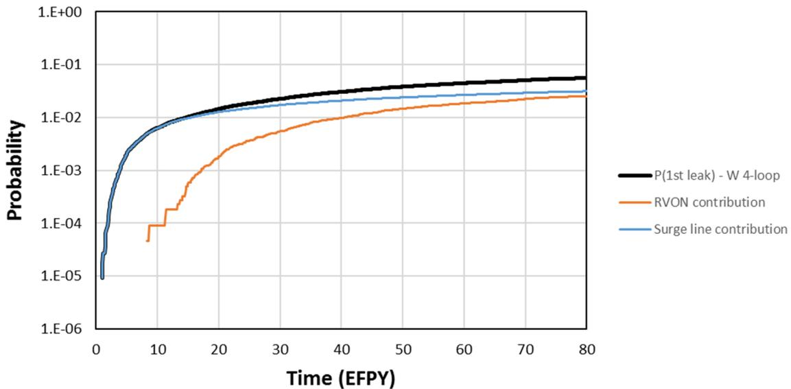
**Figure 4-4 Westinghouse four-loop system probability of first leak and component contributions**
