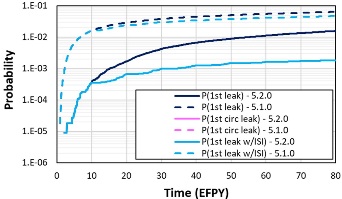
Figure 3-87 Case 5.2.0 time-dependent probabilities of first leak
