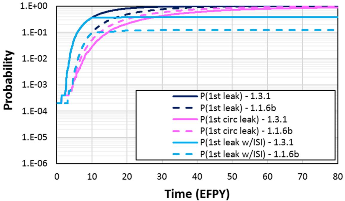
**Figure 3-100 Case 1.3.1 time-dependent probabilities of first leak**
