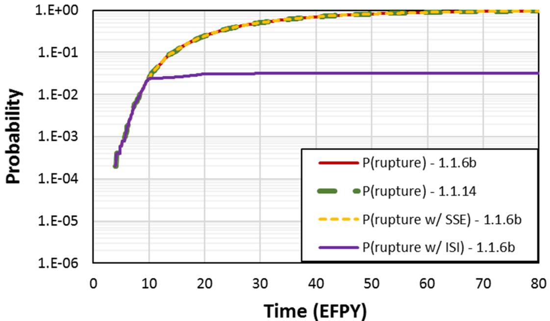
**Figure 3-12 Case 1.1.6b time-dependent probabilities of rupture**
