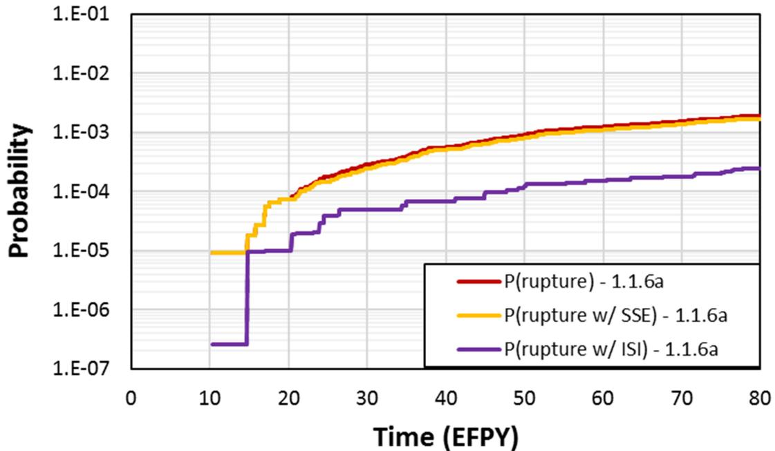
**Figure 3-7 Case 1.1.6a time-dependent probabilities of rupture with a 10-year inspection frequency**
