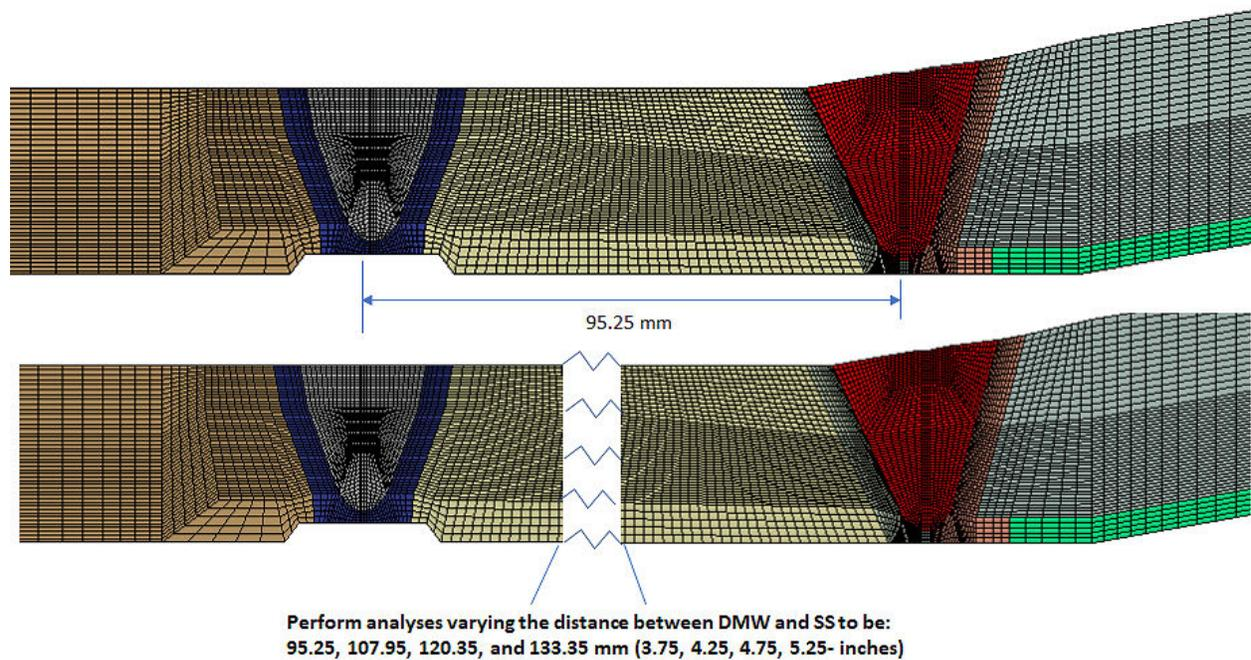
**Figure C-36 FEA mesh for DMW to SS closure weld distance**
