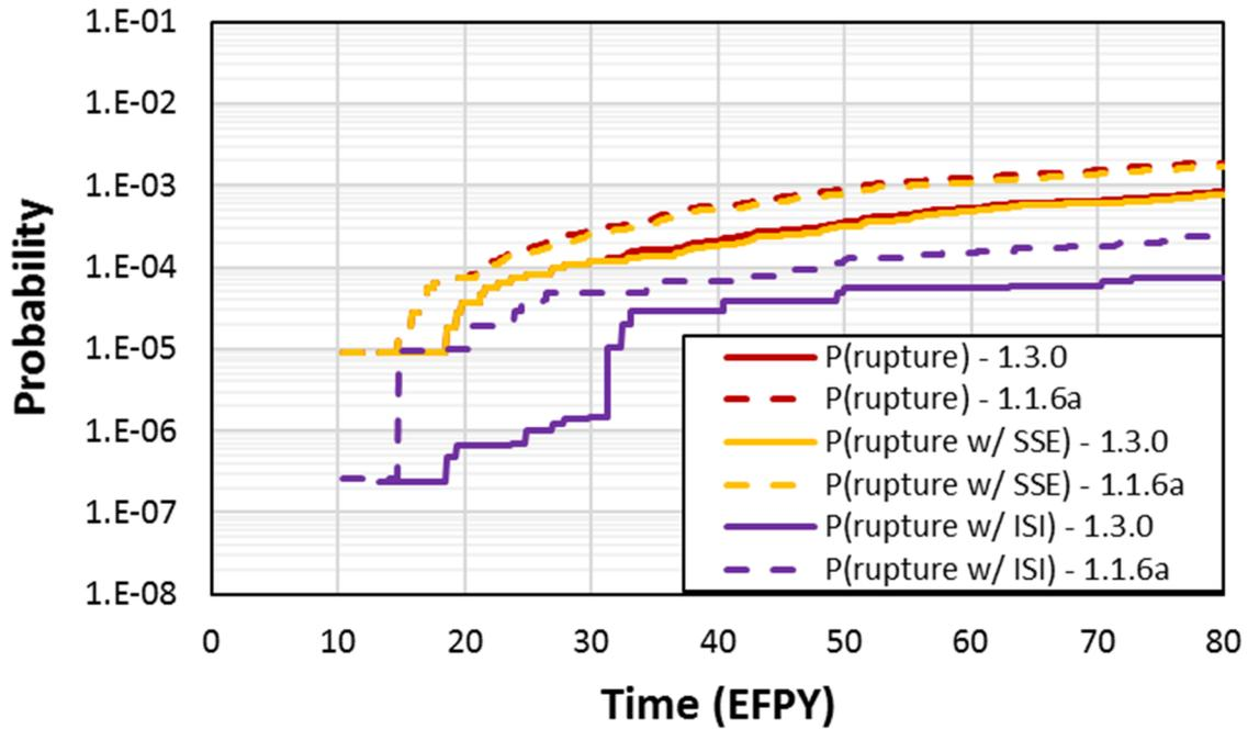
**Figure 3-97 Case 1.3.0 time-dependent probabilities of rupture**
