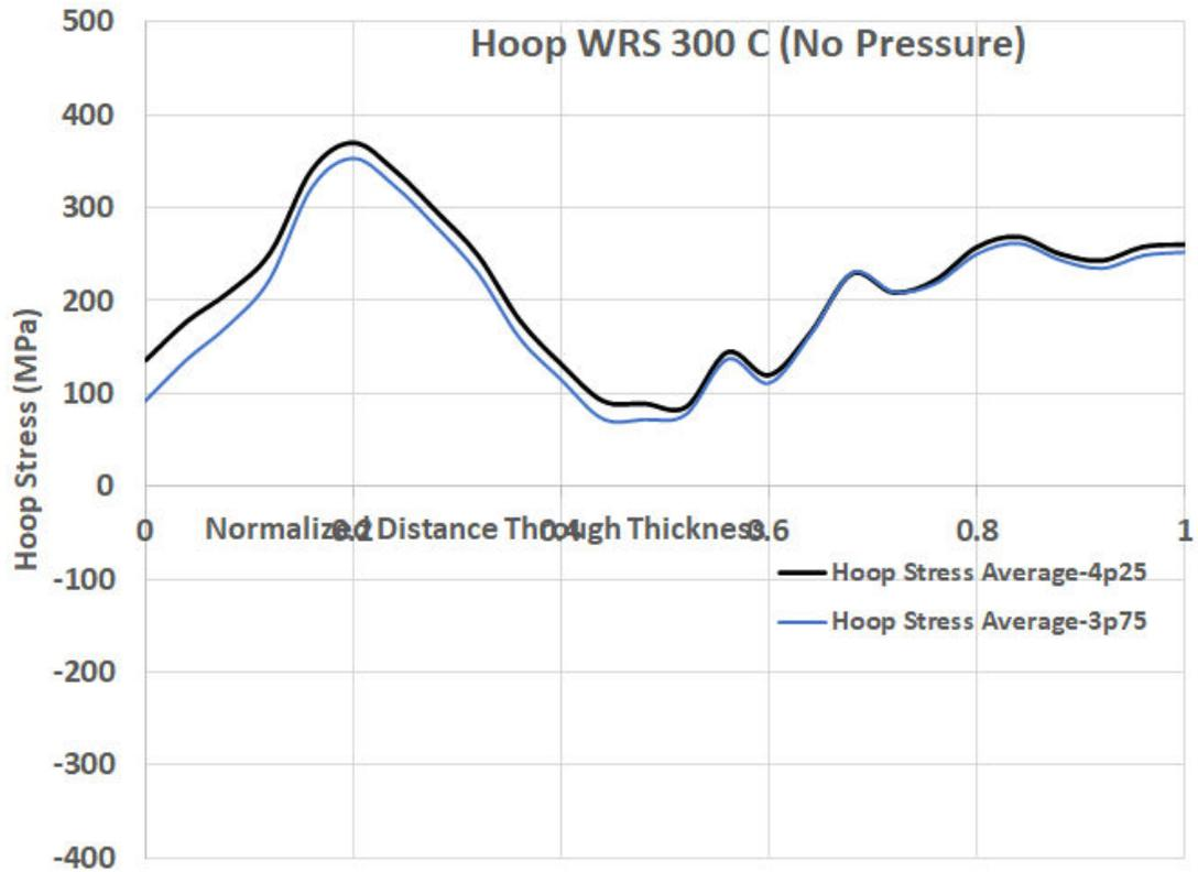
**Figure C-33 CE branch line nozzle hoop WRS profiles for different DMW to SS closure weld distances**
