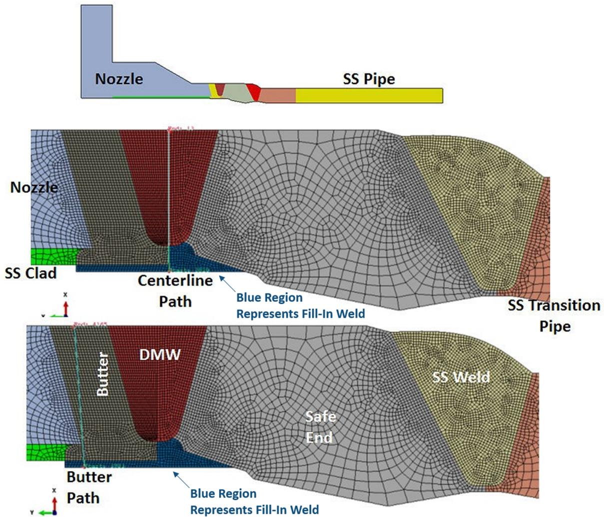
**Figure C-1 FEA model for pressurizer surge line nozzle with fill-in weld used for WRS profile development**
