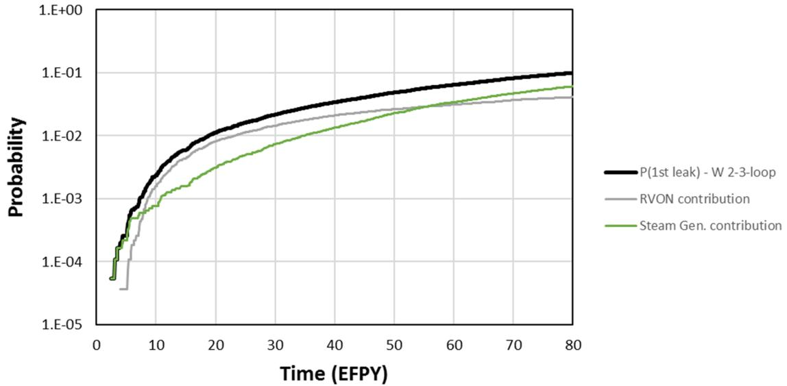
**Figure 4-12 Westinghouse two- and three-loop system probability of first leak and component contributions**
