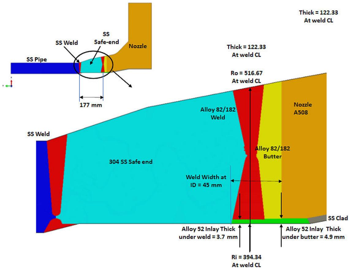
**Figure C-16 Replacement steam generator nozzle geometry, dimensions, and materials**
