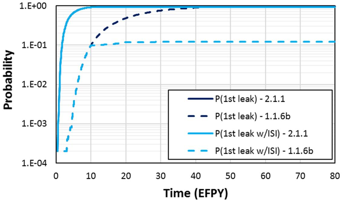
**Figure 3-21 Case 2.1.1 time-dependent probabilities of first leak**
