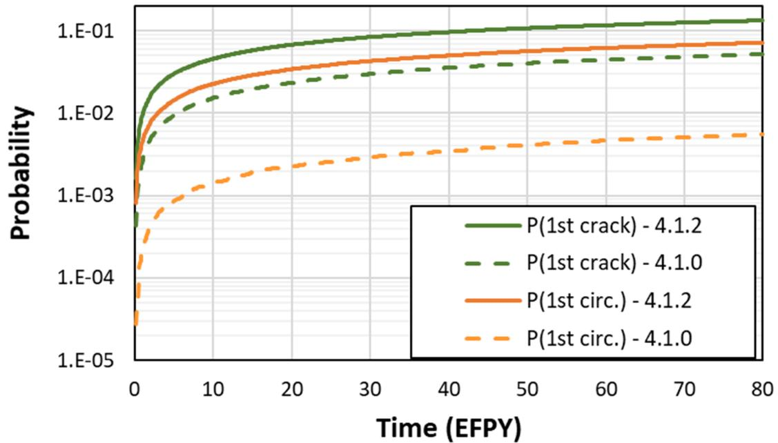
**Figure 3-66 Case 4.1.2 time-dependent probabilities of first crack**
