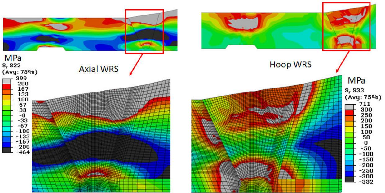
Figure C-28 CE branch line nozzle axial (left) and hoop (right) WRS contour plots generated from FEA at 300°C
