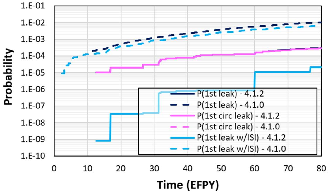
**Figure 3-67 Case 4.1.2 time-dependent probabilities of first leak**
