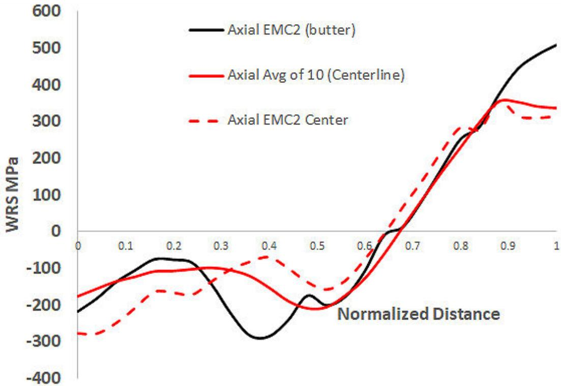
**Figure C-9 Pressurizer surge line nozzle axial WRS profiles through the weld centerline and butter using the average of the isotropic and NLKH solutions**
