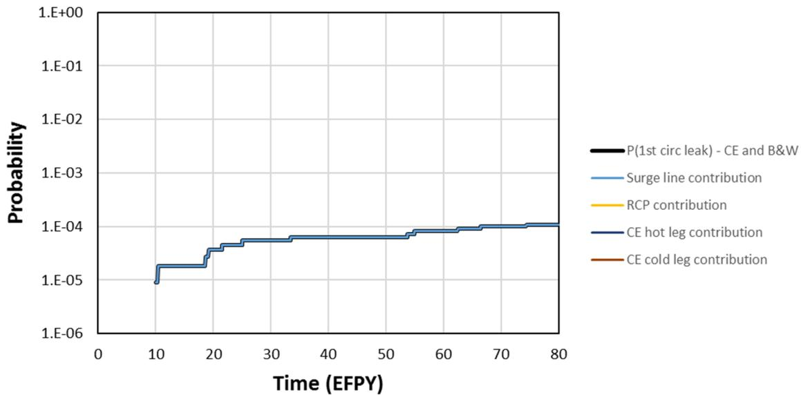
**Figure 4-22 CE and B&W system probability of first circumferential leak and component contributions**
