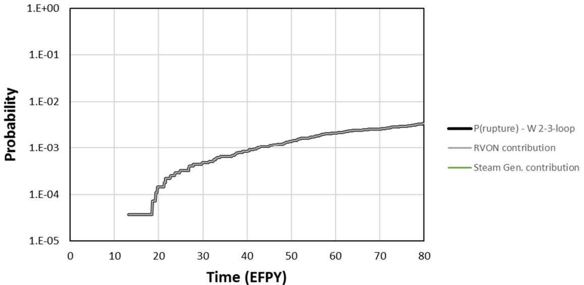
**Figure 4-15 Westinghouse two- and three-loop system probability of rupture and component contributions**
