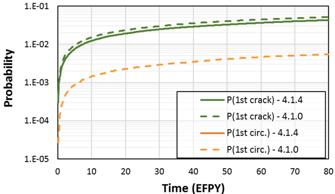
**Figure 3-73 Case 4.1.4 time-dependent probabilities of first crack**
