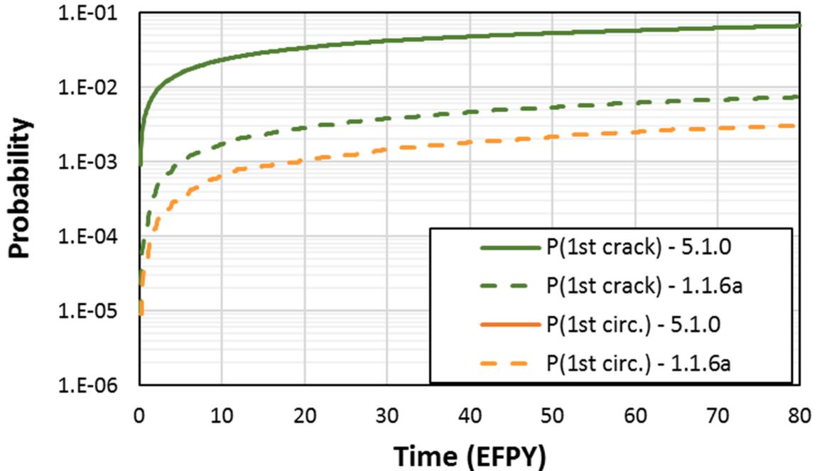
**Figure 3-76 Case 5.1.0 time-dependent probabilities of first crack**
