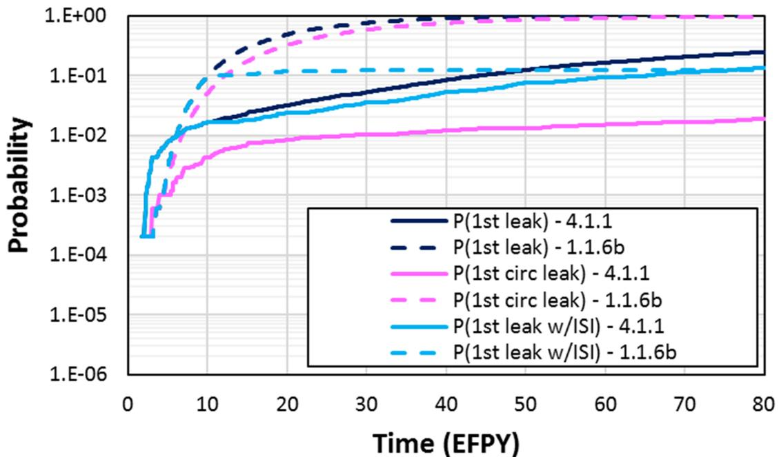
Figure 3-61 Case 4.1.1 time-dependent probabilities of first leak
