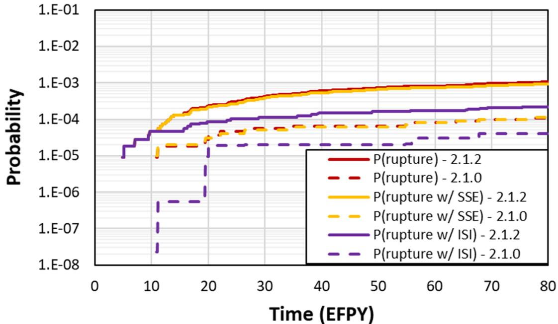
Figure 3-30 Case 2.1.2 time-dependent probabilities of rupture
