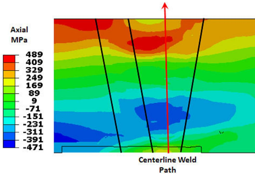
Figure C-41 More severe axial WRS contour plot for the RVON weld
