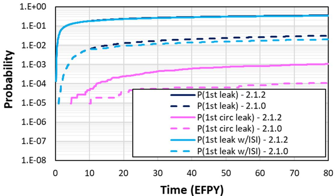
**Figure 3-29 Case 2.1.2 time-dependent probabilities of first leak**
