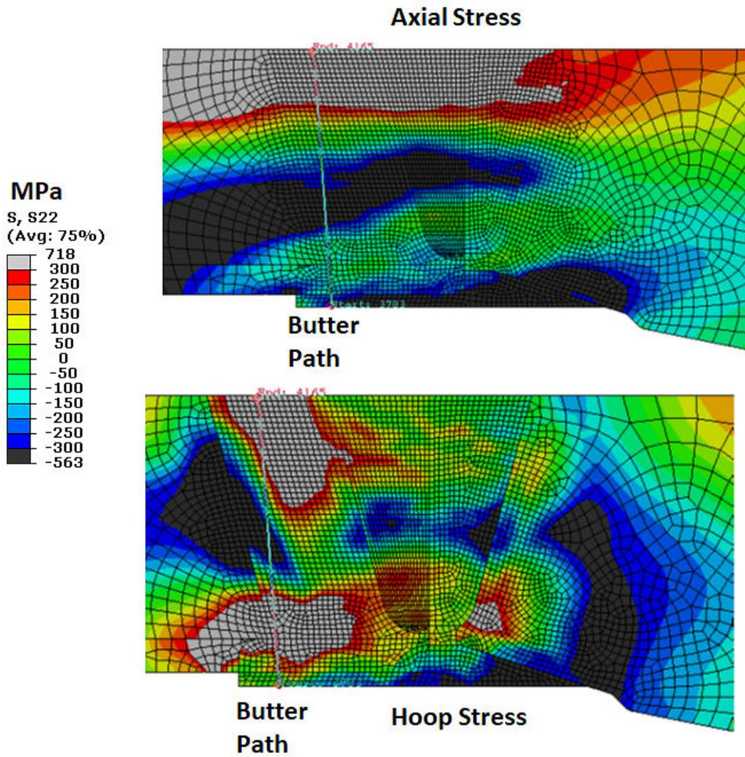
Figure C-8 Pressurizer surge line nozzle axial and hoop WRS contour plots generated from FEA with isotropic hardening law
