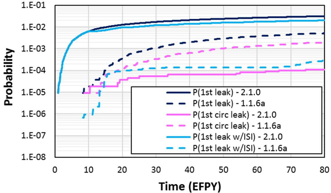
**Figure 3-17 Case 2.1.0 time-dependent probabilities of first leak**
