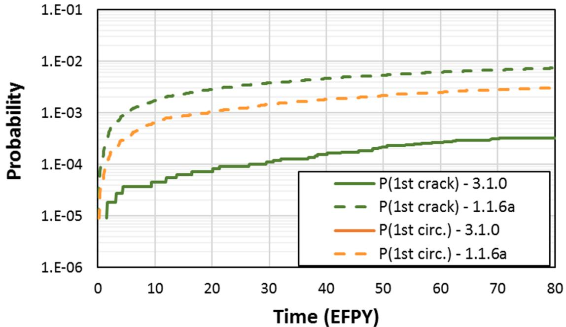
Figure 3-50 Case 3.1.0 time-dependent probabilities of first crack
