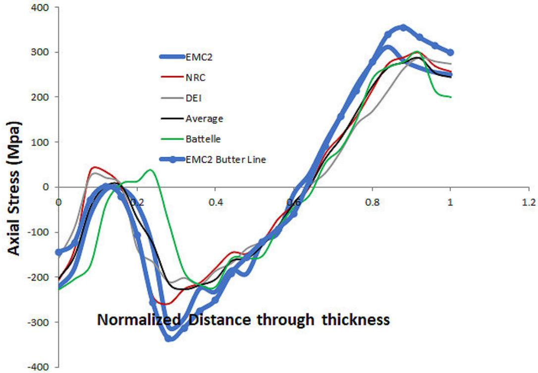
Figure C-13 RCP nozzle axial WRS profiles through the weld centerline and butter from four modelers
