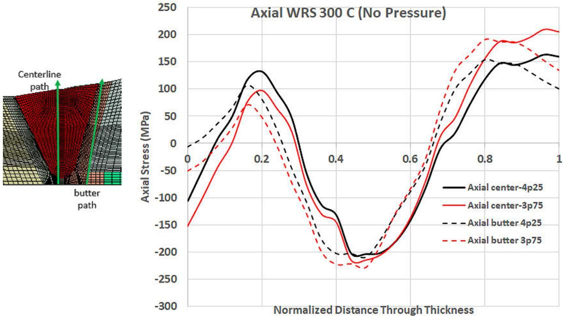
**Figure C-34 Comparison of CE branch line nozzle axial WRS profiles through weld centerline and butter**
