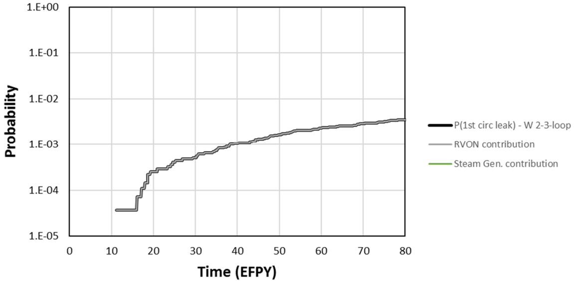
**Figure 4-14 Westinghouse two- and three-loop system probability of first circumferential leak and component contributions**
