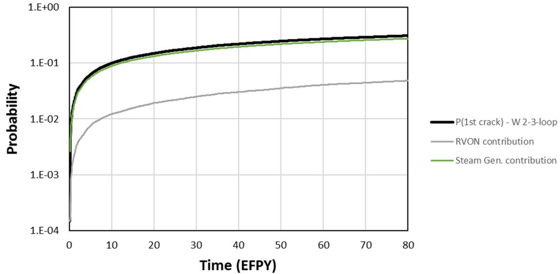
**Figure 4-10 Westinghouse two- and three-loop system probability of first crack and component contributions**
