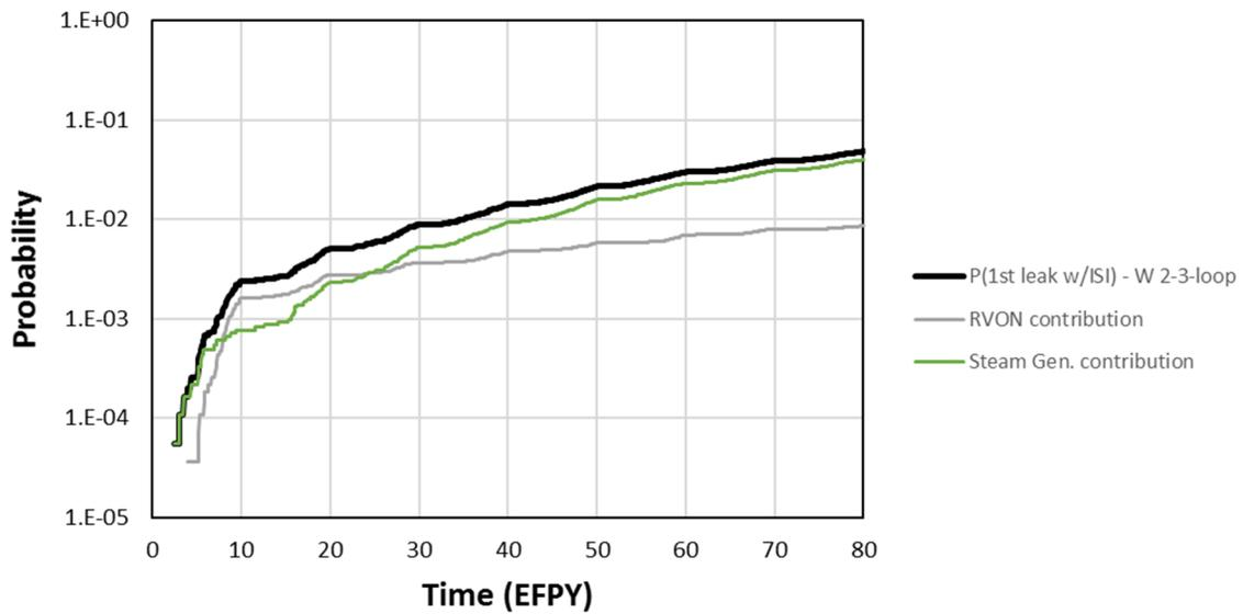
**Figure 4-13 Westinghouse two- and three-loop system probability of first leak with a 10-year inspection frequency and component contributions**
