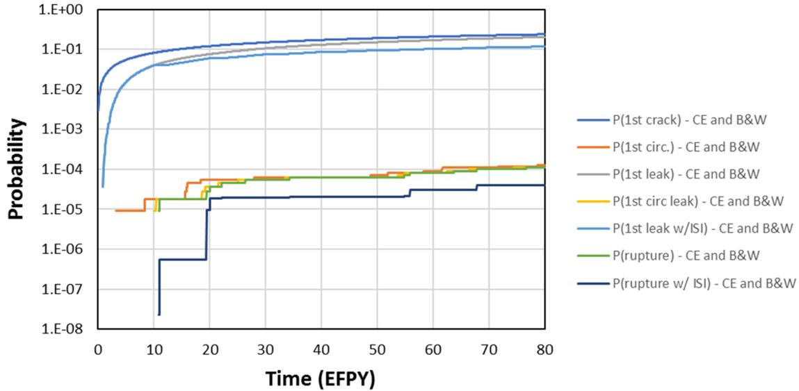
**Figure 4-17 CE and B&W time-dependent probabilities**
