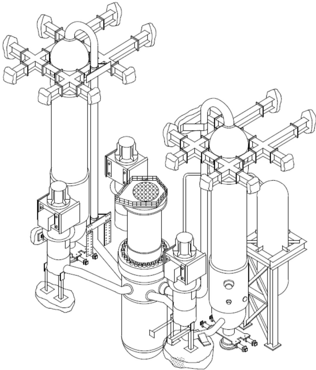
**Figure 2-3** Typical B&W PWR nuclear steam supply system piping arrangement
