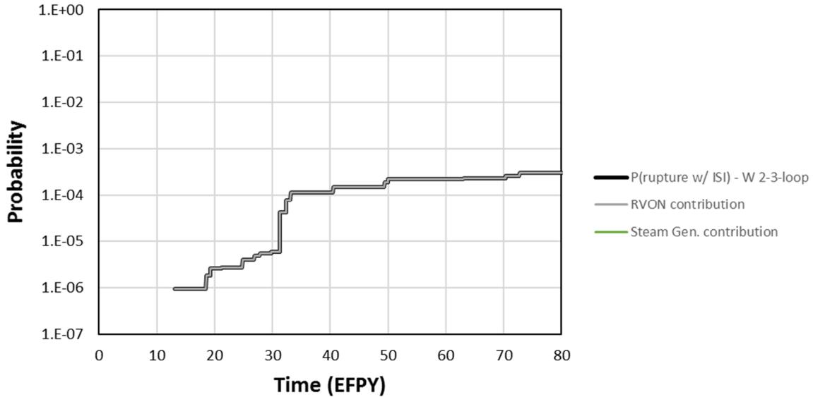
**Figure 4-16 Westinghouse two- and three-loop system probability of rupture with a 10-year inspection frequency and component contributions**
