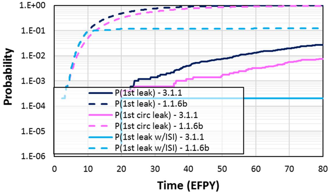
**Figure 3-53 Case 3.1.1 time-dependent probabilities of first leak**
