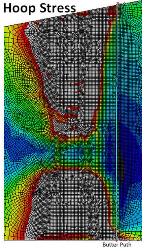
Figure C-21 Replacement steam generator nozzle hoop WRS contour plot generated from FEA
