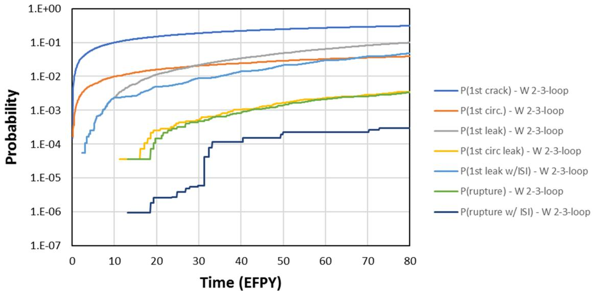
**Figure 4-9 Westinghouse two- and three-loop time-dependent probabilities**
