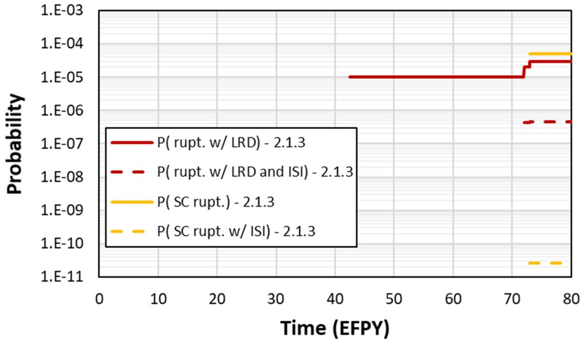
**Figure 3-32 Case 2.1.3 time-dependent probabilities of rupture with leak rate detection and ISI**
