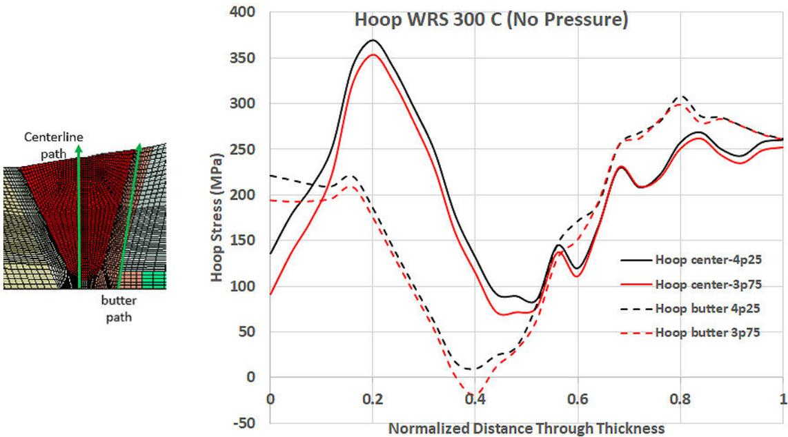
**Figure C-35 Comparison of CE branch line nozzle hoop WRS profiles through the weld centerline and butter**
