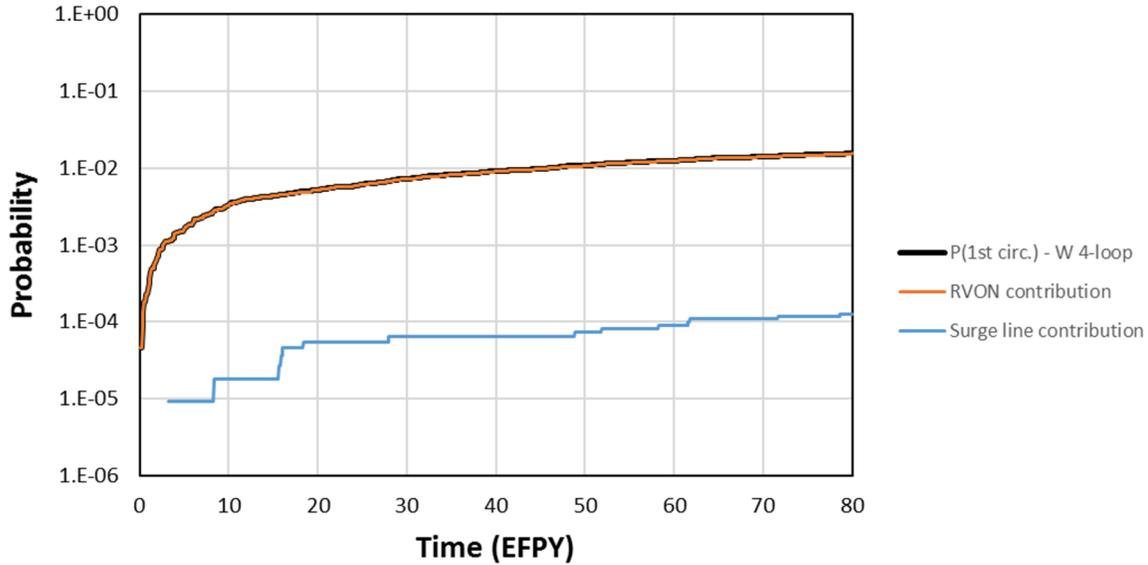
**Figure 4-3 Westinghouse four-loop system probability of first circumferential crack and component contributions**
