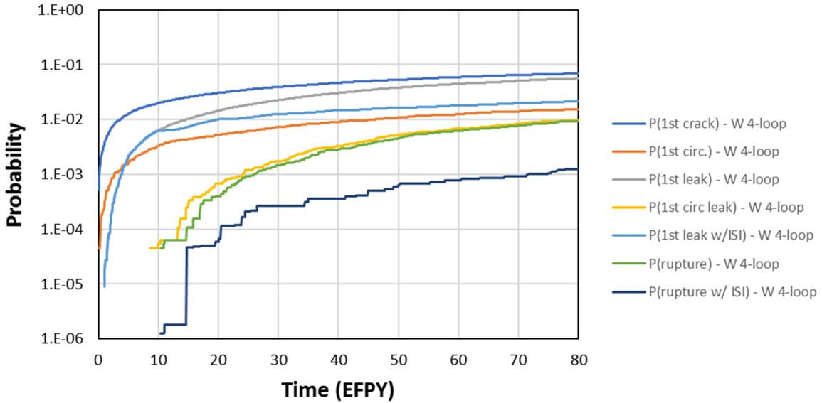
**Figure 4-1 Bounding Westinghouse four-loop time-dependent probabilities**
