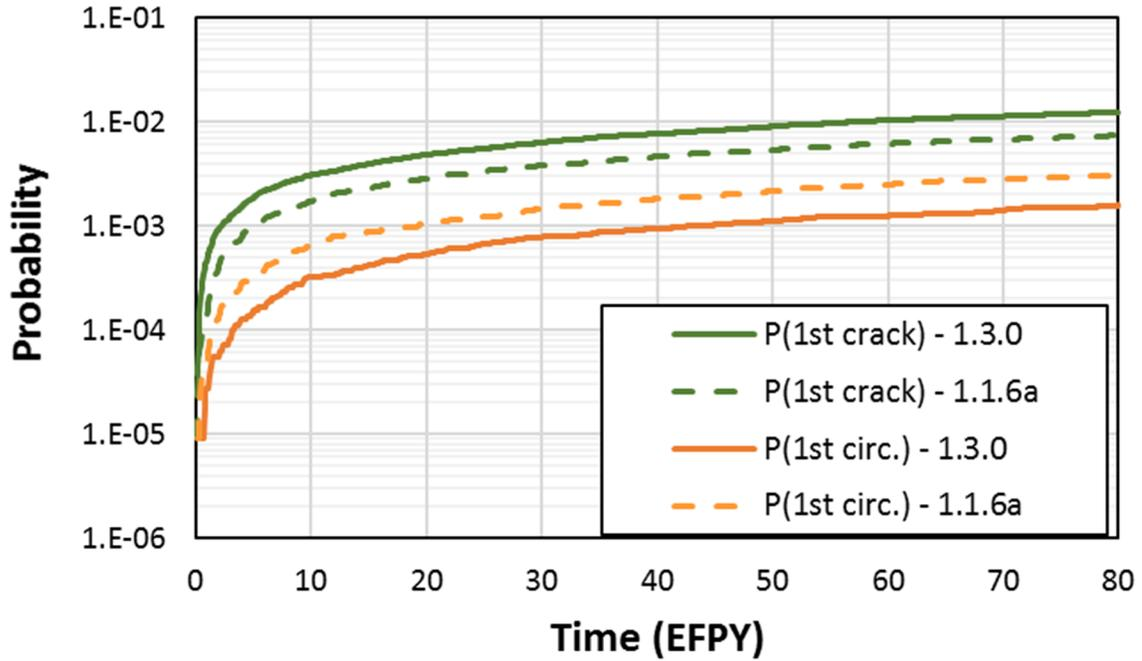
**Figure 3-95 Case 1.3.0 time-dependent probabilities of first crack**
