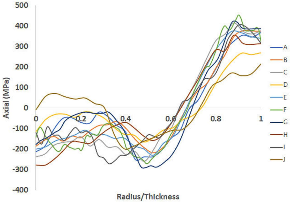
**Figure C-2 Pressurizer surge line nozzle axial WRS profiles through the weld centerline from 10 modelers**
