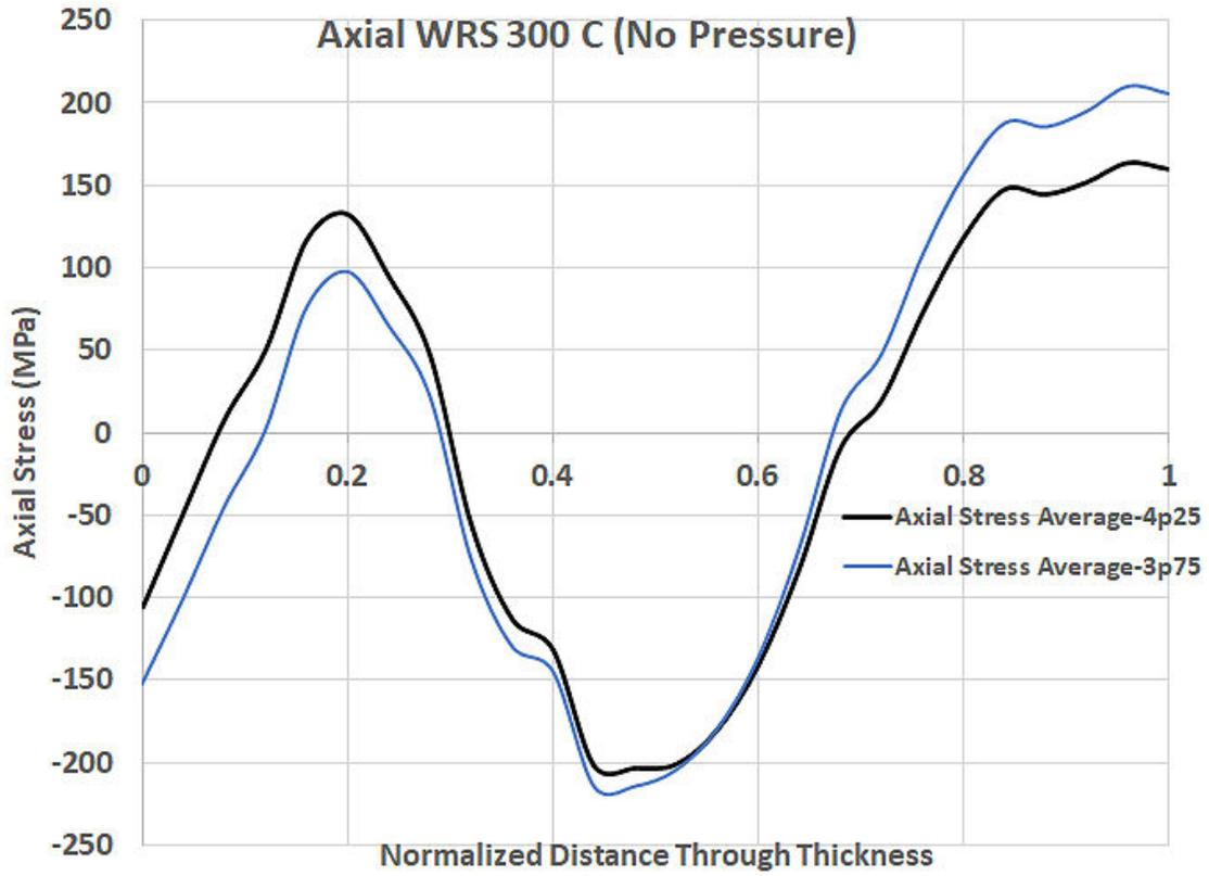
Figure C-32 CE branch line nozzle axial WRS profiles for different DMW to SS closure weld distances
