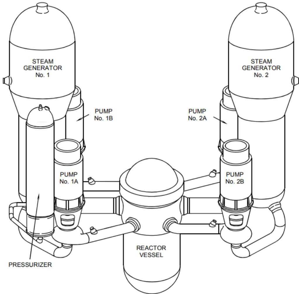
**Figure 2-2** Typical CE PWR nuclear steam supply system piping arrangement
