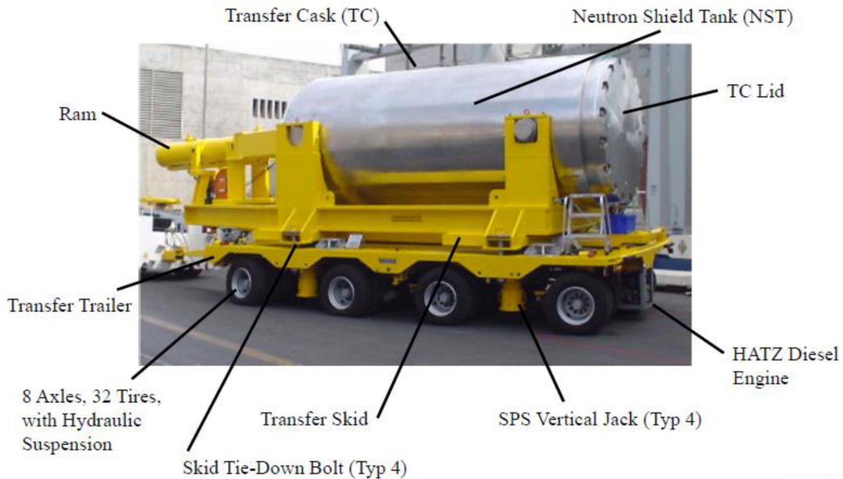
Figure 4-3 Assembled Transfer Trailer
