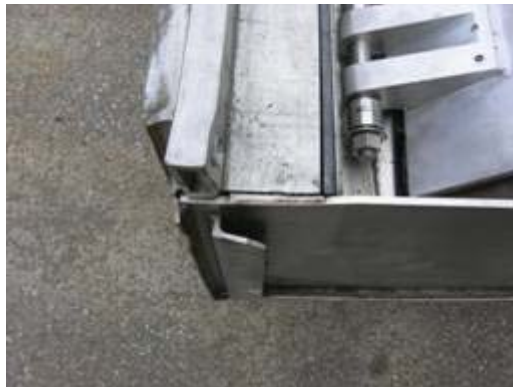
Figure 2-59 - Cracked bottom weld
