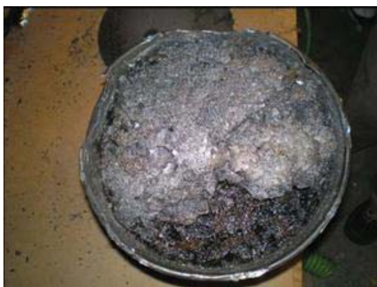
Figure 3-30 – Foam char under ceramic fiber paper
