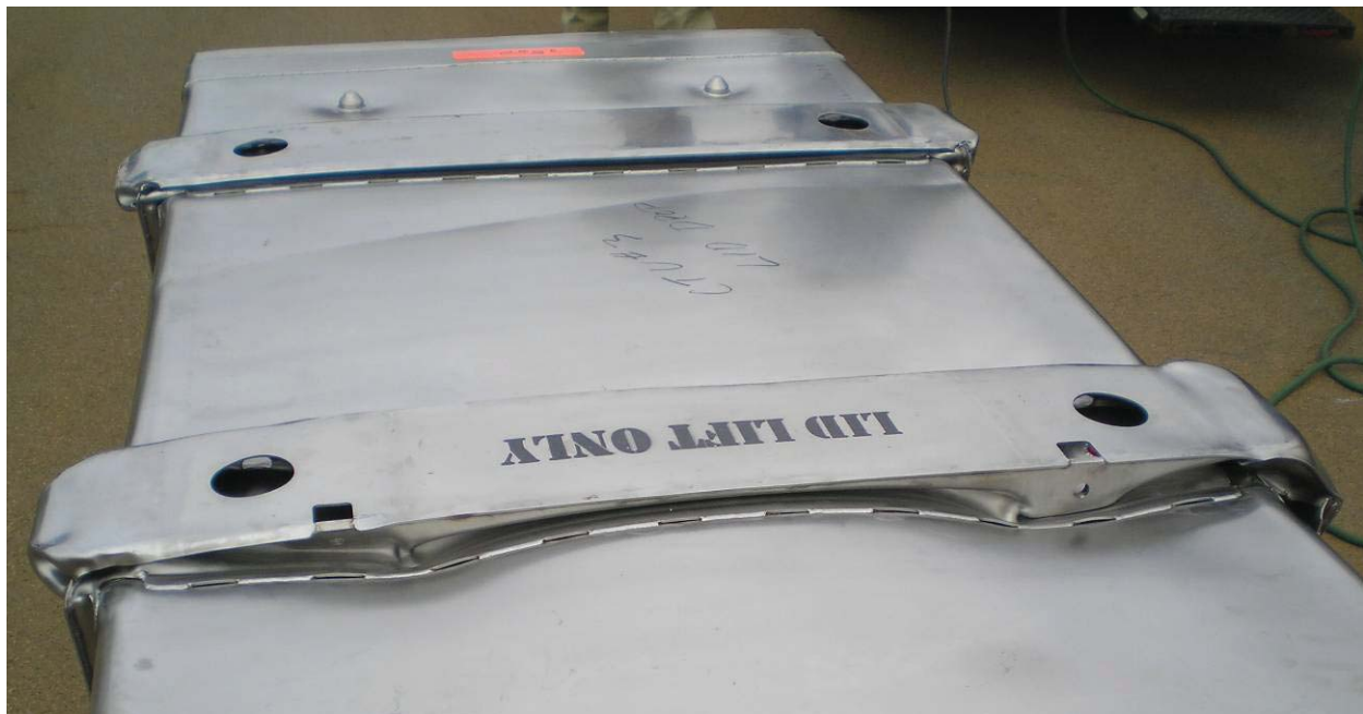
Figure 2-13 – Shell Deformation at Lid Lifting Locations
