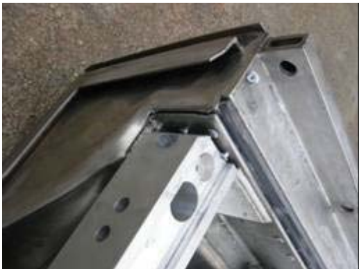
Figure 2-58 - Cracked top weld
