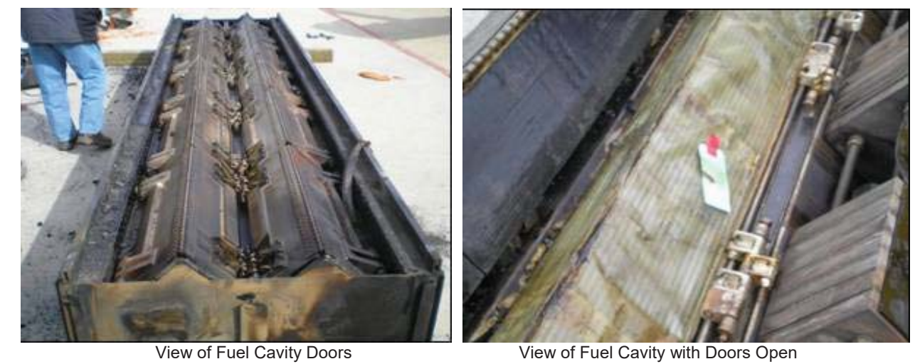
Figure 3-17 – MAP CTU 3 after Fire Test: Lid Assembly Removed
