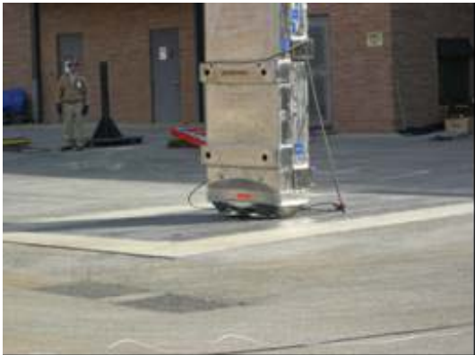
Figure 2-35 - CTU2 immediately after drop
