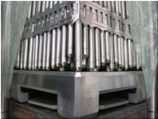
Figure 2-62 - Slight rod movement (bottom)
