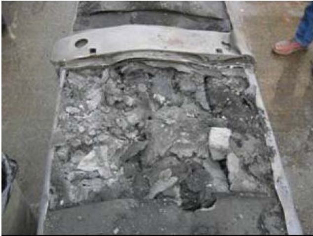
Foam Under Ceramic Fiber Paper Intumesced Filling Voids
