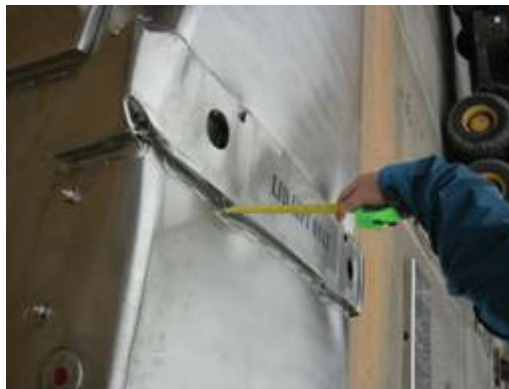
Figure 2-74 - CTU3 lid deformation measurement
