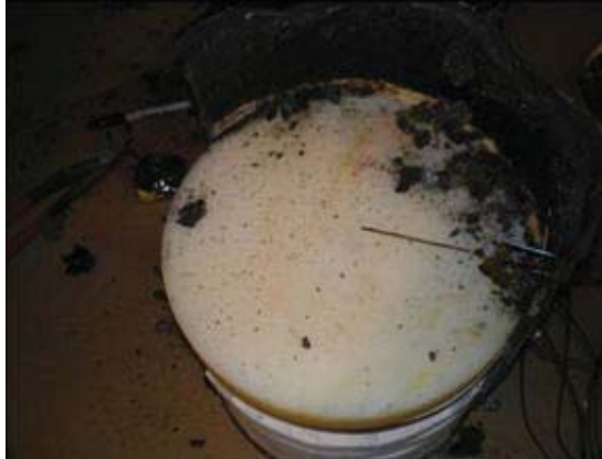
Figure 3-32 – Moderator surface, flame side
