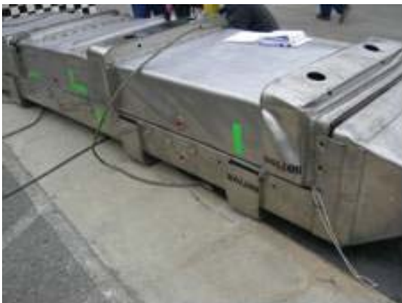
Figure 2-47 - CTU1 inverted for puncture test
