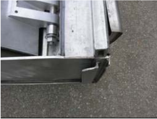
Figure 2-60 - No damage to bottom closure
