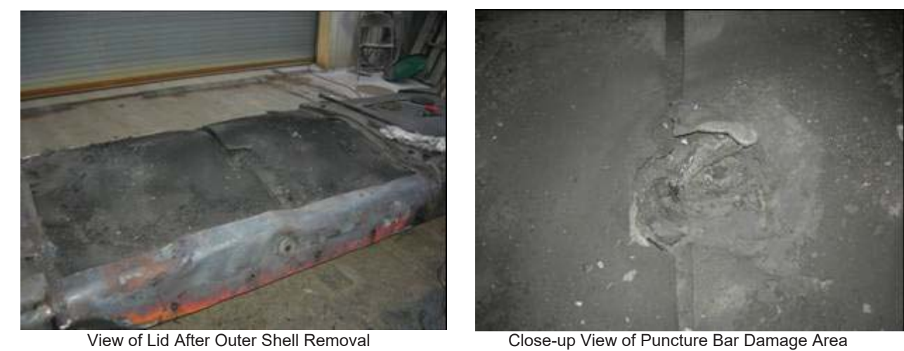
Figure 3-18 – Dissection of CTU 3 after Fire Test: Lid Outer Shell Removal
