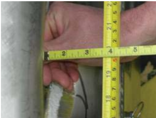
Figure 2-78 - CTU3 puncture depth measurement
