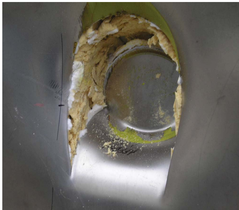
Figure 2-14 – Puncture Damage for Test CP1
