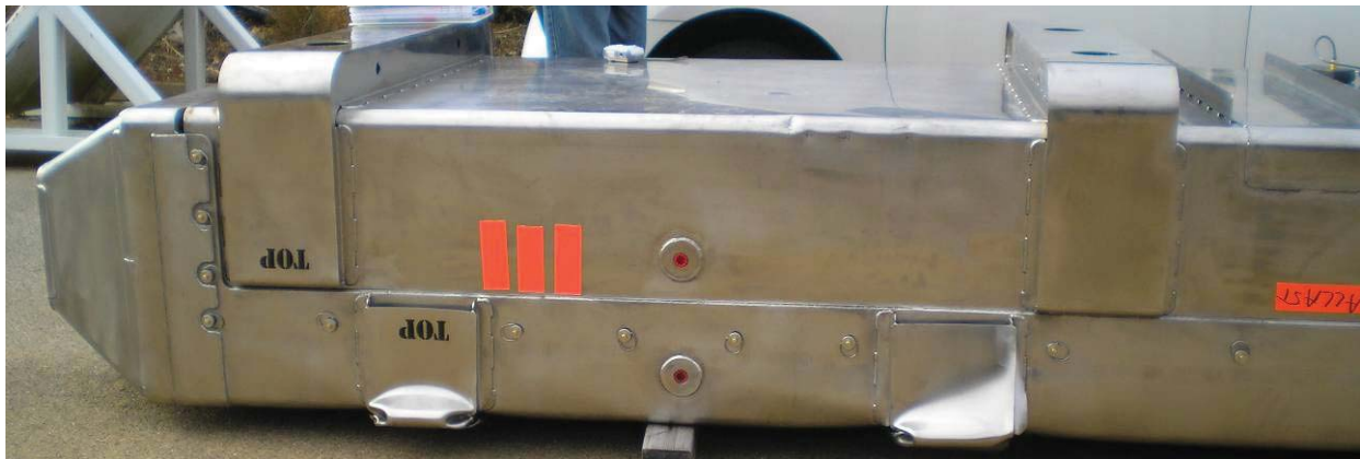
Figure 2-11 – Top End Stiffener Damage
