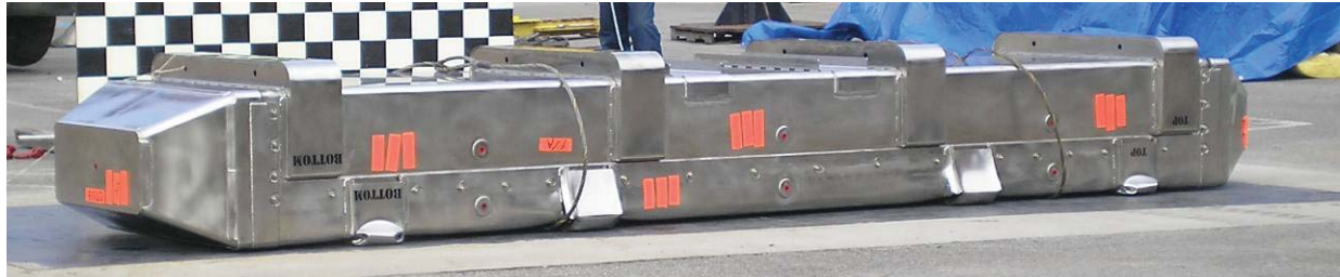
Figure 2-10 – Global Package Damage after Test CD5
