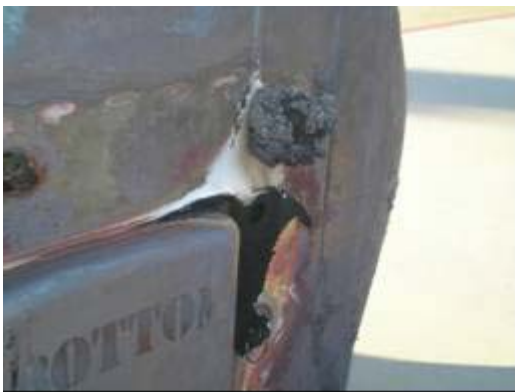
Figure 2-87 - Foam char in lock pin area
