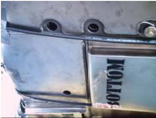
Figure 2-81 - CTU3 lock pin removal opposite side
