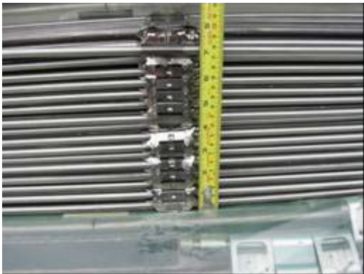
Figure 2-65 - Mid-span lattice compression
