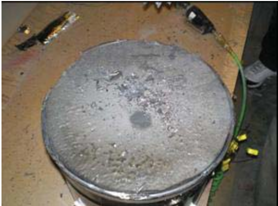
Figure 3-27 – Intact ceramic fiber following test
