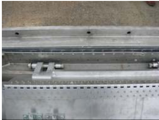
Figure 2-55 - Location of broken rivets
