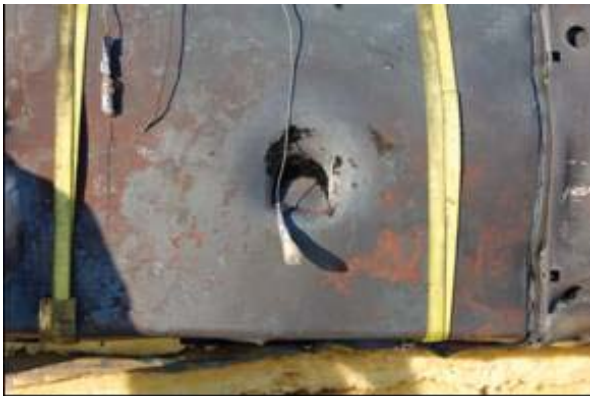
Figure 2-83 - Puncture area after thermal test
