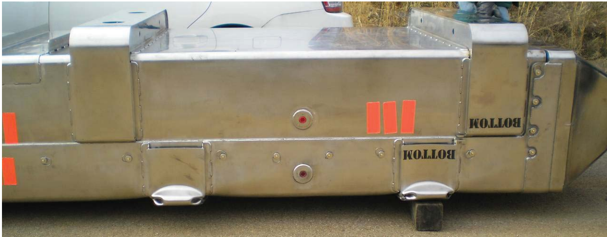
Figure 2-12 – Bottom End Stiffener Damage
