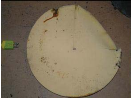
Figure 3-29 – Remaining 6 lb/ft 3 foam, backside
