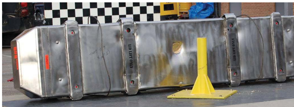
Figure 2-18 – Puncture Damage for Test CP3
