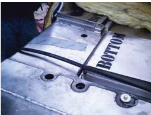
Figure 2-80 - CTU3 lock pin removal
