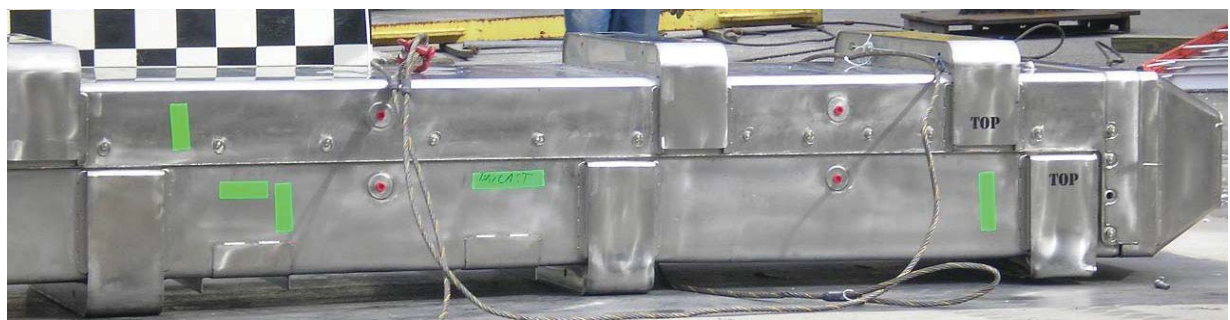
Figure 2-3 – Secondary Impact Stiffener Damage
