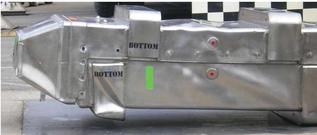
Figure 2-8 – Primary Impact End Damage
