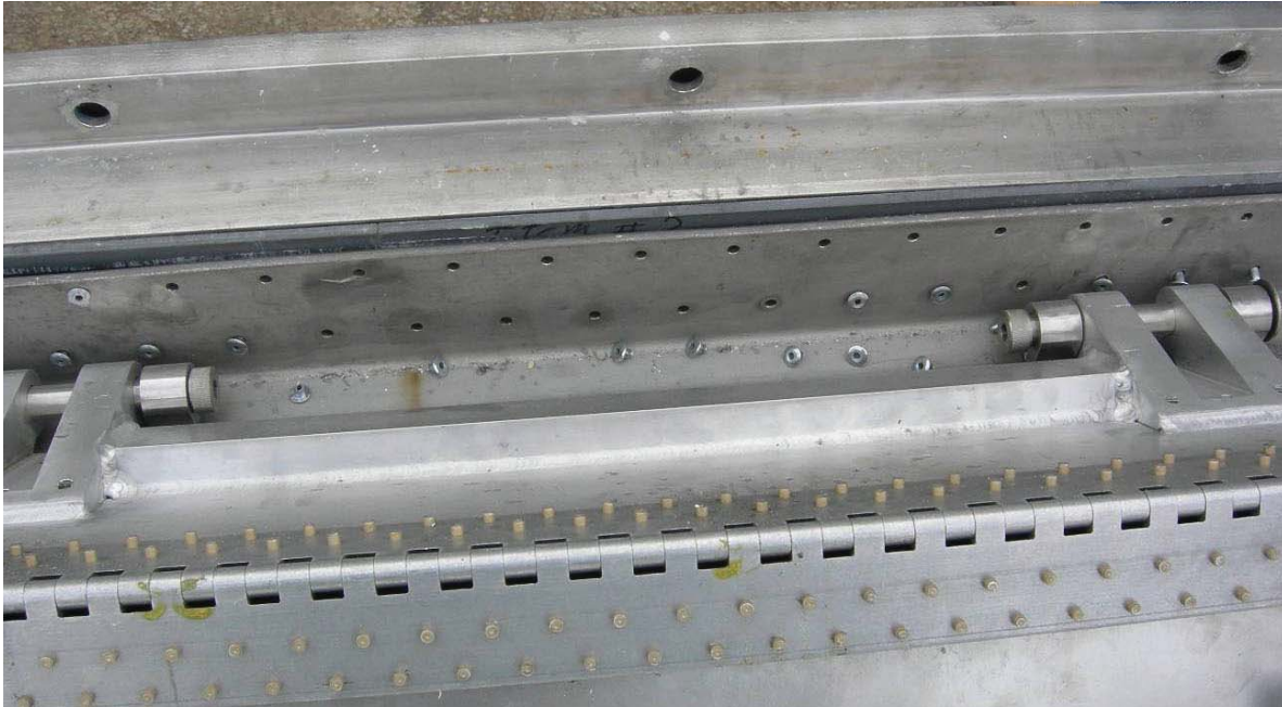
Figure 2-22 – Sheared Base Assembly Rivets
