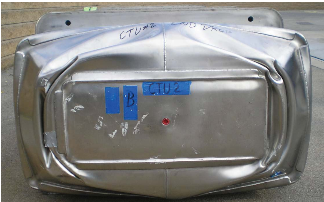
Figure 2-5 – Front View of Impact Limiter Damage
