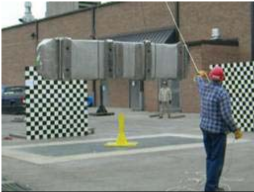
Figure 2-52 - CTU1 side puncture test
