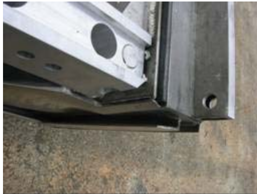
Figure 2-57 - Cracked top weld
