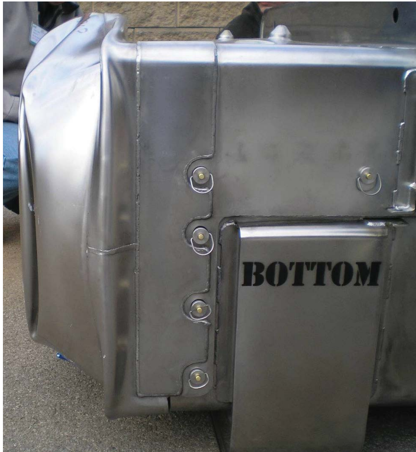
Figure 2-6 – Side View of Impact Limiter Damage
