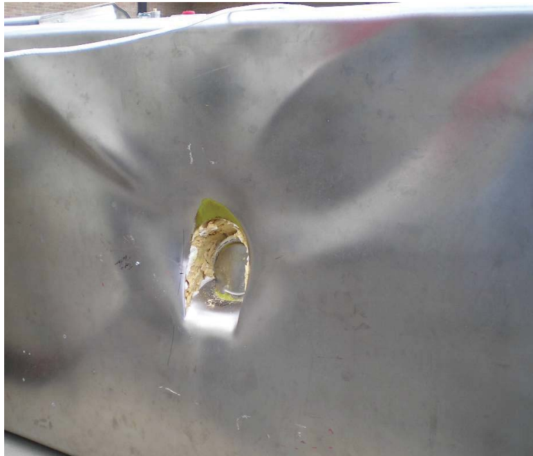
Figure 2-14 – Puncture Damage for Test CP1
