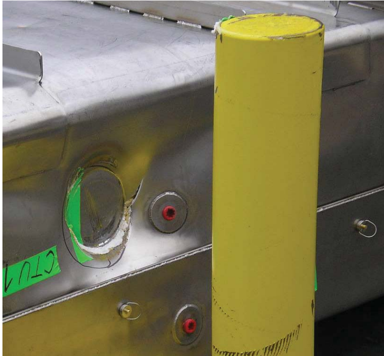
Figure 2-16 – Puncture Damage for Test CP2
