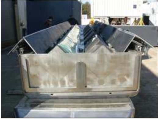
Figure 2-40 - Base interior after impact
