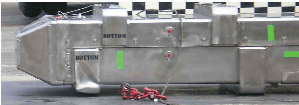
Figure 2-2 – Primary Impact Stiffener Damage
