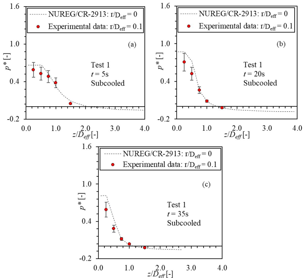
Figure 3-52 Comparison between NUREG/CR-2913 and Experimental Data in Marviken Tests of Test 1 for Static Pressure: (a) 5 s, (b) 20 s, and (c) 35 s. Error Bar:  $\pm 20\%$ . Comparisons are Obtained from NUREG/CR-2913
