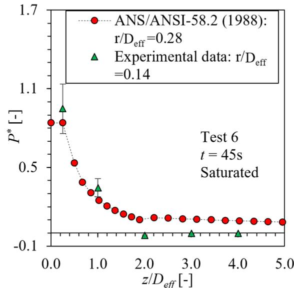
Figure 3-40 Pressure Profiles at Different Axial Locations at 45 s in Test 6. Error Bar:  $\pm 20\%$
