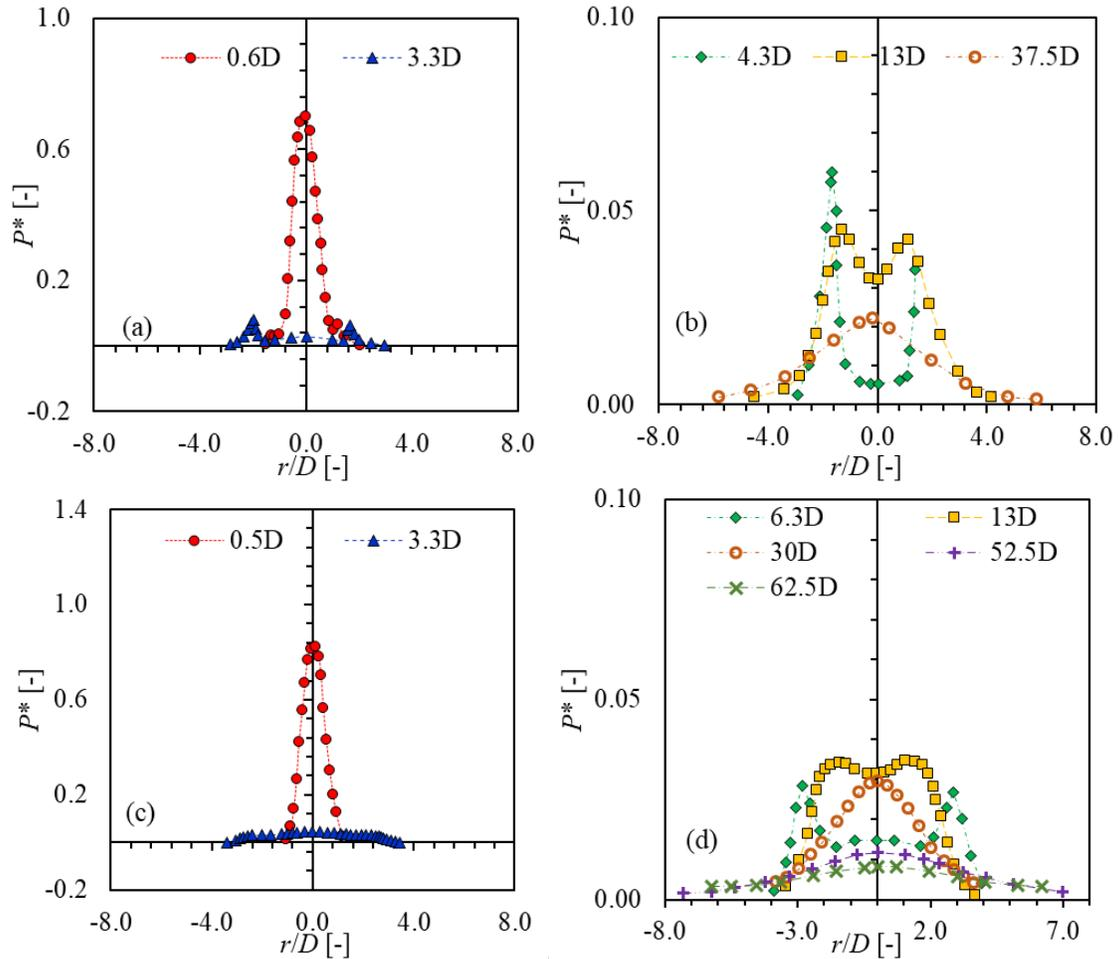
Figure 3-17 Stagnation Pressure Downstream of the Break Plane at Different Axial Locations in Masuda et al. (1981): (a) and (b) Free Steam Jets, (c) and (d) Impinging Steam Jets ( $P_0 = 4.02$  MPa,  $D = 10$  mm)
