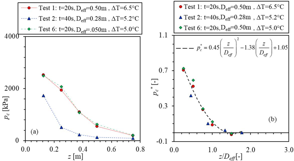
Figure 3-26 Static Pressure Profiles at the Center of Free Subcooled Water Jets ( $\Delta T \sim 5^\circ C$ ) as a Function of Axial Distance. The Best Fitting Line in Figure (b) is Given by Equation (3-10)
