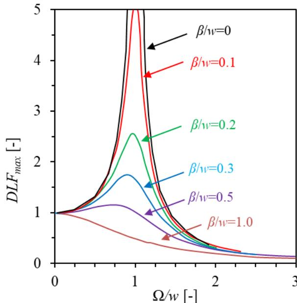
Figure 2-3 Dynamic Load Factor (DLF) with a Sinusoidally Varying Load (Biggs, 1964)
