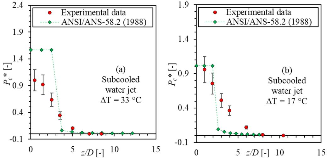
Figure 3-50 Comparison between Standard Model Calculation (ANSI/ANS-58.2, 1988) and Experimental Data of Free Subcooled Water Jets in Kawanishi et al. (1986). Error Bar:  $\pm 20\%$
