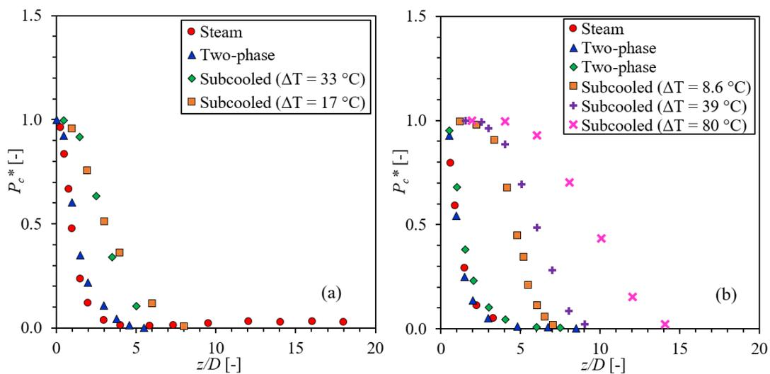
Figure 3-18 The Stagnation Pressure at the Center of Target Plate Downstream of the Break Plane at Different Axial Locations: (a) Free Jets and (b) Impinging Jets in Kawanishi et al. (1986). ( $P_0 = 4.02$  MPa,  $D = 5$  mm)
