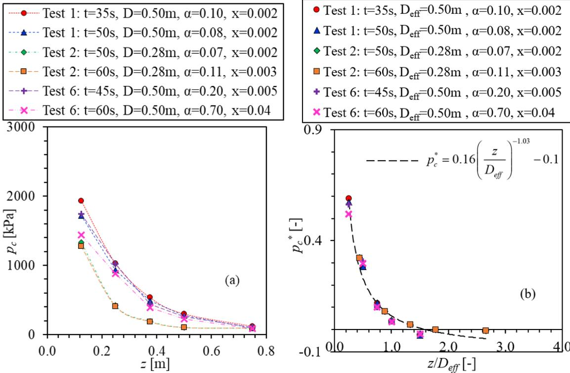
Figure 3-23 Static Pressure Profiles at the Center of Free Saturated Water Jets as a Function of Axial Distance. The Best Fitting Line in Figure (b) is Given by Equation (3-7)
