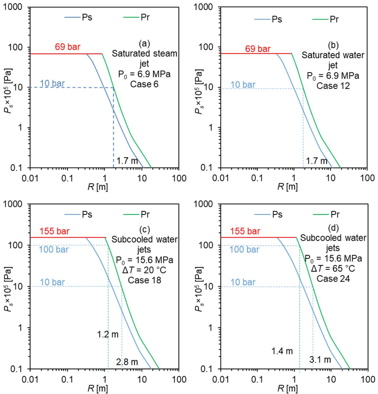
Figure 4-11 Calculated Static Overpressure ( $P_s$ ) and Reflected Pressure ( $P_r$ ) for (a) Saturated Steam Jet Case 6, (b) Saturated Water Jet Case 12, (c) Subcooled Water Jet Case 18, and (d) Subcooled Water Jet Case 24
