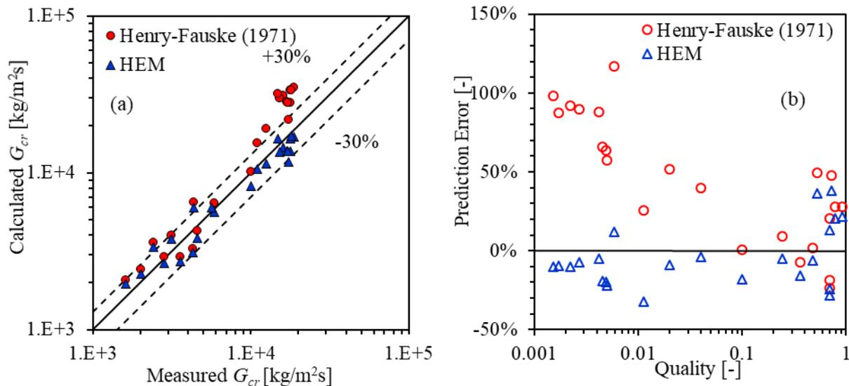
Figure 3-61 Homogeneous Models: (a) Comparison between Calculated  $G_{cr}$  and Measured  $G_{cr}$  in Marviken Tests for Saturated Water/Two-phase Jets and (b) Prediction Error as a Function of the Quality
