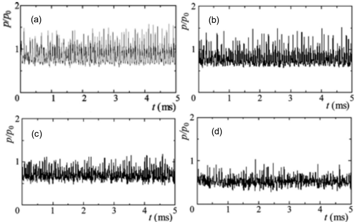
Figure 4-18 Time History of Pressure at the Center of Target for Dry Air Jets: (a)  $S_o = 0$  (Dry Air), (b)  $S_o = 0.4$ , (c)  $S_o = 0.6$ , and (d)  $S_o = 0.8$  (Alam et al., 2010). Nozzle Size: 12.7 mm
