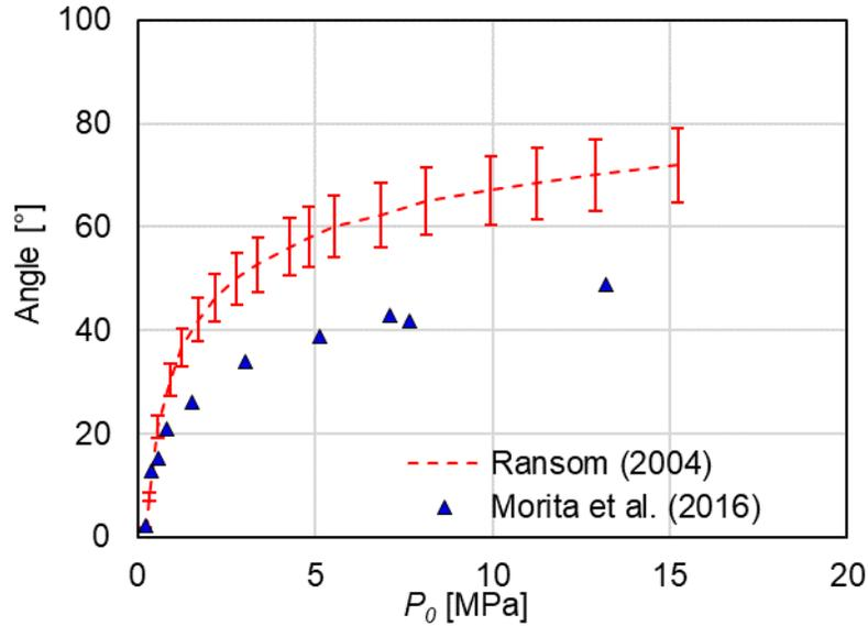
Figure 4-15 Comparison on Prandtl-Meyer Angle between Ransom (2004) and Morita et al. (2016)
