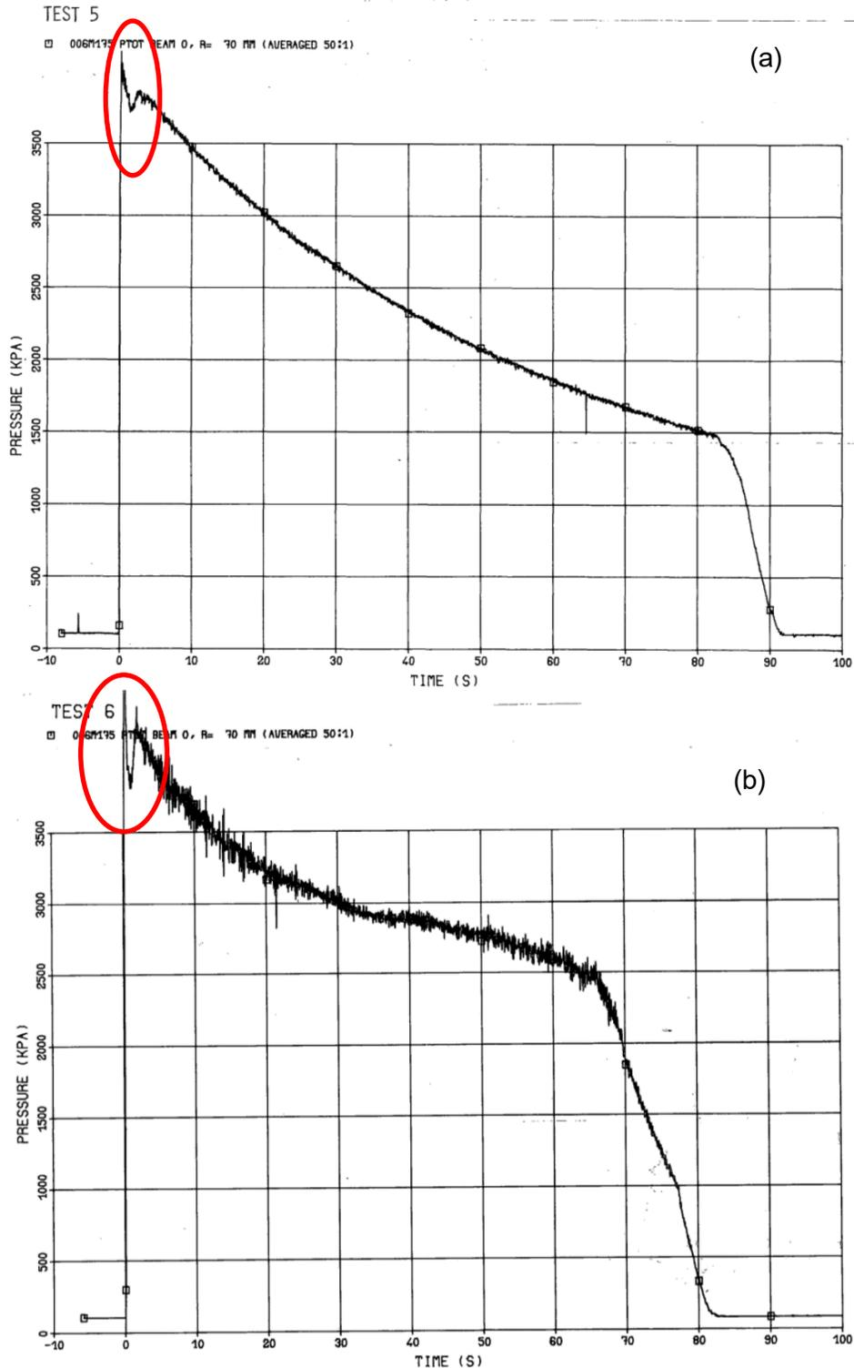
Figure 4-9 Stagnation Pressure near the Center of the Jet Measured at Different Axial Locations for (a) Test 5 Free Steam Jet ( $z/D_{eff} = 0.44$ ) and (b) Test 6 ( $z/D_{eff} = 0.44$ ) of Marviken Tests (Marklund, 1985a). Initial Vessel Stagnation Pressure: 5.0 MPa
