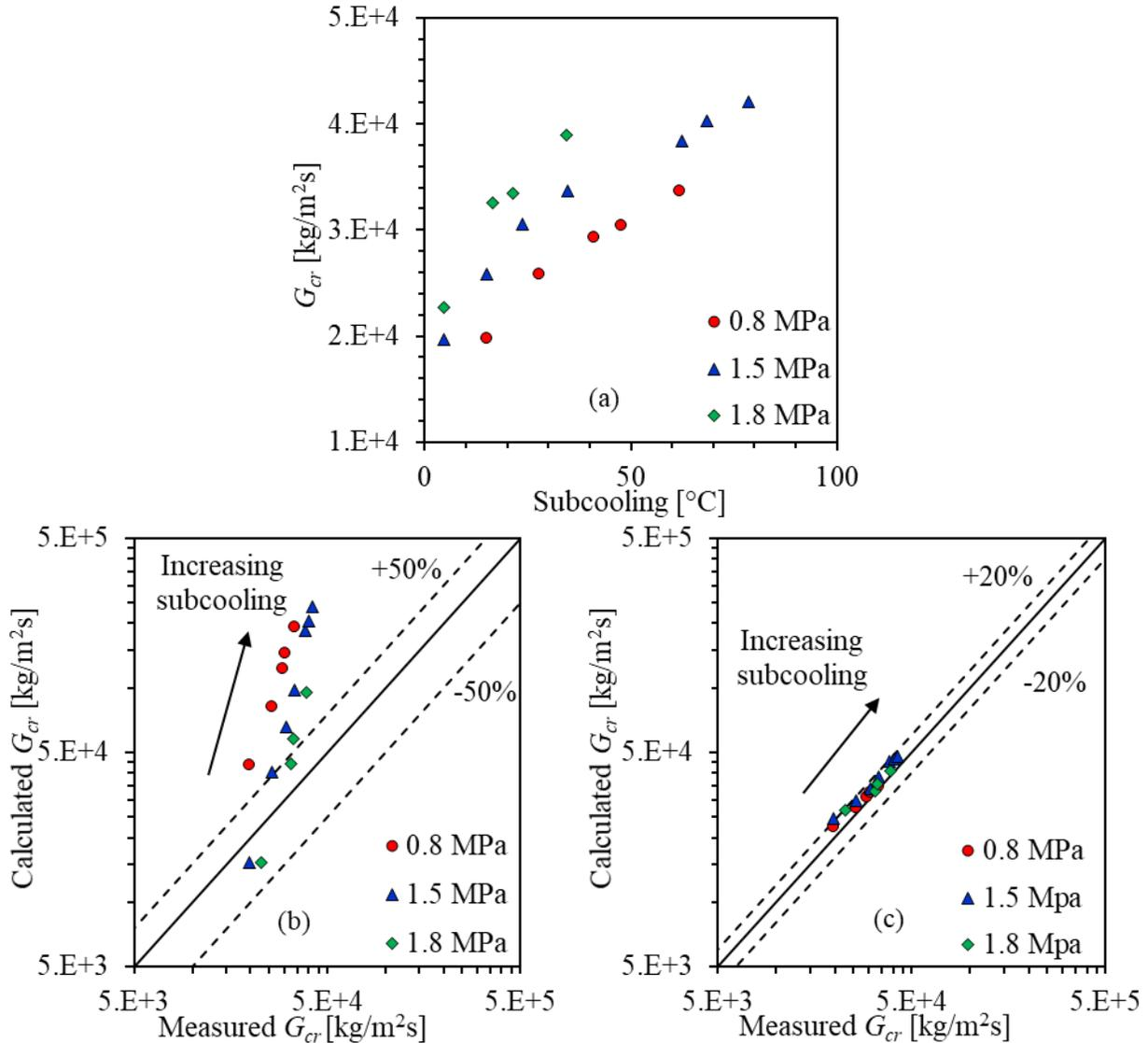
Figure 3-59 Critical Mass Flux for Subcooled Water Jets: (a) Experimental Data in Celata et al. (1986) for  $L_p/D = 10$  in 4.6 mm Pipe, (b) Comparison between Experimental Data and HEM, and (c) Comparison between Experimental Data and Henry and Fauske Model (1971)
