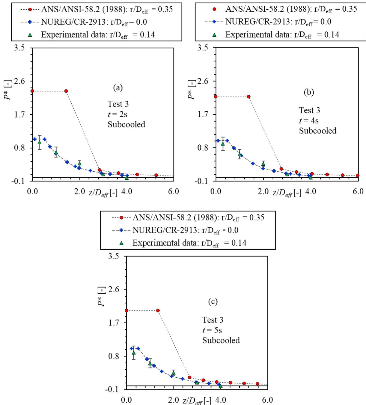
Figure 3-54 Comparison between ANS/ANSI-58.2 (1988), NUREG/CR-2913 and Experimental Data in Marviken Tests of Test 3 for Stagnation Pressure: (a) 2 s, (b) 4 s and (c) 5 s. Error Bar:  $\pm 20\%$ . Comparisons between NUREG/CR-2913 and Experimental Data are Obtained from NUREG/CR-2913
