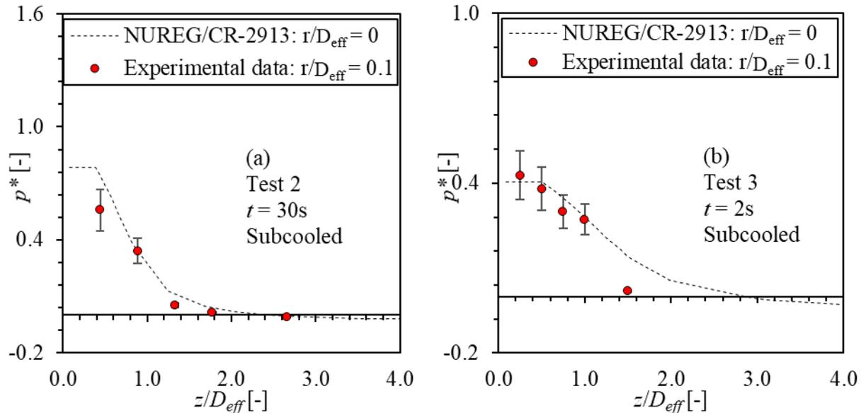
Figure 3-53 Comparison between NUREG/CR-2913 and Experimental Data in Marviken Tests for Static Pressure: (a) Test 2: 30 s, (b) Test 3: 2 s. Error Bar:  $\pm 20\%$ . Comparisons are Obtained from NUREG/CR-2913
