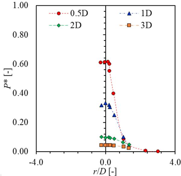
Figure 3-20 Impinging Saturated Water Jets in Kastner and Rippel (1987): Stagnation Pressure at the Target Plate Downstream of the Break Plane ( $P_o = 10$  MPa,  $D = 65$  mm)
