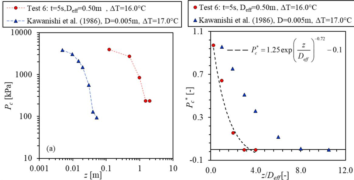
Figure 3-27 Stagnation Pressure Profiles at the Center of Free Subcooled Water Jets ( $\Delta T \sim 16^\circ\text{C}$ ) as a Function of Axial Distance. The Best Fitting Line in Figure (b) is Given by Equation (3-11)
