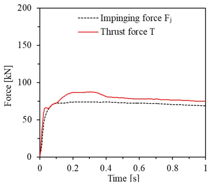
Figure 2-25 Comparison between Thrust Force and Impinging Force for BWR LOCA ( $D = 150$  mm) Conditions (Yano et al., 1984)
