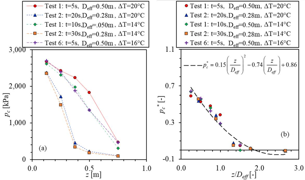
Figure 3-25 Static Pressure Profiles at the Center of Free Subcooled Water Jets ( $\Delta T = 14^\circ C \sim 20^\circ C$ ) as a Function of Axial Distance. The Best Fitting Line in Figure (b) is Given by Equation (3-9)
