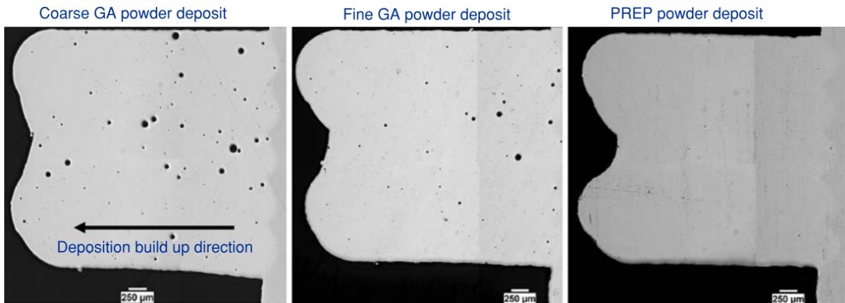
Figure 6. Examples of powder atomization-induced porosity in components [26]. GA = gas-atomized; PREP = plasma rotating electrode process
