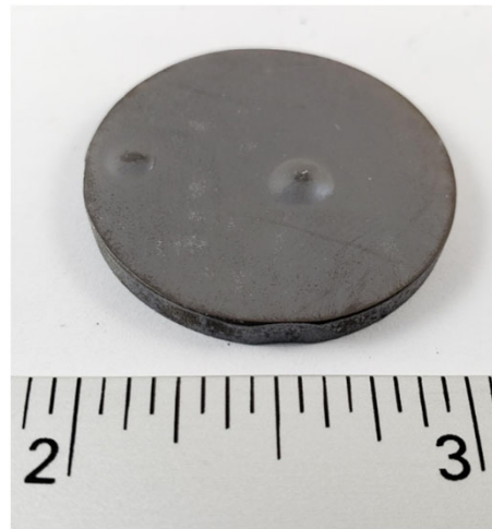
Blistered pure Ni coating after thermal cycling
