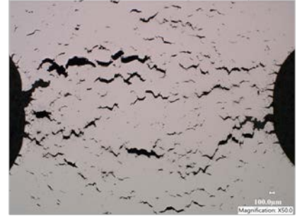
Creep cavitation (INL)
