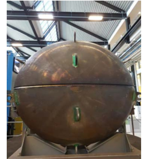
Mockup EB weld of lower head
