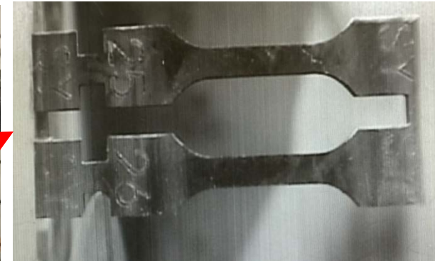
Intact irradiated quad held with hot cell grips prior to separation into 4 individual miniature tensile specimens
