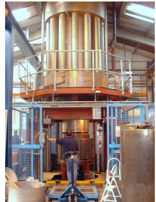
40" diameter HIP Vessel Courtesy: Isostatic Forge International
