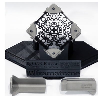
Framatome/TVA/ORNL TCR – AM Channel Fasteners Source: ORNL Press Release October 19, 2020
