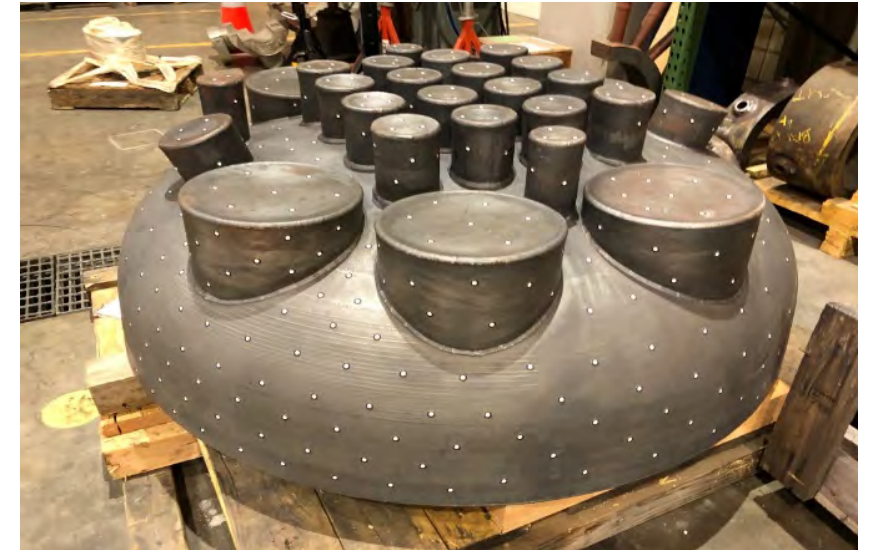
Powder Metallurgy-HIP: 100-10,000 lbs (45-4500 kg)
