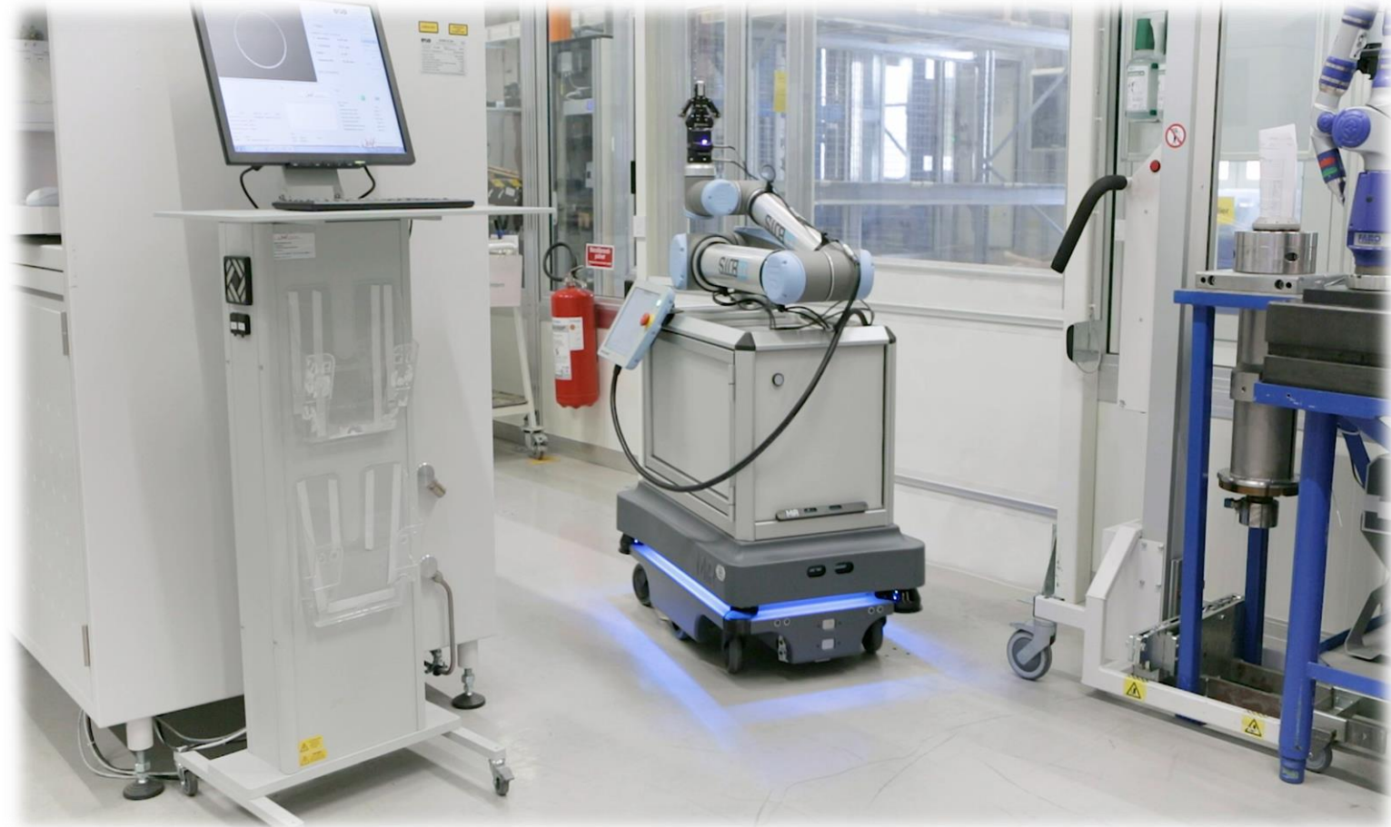
Collaborative robots for cleaning of machines chamber
