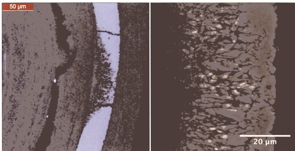
Figure 7-9 Optical (left) and electron (right) micrographs of a region of the SiC layer corroded by CO in an irradiated UO 2 particle heated to 1600°C
