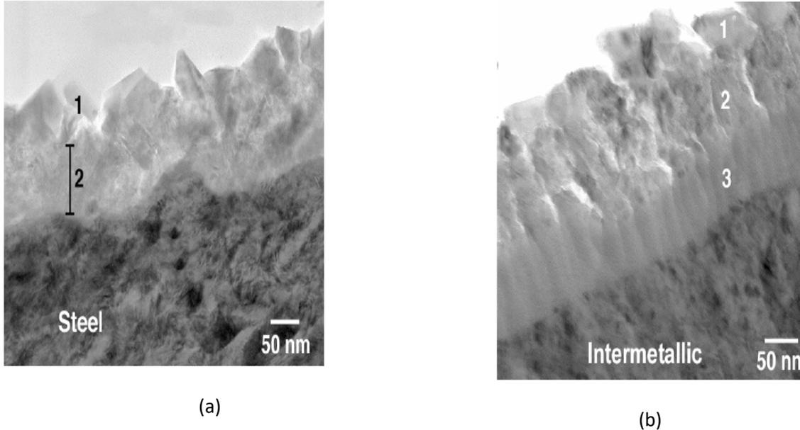
**Figure 3-6. Transmission electron microscope photomicrographs of (a) two labeled oxide layers with different morphologies over stainless steel phase and (b) three labeled oxide layers with different morphologies over intermetallic phase of metallic HLW form reacted at 200 °C [392 °F] for 91 days in water vapor (Ebert, 2005)**
