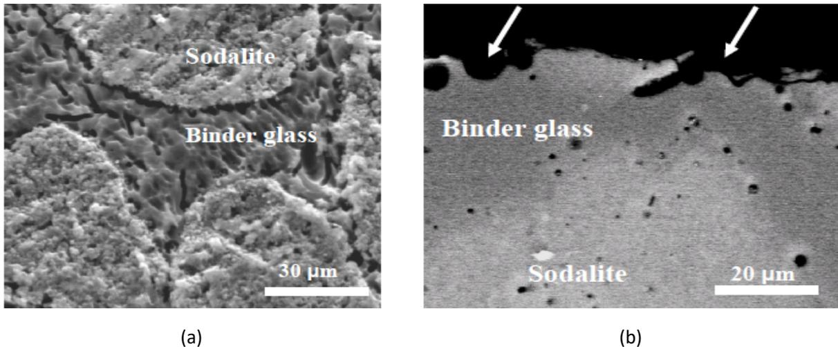
Figure 3-3. Photomicrographs showing (a) surface and (b) cross-section of ceramic HLW form reacted with humid air for 105 days at 150 °C [302°F] (Ebert, 2005)
