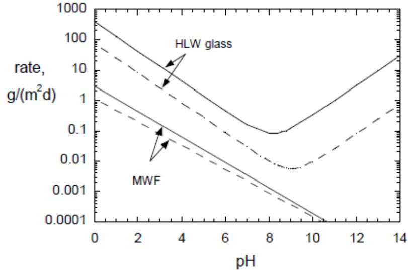
**Figure 3-7. Dissolution rates for metallic HLW form and high-level waste glass (Ebert, 2005)**
