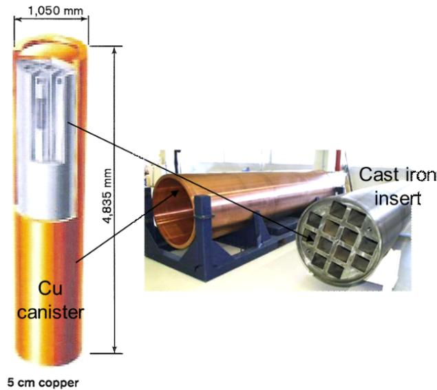
Figure 2-2. Waste container proposed by the Swedish Nuclear Fuel and Waste Management Co. (SKB, 2011)
