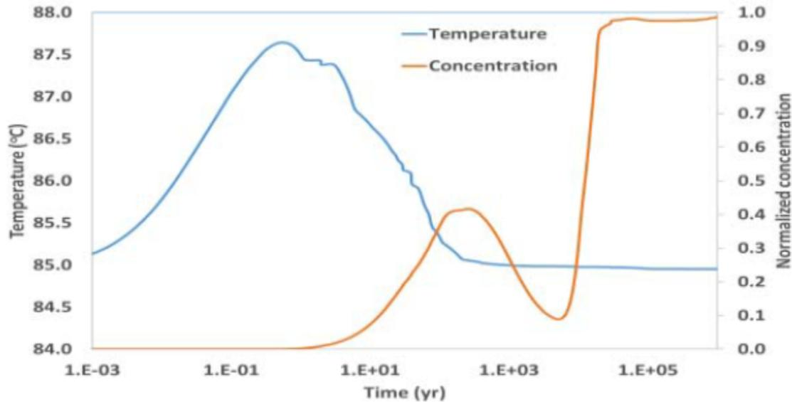
**Figure 2-4. Computed thermal and salt concentration as a function of time for salt water at 3,000-m [1.9 mi] depth in a disposal borehole (Rechar et al., 2017a)**
