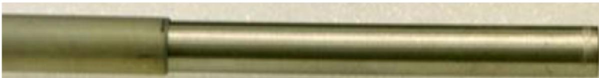
**Figure 2-7. Fermi-1 blanket fuel rod after removing sodium by melt-drain-evaporate-carbonate process (INL, 2007)**
