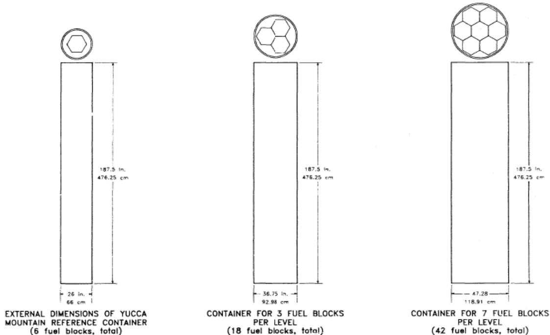
**Figure 2-3. Example waste package design for spent coated particle fuel (Lotts et al., 1992)**
