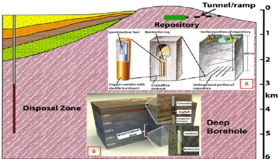
Figure 2-1. Concepts of a mined geologic repository and deep borehole for high-level waste disposal (NWTRB, 2017)
