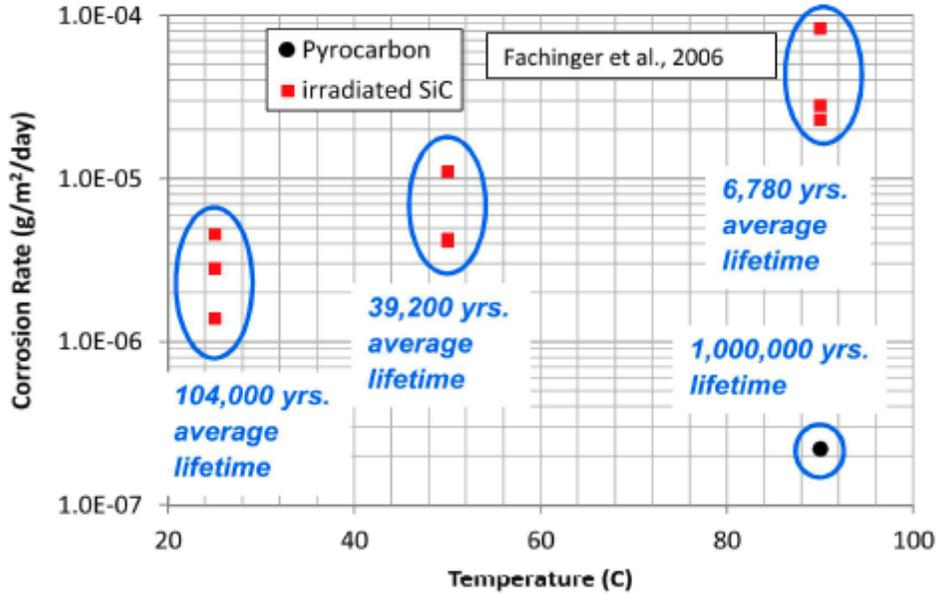
Figure 3-1. Estimated SiC layer lifetimes by corrosion of SiC at various temperatures for different brines (Gelbard and Sassani, 2018)
