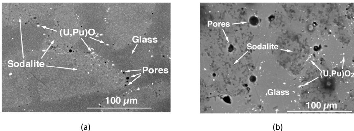
**Figure 2-5. Photomicrographs showing microstructures of U, Pu-doped ceramic HLW forms produced from (a) hot isostatic press and (b) pressure-less consolidation (Ebert, 2005)**
