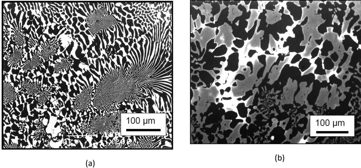
**Figure 2-6. (a) Microstructure of a metallic waste form with 15 mass percent Zr containing about 50 volume percent stainless steel (dark regions) and 50 volume percent intermetallic phase (light regions) (b) regions in intermetallic phase enriched in uranium (brighter regions) (Ebert, 2005)**
