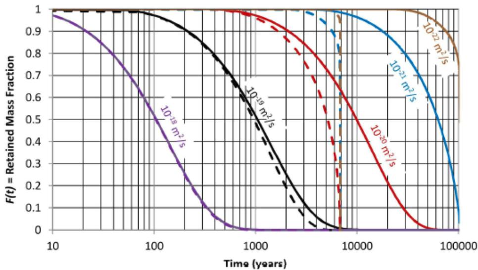
Figure 3-2. Fraction of fission product mass remaining within the TRISO fuel as a function of the diffusivity and corrosion rate of the SiC layer. Solid lines and dashed lines correspond to corrosion lifetimes of 100,000 years and 7,000 years, respectively. (Gelbard and Sassani, 2018)
