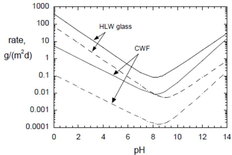
Figure 3-5. Dissolution rates for ceramic HLW form compared to HLW glass (Ebert, 2005)
