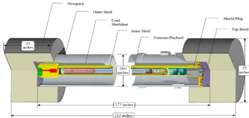
**Figure 2-2. T-3 cask used to transport sodium-bonded spent FFTF metal fuel from Hanford to INL (Ross et al., 2014)**
