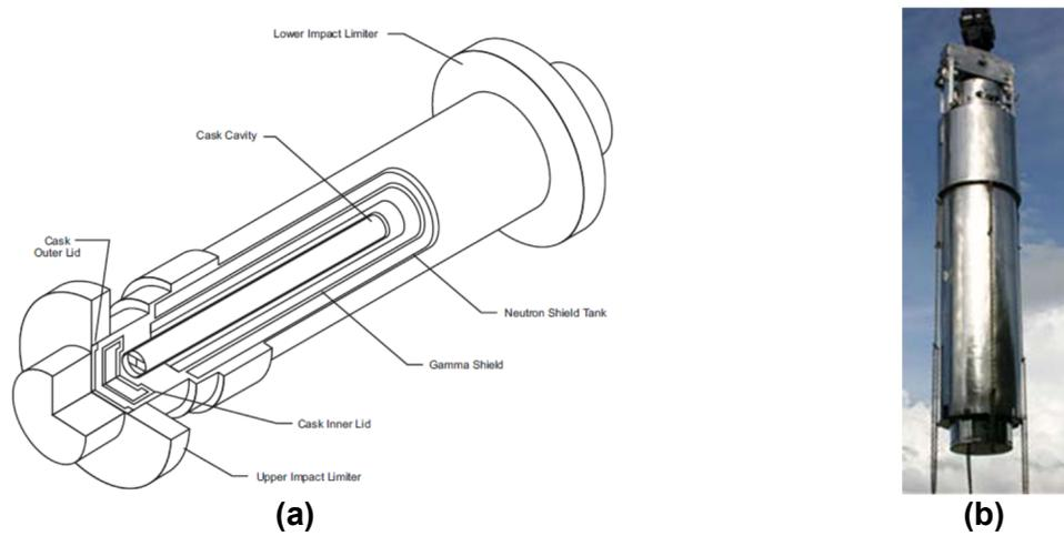
**Figure 2-3. (a) Simplified drawing and (b) a photo of a NAC-LWT (legal weight truck) shipping cask (DOE, 2000)**
