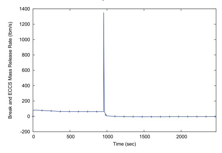
Figure 6.2-14: Break and Emergency Core Cooling System Energy Release Rate - Peak Containment Vessel Temperature Case
