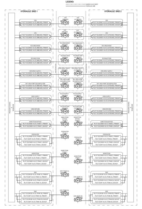
Figure 6.2-8: Containment Isolation Valve Hydraulic Skid Schematic
