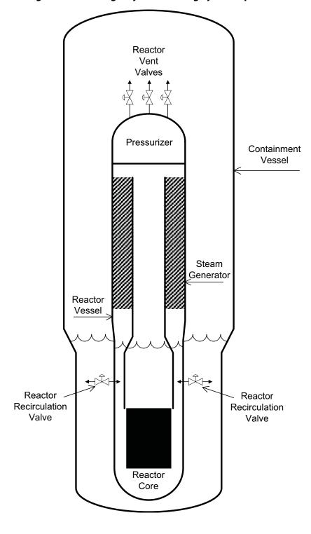
Figure 6.3-2: Emergency Core Cooling System Operation
