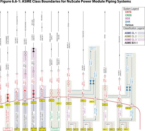
Figure 6.6-1: ASME Class Boundaries for NuScale Power Module Piping Systems
