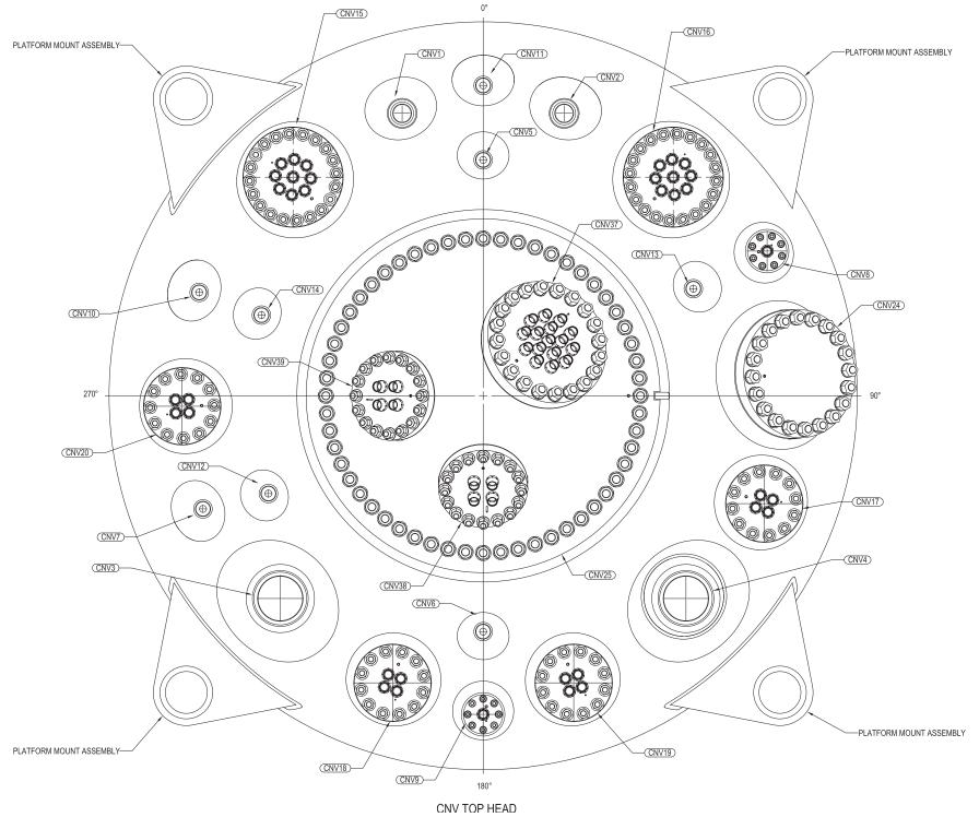
Figure 6.2-3b: Containment Vessel Penetrations
