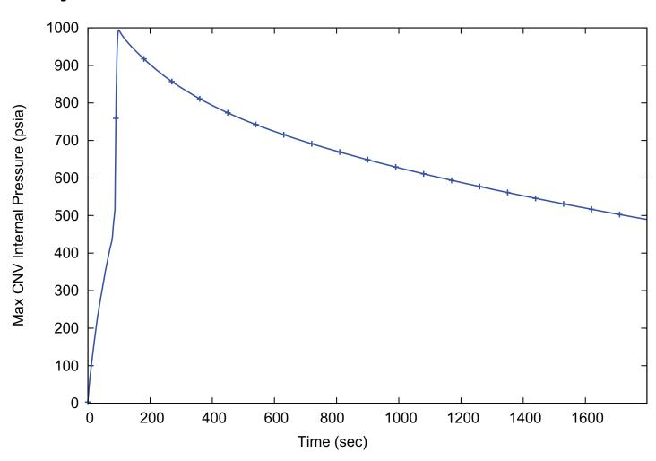
Figure 6.2-10: Break and Emergency Core Cooling System Mass Release Rate - Peak Containment Vessel Pressure Case
