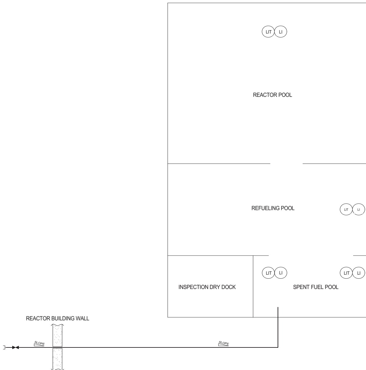
Figure 9.2.5-2: Ultimate Heat Sink Qualified Makeup Line and Instrumentation Diagram
