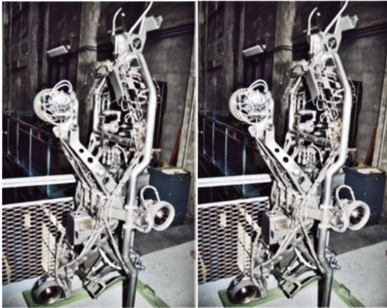
**Figure 8 MIR inspection device (from [9, Figure 19.2])**
