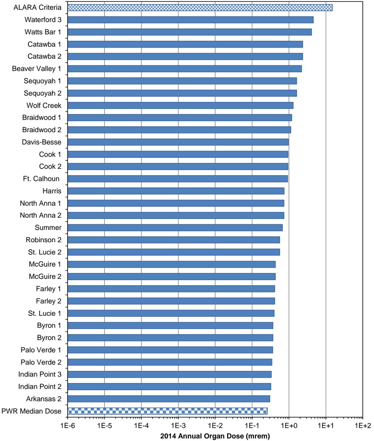
**Figure 3.18 PWR Gaseous Effluents — Maximum Annual Organ Dose**
