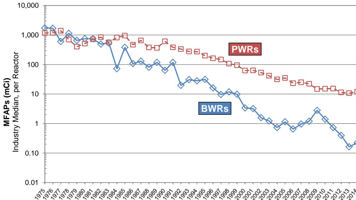
**Figure 3.16 Long-Term Trend in MFAPs in Liquid Effluents**
