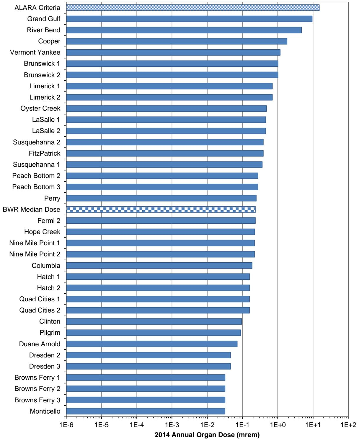
**Figure 3.17 BWR Gaseous Effluents — Maximum Annual Organ Dose**
