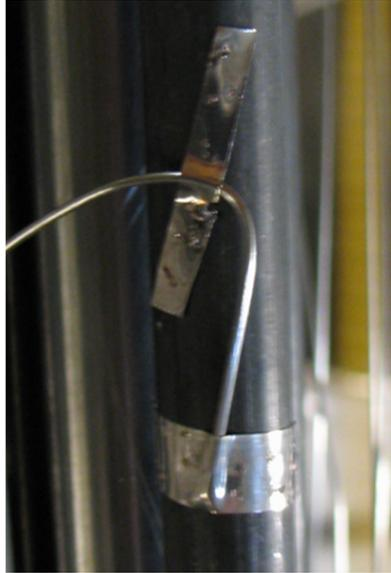
**Figure 2-5 Typical TC Attachment to Heater Rod**
