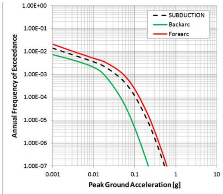
**Figure 3-13** Example of seismic hazard feedback showing the effect of alternative branches of a GMC logic tree. Shown are the hazard curves resulting from use of either a backarc or a forearc GMPE. The dashed line is the weighted combination of both branches of the logic tree.
