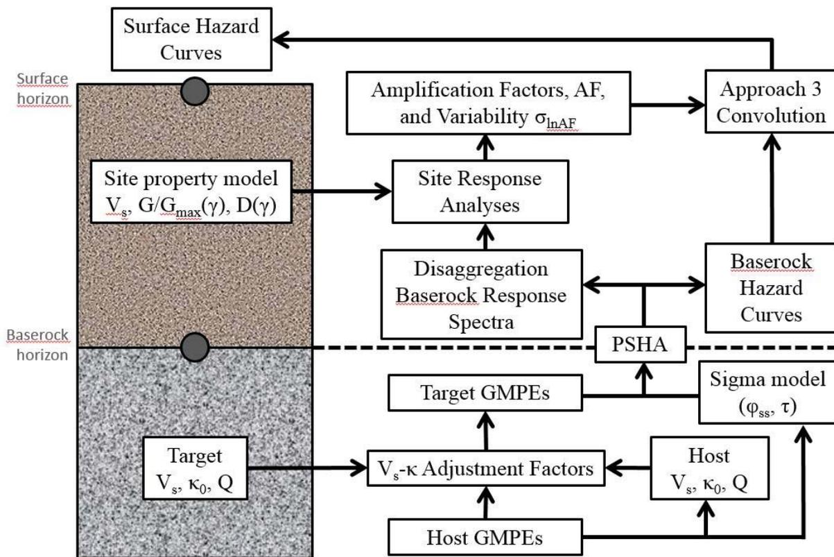
**Figure 3-7 Schematic illustration of the incorporation of site response into PSHA following the Bazzurro and Cornell (2004a,b) approach, which is also referred to as Approach 3 in NUREG/CR-6728. Figure from Rodriguez-Marek et al. (2014). AFs refer to amplification functions.**
