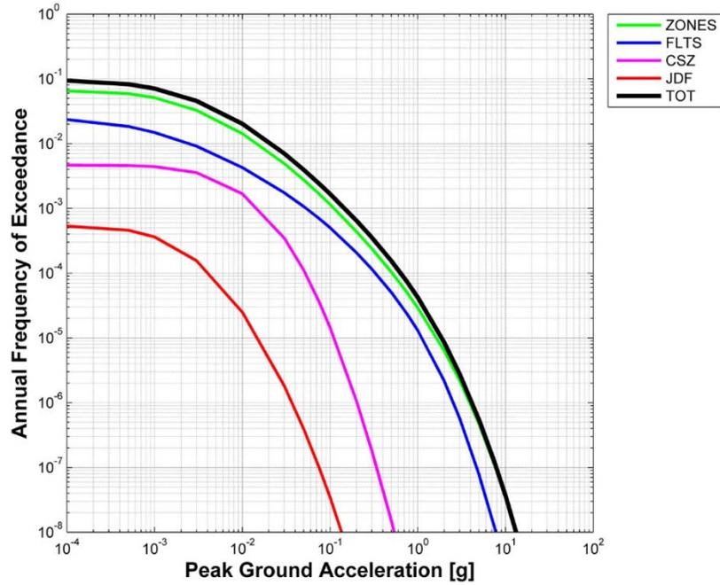
**Figure 3-10** Example of seismic hazard feedback showing the relative contributions of various types of seismic sources to the peak ground acceleration hazard at a site of interest. The total hazard is shown by the black hazard curve.
