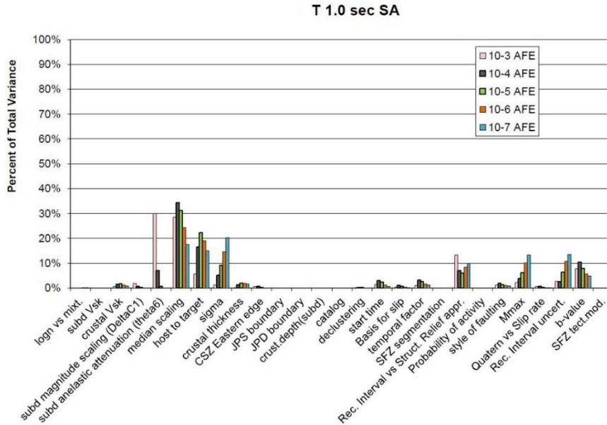
**Figure 3-14** Example of seismic hazard feedback showing the percent contribution that various elements of the GMC and SSC logic trees make to the total variance in the hazard distribution. Variance contribution histogram at the  $10^{-3}$ ,  $10^{-4}$ ,  $10^{-5}$ ,  $10^{-6}$ , and  $10^{-7}$  annual frequencies of exceedance for the T 1.0-sec spectral acceleration. These types of plots provide insight into the largest contributors to the uncertainties in the seismic hazard.
