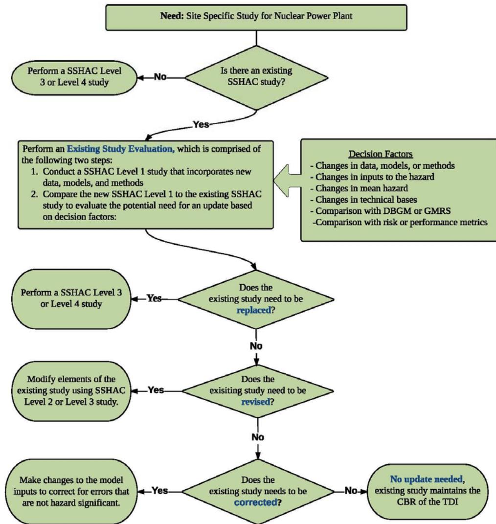
Figure 4-1 Flowchart illustrating the steps to evaluate the need for updating an existing site-specific PSHA.
