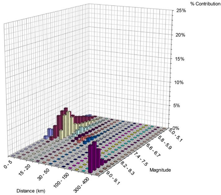
**Figure 3-12** Example of seismic hazard feedback showing a deaggregation plot for the magnitude and distance contributions to the hazard at 1.0 second spectral accelerations at an annual frequency of exceedance of  $10^{-4}$ . Such plots can be compared to the magnitude and distance contributions at other structural periods and other annual frequencies of exceedance.
