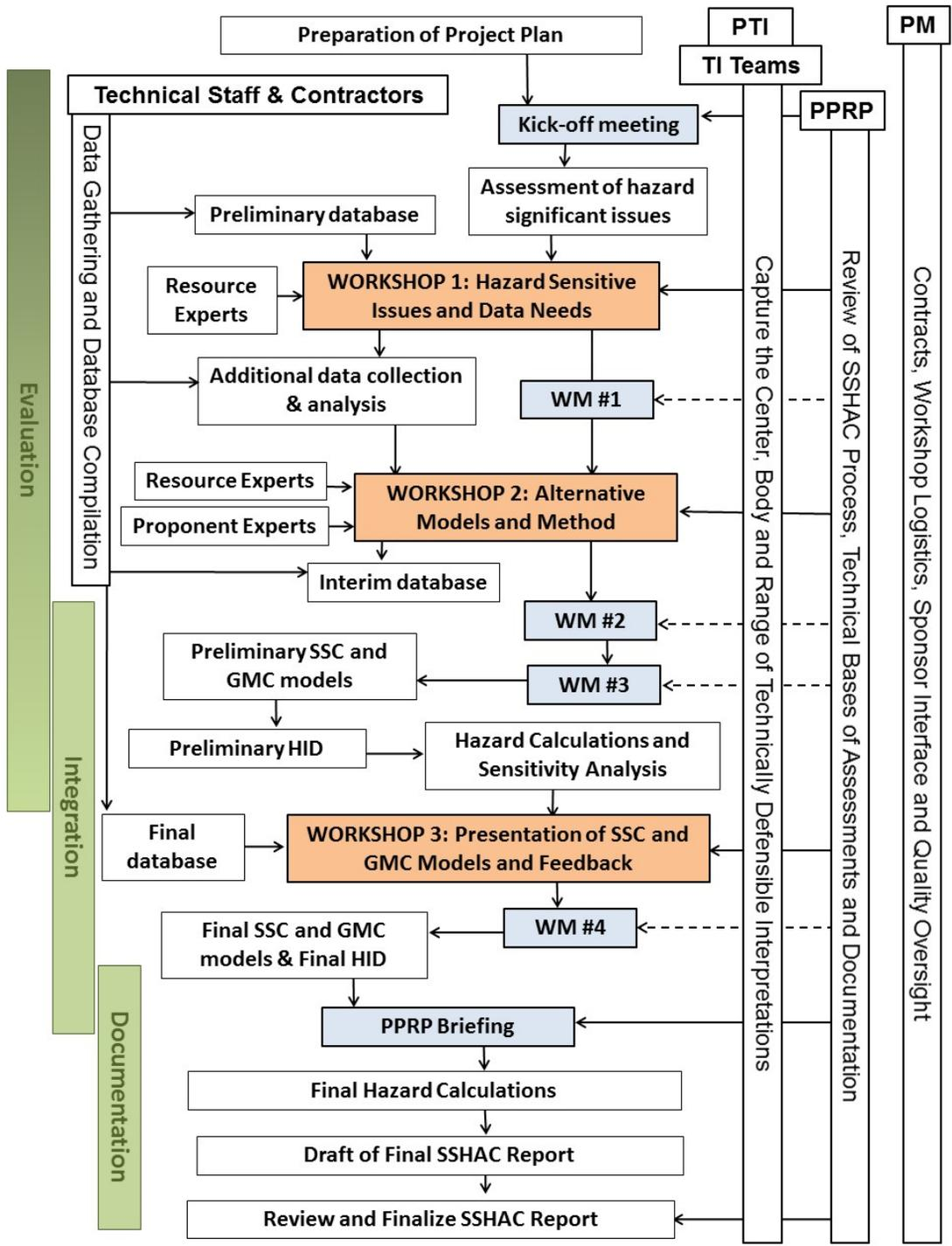
**Figure 3-4** Flowchart illustrating the key features in a SSHAC Level 3 process. The order of activities runs from top to bottom of the diagram. The timing of the working meetings reflects one suggested arrangement and alternative schemes may be used, although one meeting after Workshop #3 is essential. Dashed arrows indicate activities where one (or more) PPRP member(s) is selected to observe and represent the larger panel.
