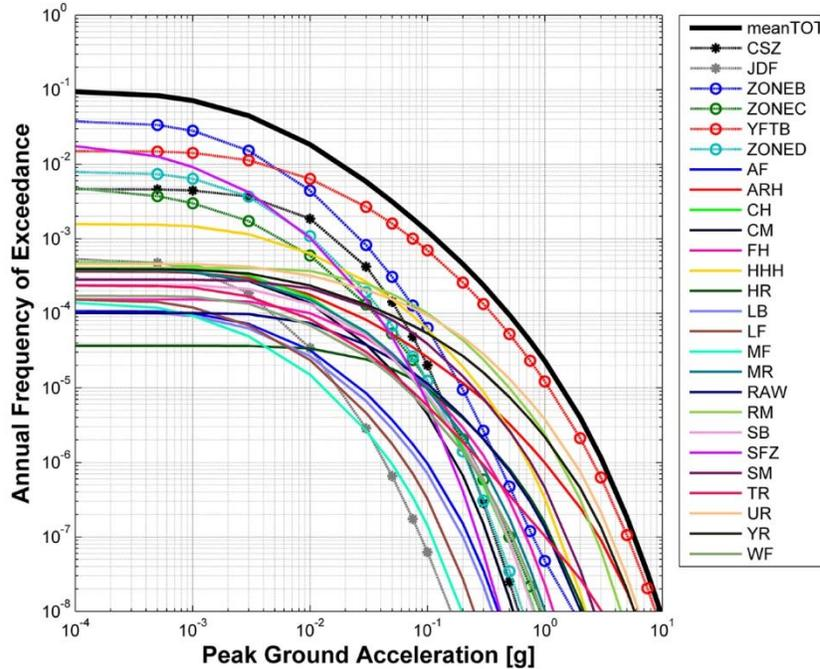
**Figure 3-11** Example of seismic hazard feedback showing the relative contributions to the peak ground acceleration hazard of all seismic sources in an SSC model. Such plots can provide an indication of the dominant contributors to the hazard at annual frequencies of exceedance of interest.
