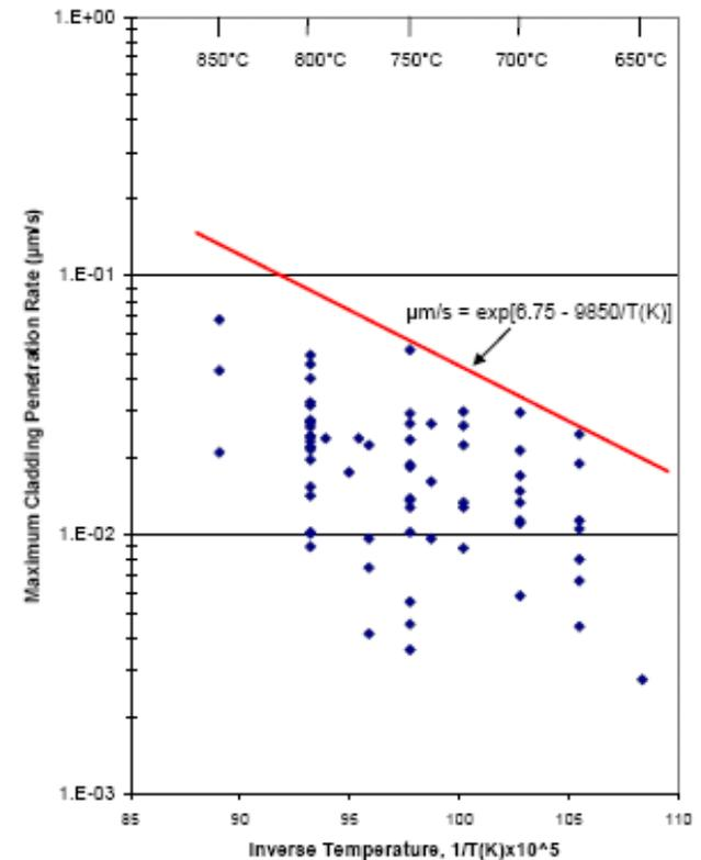
**Effective cladding penetration rates from FBTA tests for specimens tested for 1.0 hour (Tsai, et al., 2007)**
