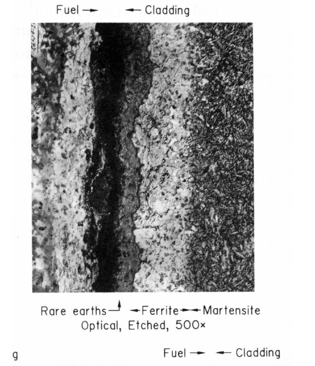
FCCI of U-10Zr/HT-9 due to interdiffusion of fuel/cladding constituents after 6 at% burnup at 620°C (Hofman & Walter 1994)
