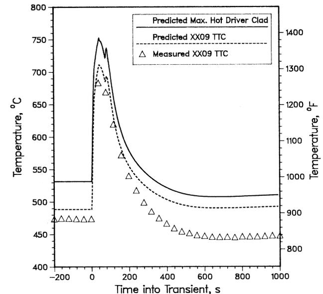
Unprotected loss-of-flow test in EBR-II demonstrated the benign behavior predicted (Mohr, et al., 1987)
