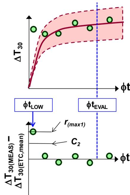
Figure 5-3 Specific procedures to account for failure of the mean test (left) or low-fluence outlier statistical test (right)
