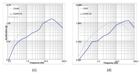
Figure 2.5-2 NuScale horizontal (c) and vertical (d) certified seismic design response spectra— high frequency 5-percent damping (after DCA PART 2 Figures 5.0-3 and 5.0-4)
