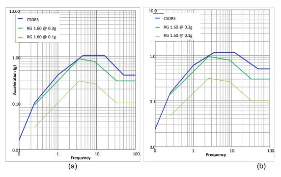
Figure 2.5-1 NuScale horizontal (a) and vertical (b) certified seismic design response spectra 5-percent damping (after DCA PART 2 Figures 5.0-1 and 5.0-2)
