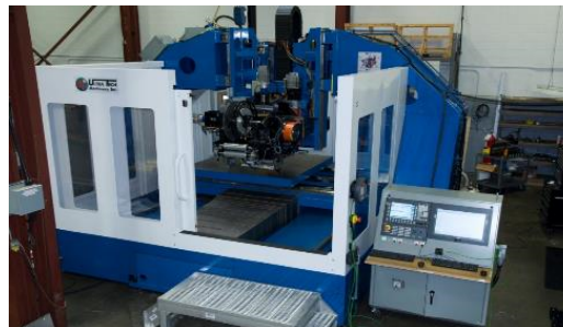
Sheet Lamination UAM Fabrisonic
