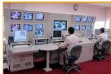
Automatic control system and computer measurement system for short-circuit test
