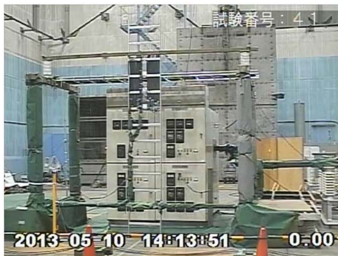
[Test 4-1: Lower VCB Terminal, Arc duration 2.39s, Arc Energy 44.6MJ]
