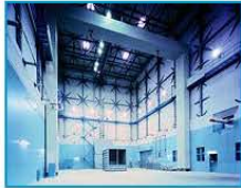
Indoor test cell with soundproofing 40m X 25 m X 29 m (H)
