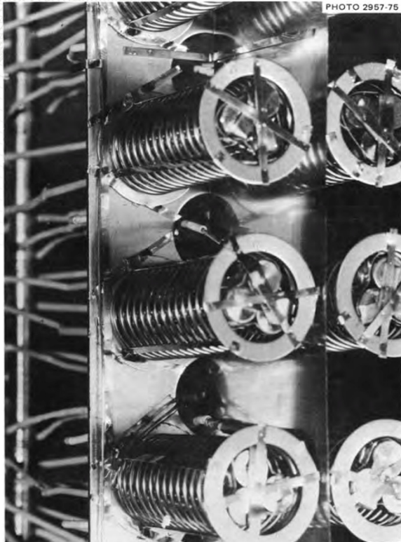
Cluster of modified Alloy N creep specimens prior to irradiation
