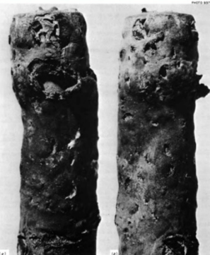
Tip of a SS304 probe inadvertently used in an Inconel 600 salt loop for 192 hours
