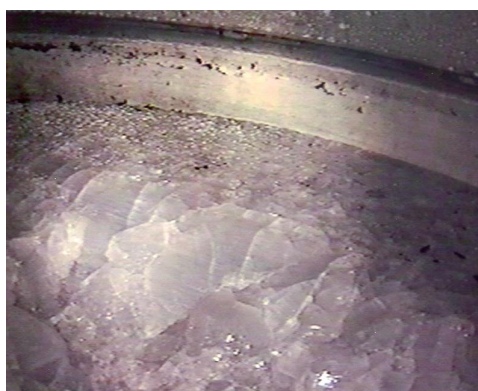
(left) Solid “Frozen” and (right) Liquid “Molten” 2LiF-BeF 2 salt
