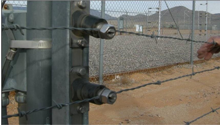
**Figure 28 Taut wire push test**
