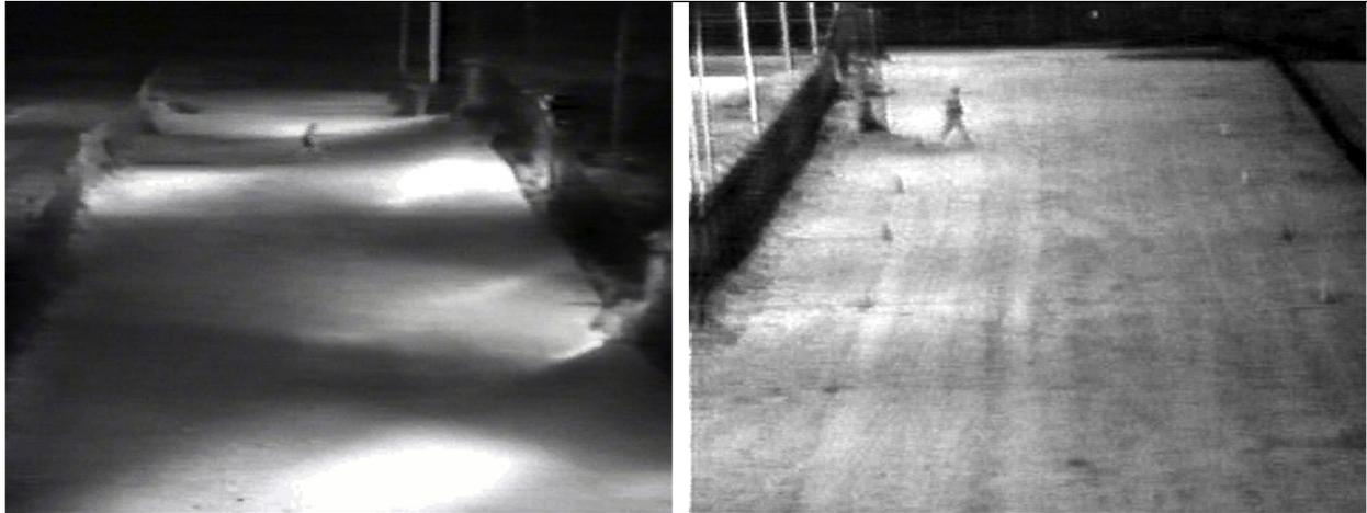
**Figure 73 Examples of light-to-dark ratios for camera assessment**
