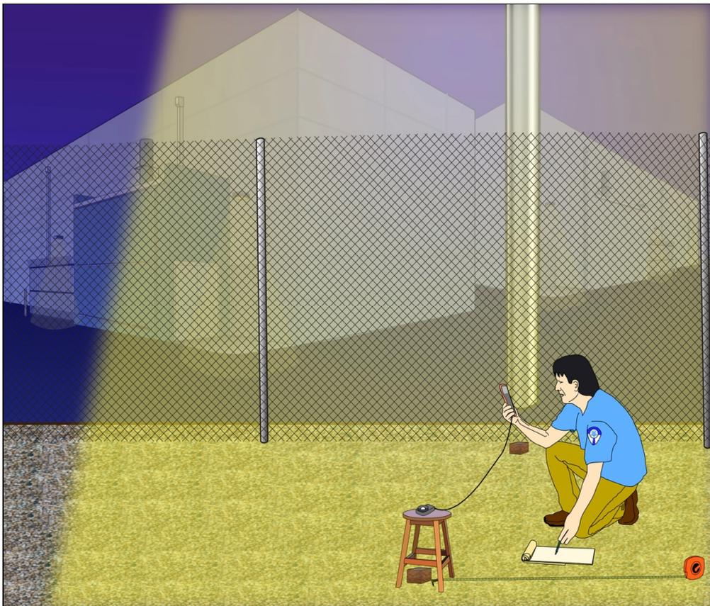
**Figure 76 Checking light levels with a light meter within a perimeter isolation zone**
