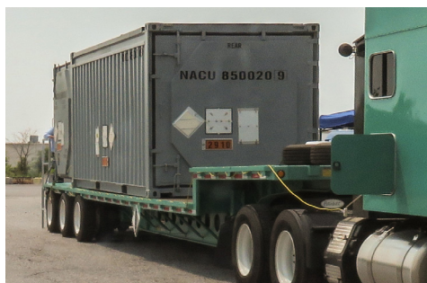
Truck carries NAC LWT transport package.
