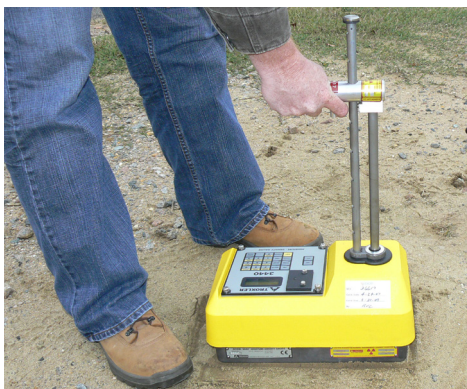
A moisture density gauge indicates whether a foundation is suitable for supporting a building or roadway.
