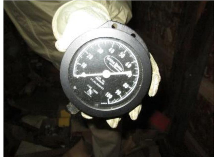
**A-10. Gauge Found with up to 30,000 cpm and 16  $\mu$ R/h on contact**
