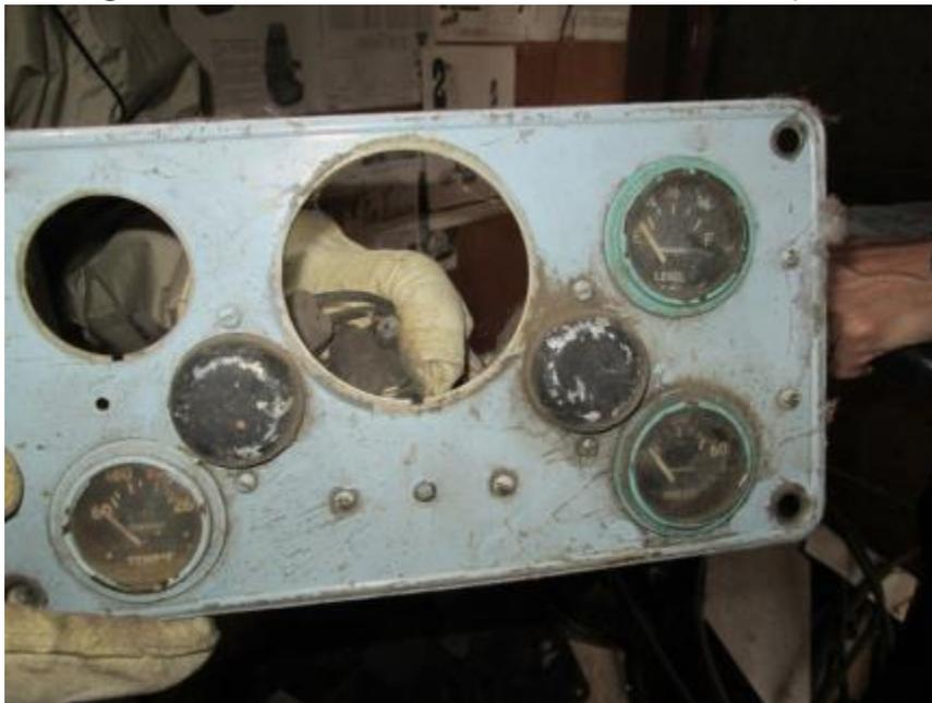
**A-11. Gauges Found with Measurable Exposure Rates up to 100  $\mu$ R/h on contact**
