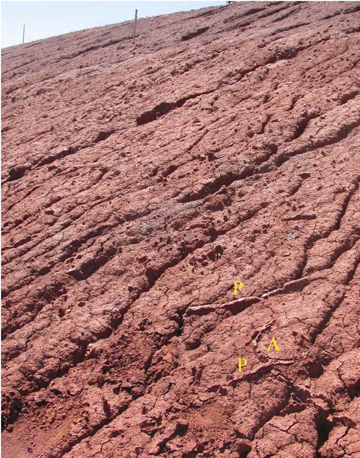
Figure 1. Antitaxial gypsum veins found in the WCS RCRA landfill are discontinuous and display planar (P) and arcuate (A) morphologies.
