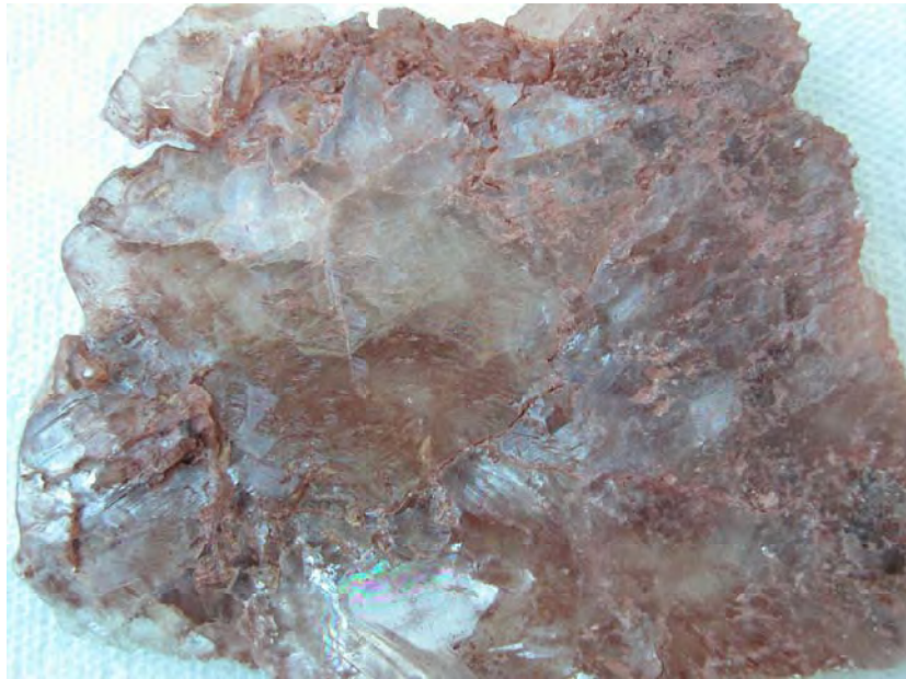
Figure 5. This gypsum fracture filling from the WCS site displays large interlocking crystals with lenticular surfaces. Note that some wall rock mudstone has been incorporated within the crystals, especially along crystal boundaries.
