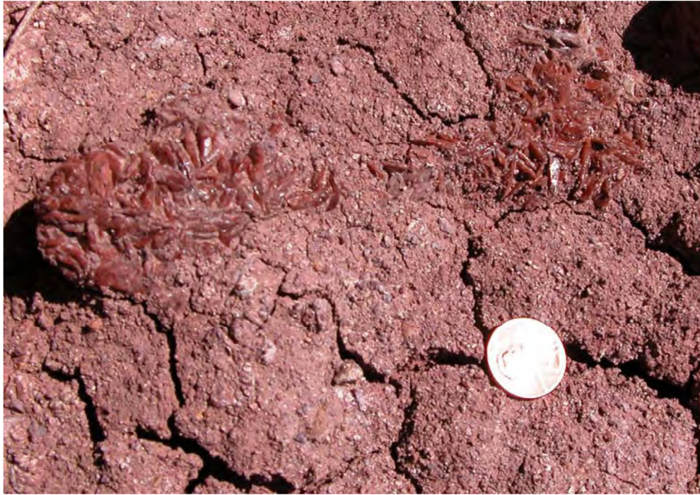
Figure 4. Some lenticular gypsum rosettes occur in irregular masses within the host mudstone.
