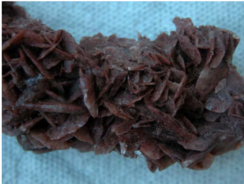
Figure 3. Rosettes of gypsum crystals display lenticular crystal habits. This example occurs in a roughly cylindrical zone and could be a rizolith.
