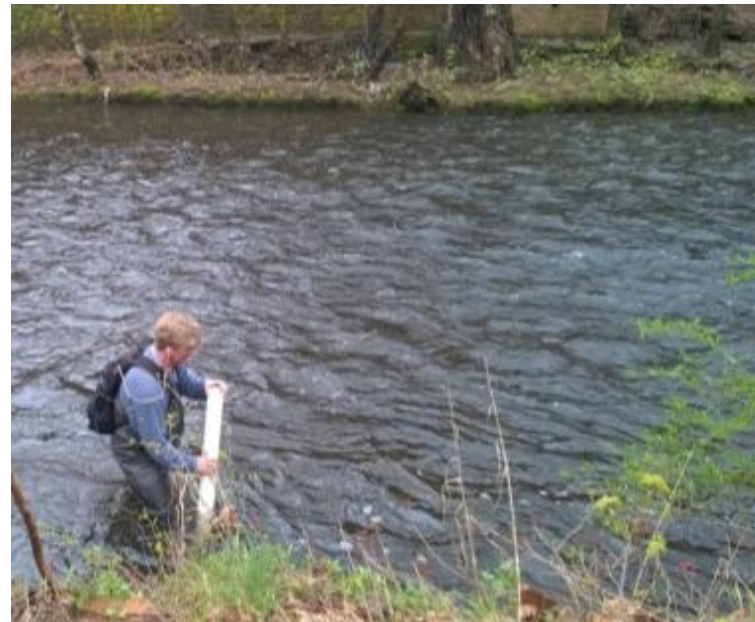
A-22. River Survey using 2×2 NaI in PVC Tube
