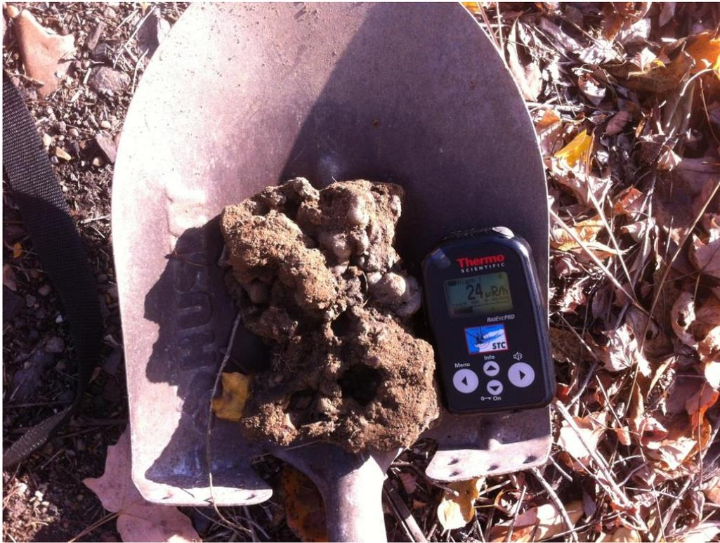
**Figure A.1. Slag-like material removed from location A**
