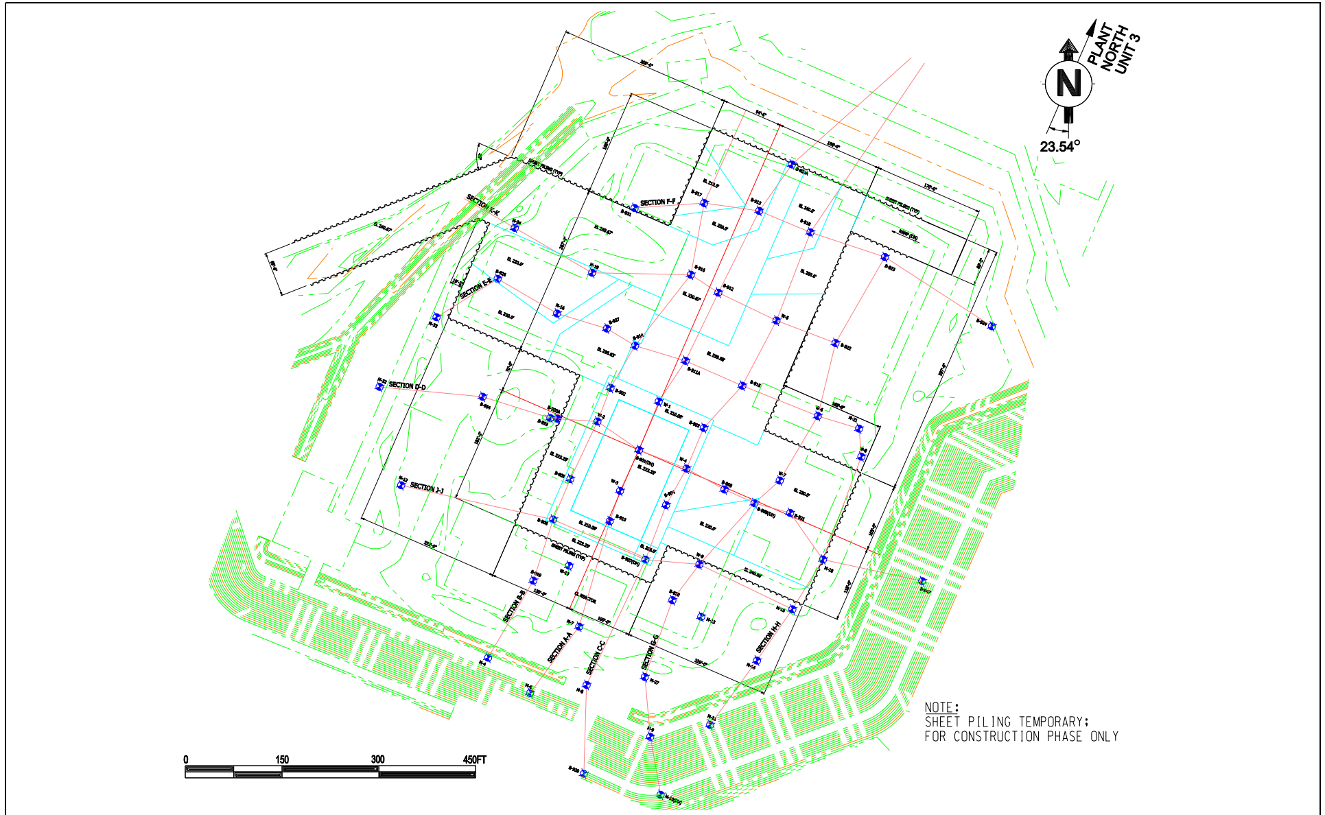
NAPS COL 2.0-29-A Figure 2.5.4-206 Excavation Plan and Locations of Profiles
