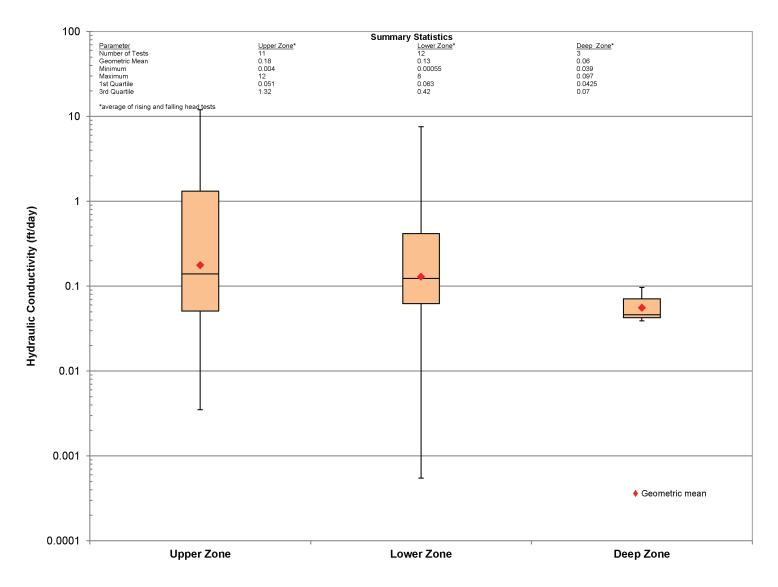
a) Box and whisker plot of slug test hydraulic conductivity by observation well monitoring zone. Data from Table 2.3.1-6
