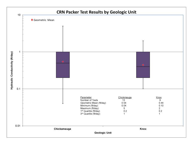
a) Box and whisker plot of CRN packer test results by geologic unit. Data from Table 2.3.1-5 and Appendix 2.3-B
