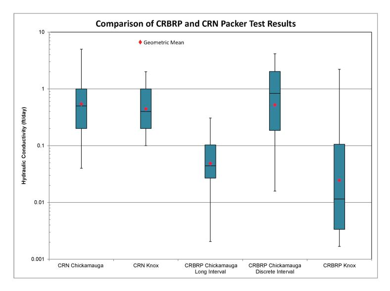
b) Box and whisker plot comparing CRN packer test results with CRBRP packer test results. Data from Table 2.3.1-5 and Appendix 2.3-B
