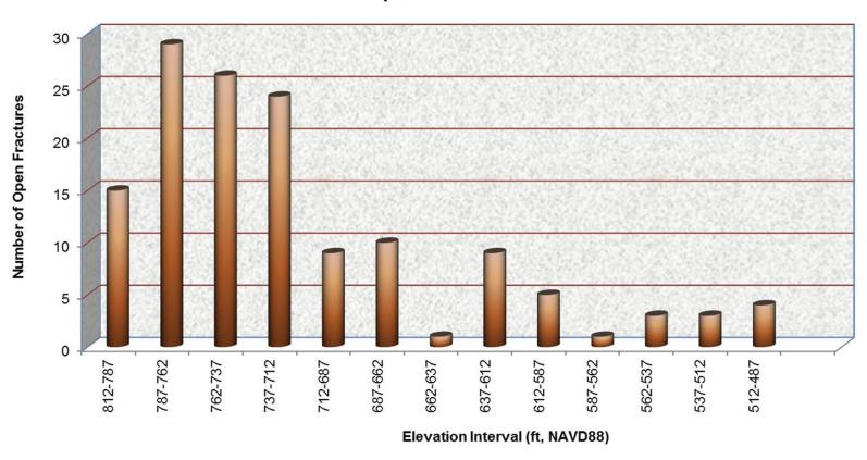
Figure 2.3.1-44. Fracture Frequency Histogram
