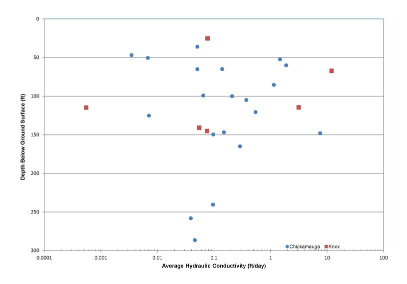
b) Scatter plot of slug test hydraulic conductivity with depth below ground surface. Data from Table 2.3.1-6
