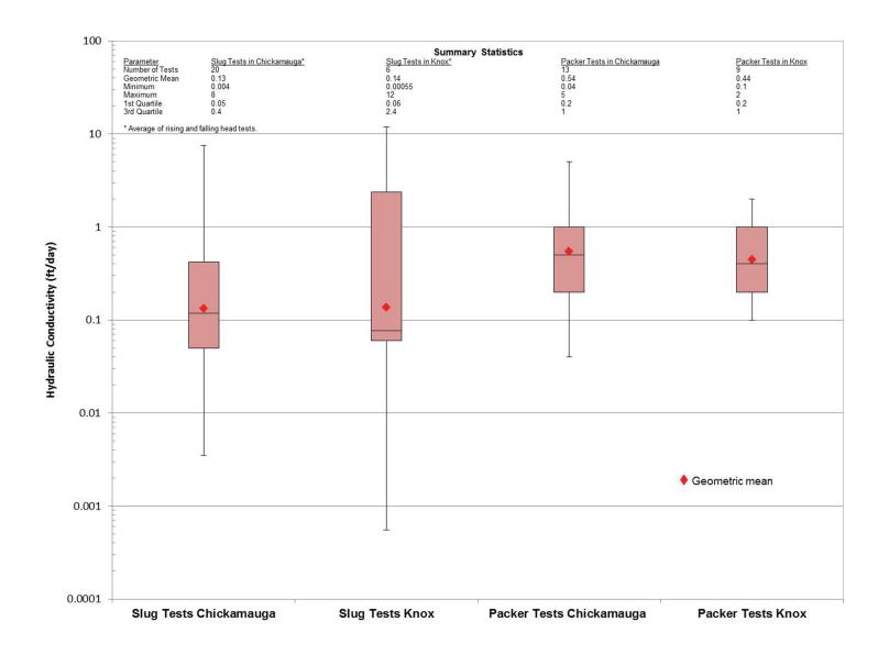
Figure 2.3.1-49. Comparison of Slug and Packer Test Results
